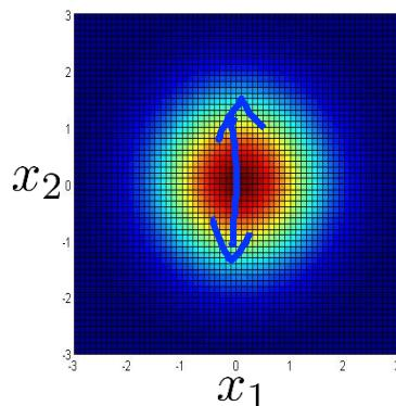
$$\mu = \begin{bmatrix} 0 \\ 0 \end{bmatrix} \Sigma = \begin{bmatrix} 1 & 0 \\ 0 & 0.6 \end{bmatrix}$$
