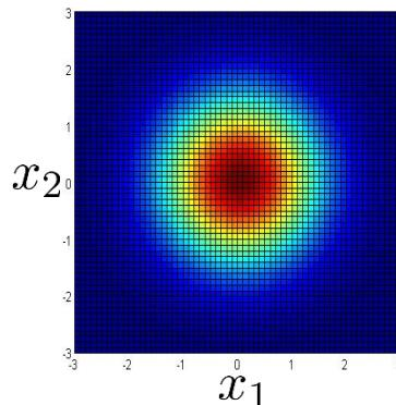
$$\mu = \begin{bmatrix} 0 \\ 0 \end{bmatrix} \Sigma = \begin{bmatrix} 0.6 & 0 \\ 0 & 1 \end{bmatrix}$$
