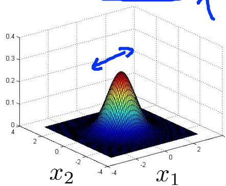
$$\mu = \begin{bmatrix} 0 \\ 0 \end{bmatrix} \Sigma = \begin{bmatrix} 2 & 0 \\ 0 & 2 \end{bmatrix}$$
