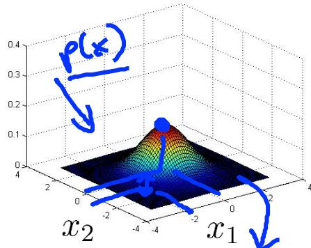
$$\mu = \begin{bmatrix} 0 \\ 0 \end{bmatrix} \Sigma = \begin{bmatrix} 0.6 & 0 \\ 0 & 0.6 \end{bmatrix}$$
