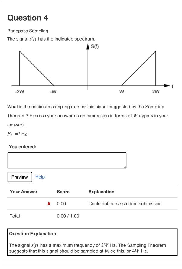
Because of the particular structure of this bandpass spectrum, you might wonder whether a lower sampling rate could be used. This is indeed the case, first find the lower sampling rate that can be used to reconstruct s(t) from its samples. Express your answer in terms of W.
