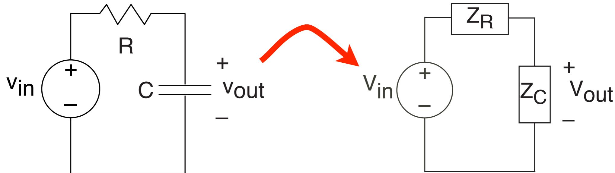
$$V_{\text{out}} e^{j2\pi ft} = \frac{1}{j2\pi fRC + 1} V_{\text{in}} e^{j2\pi ft}$$
