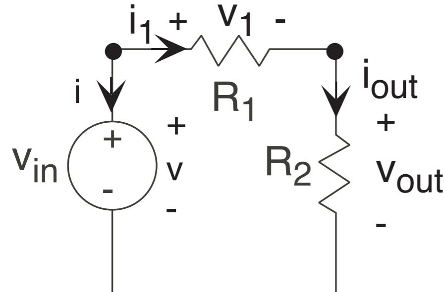
$$v_{\text{out}}(t) = \frac{R_2}{R_1 + R_2} v_{\text{in}}(t)$$
