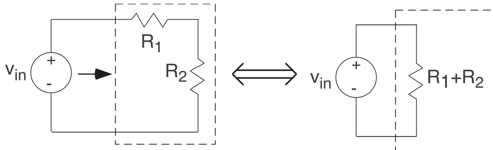
Resistors in series appear to be a *single* resistor, the value of which is the sum of the component values
