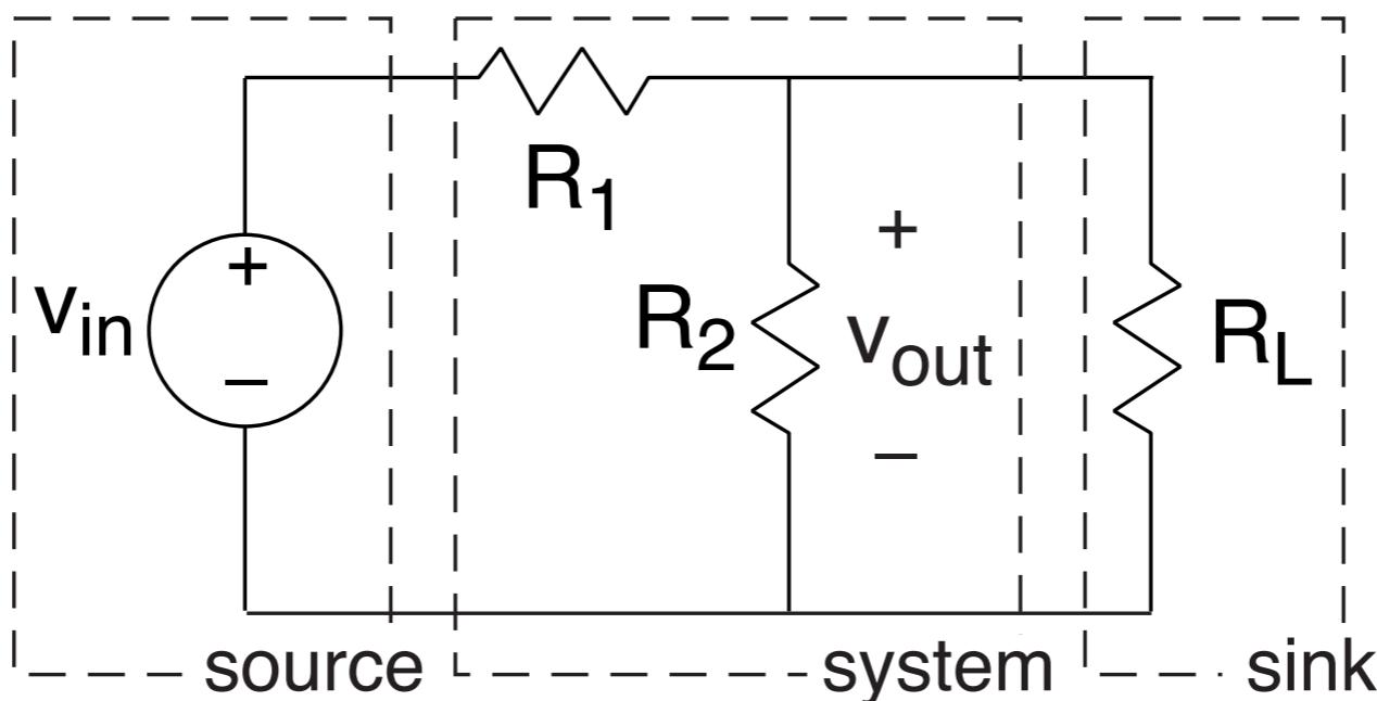
$$\begin{aligned}v_{out} &= \frac{R_2 \| R_L}{R_1 + R_2 \| R_L} v_{in} \\&= \frac{\frac{R_2 R_L}{R_2 + R_L}}{R_1 + \frac{R_2 R_L}{R_2 + R_L}} v_{in} \\&= \frac{R_2 R_L}{R_1 R_2 + R_1 R_L + R_2 R_L} v_{in}\end{aligned}$$
