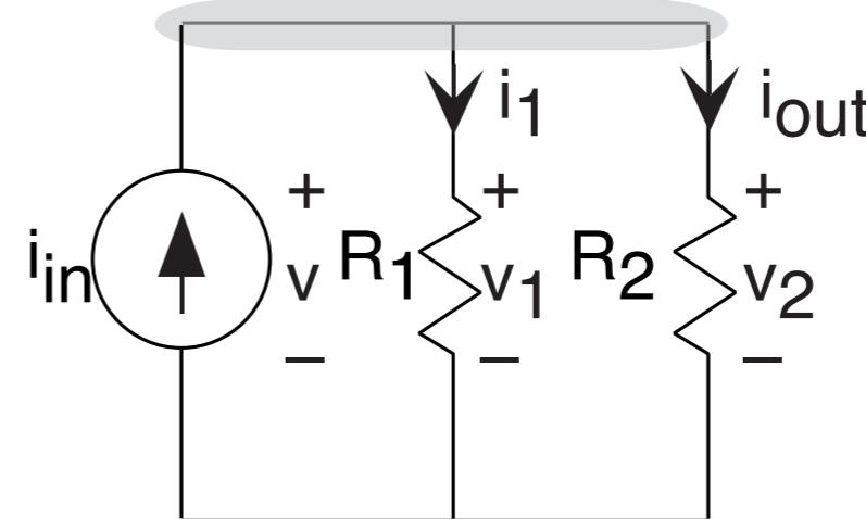
$$i_{out} = \frac{R_1}{R_1 + R_2} i_{in} \implies v = v_2 = \frac{R_1 R_2}{R_1 + R_2} i_{in}$$
