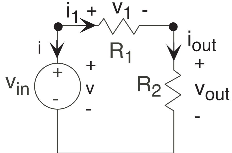
$$v_{out}(t) = \frac{R_2}{R_1 + R_2} v_{in}(t)$$
