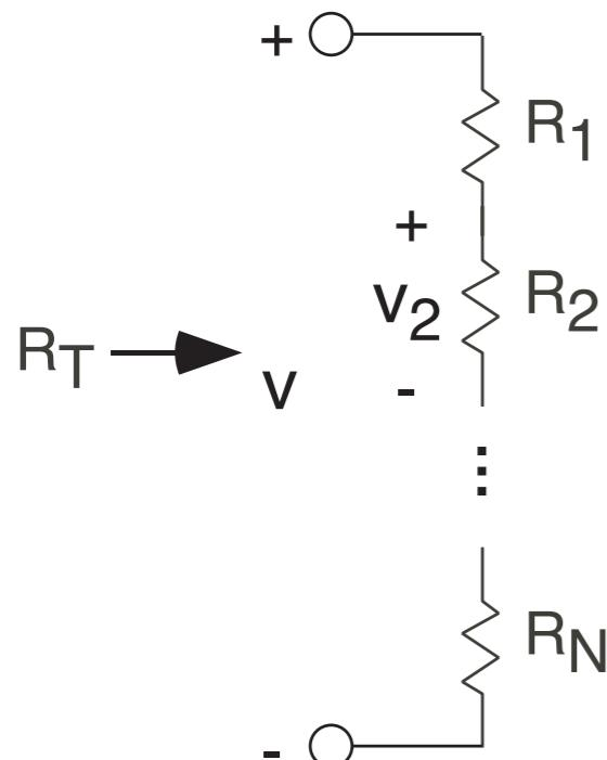
$$R_T = \sum_{n=1}^N R_n \quad v_2 = \frac{R_2}{R_T} \cdot v$$
