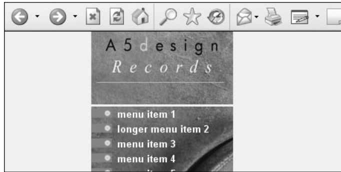
FIGURE 10.6 Space that is added between the logo and the menu area in IE 5, 5.5, and 6 because <DIV> tags were not wrapped around the image.
