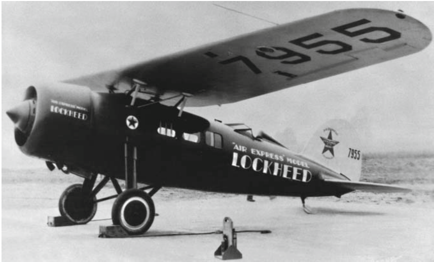
Fig. 9.4 The Vega Air Express, with NACA-designed cowling, broke the transcontinental speed record in 1929 (courtesy NASA)
