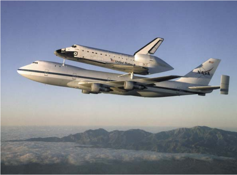
Fig. 7.7 By taking off in a horizontal attitude, the carrier aircraft becomes the booster, and the piggyback stage is given a free lift part-way to space. The Spacecab concept involves a much more streamlined design (courtesy NASA)
