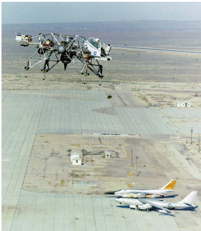
Fig. 9.14 Lunar-based shuttles might resemble this Lunar landing research vehicle, used by Apollo astronauts to practice Moon landings (courtesy NASA)
