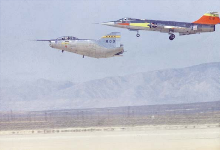
Fig. 1.15 M2-F2 lifting body landing with F-104 Starfighter flying chase, 1966 (courtesy NASA)
