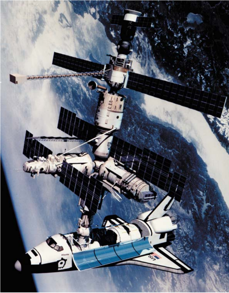
Fig. 4.5 “Technical rendition” of STS-71 Shuttle orbiter docked to the Russian Mir space station. Note the contrast between the modular station and the nonmodular Shuttle (courtesy NASA)
