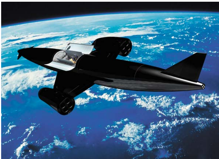
Fig. 12.4 Skylon spaceplane in low Earth orbit. It requires no external tanks, drop-off boosters, stages, or carrier aircraft. It is the epitome of the advanced spaceplane (courtesy Reaction Engines Limited)
