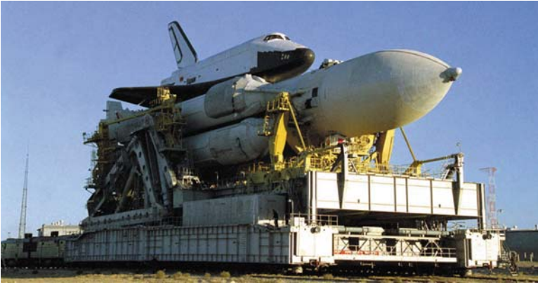
Fig. 7.5 Buran spaceplane piggybacking its way to the launch pad atop its Energiya booster. Russian rockets are transported horizontally before erection at the pad (courtesy http://www.buran-energiya.com )
