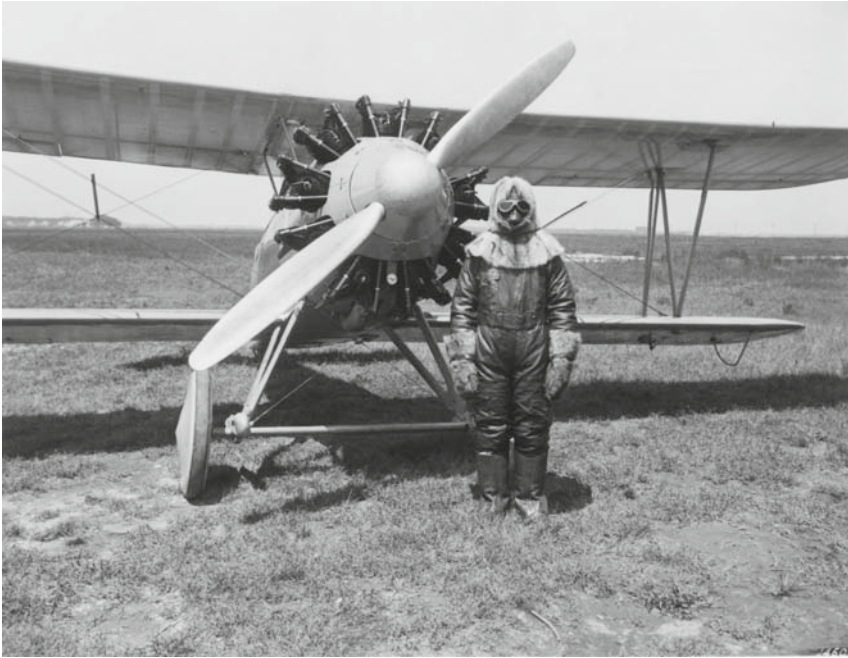
Fig. 1.2 Fully suited aeronaut prepares to take Wright Apache to high altitude in 1928. The 18-cylinder radial engine was a significant advancement over the Wright Flyer (courtesy NASA)
