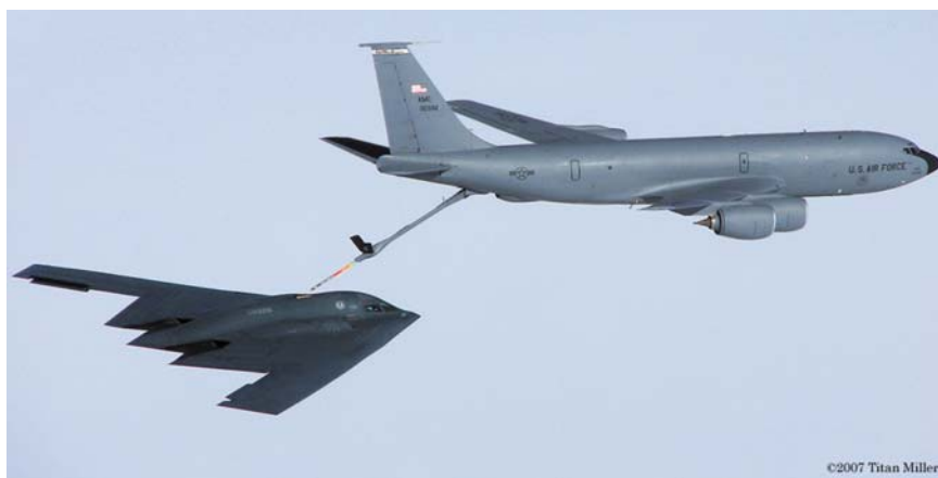
Fig. 9.17 Spaceplanes may refuel in flight after taking off, like this B-2 Bomber being refueled by a US Air Force KC-135 tanker (courtesy USAF)
