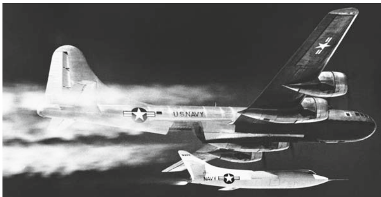
Fig. 1.10 The Douglas D-558-2 Skyrocket is dropped from P2B-1 mothership (Navy version of the USAF's B-29 Superfortress ) in 1956. Although technically not an X-plane, it nevertheless contributed much to aeronautics research (courtesy NASA)
