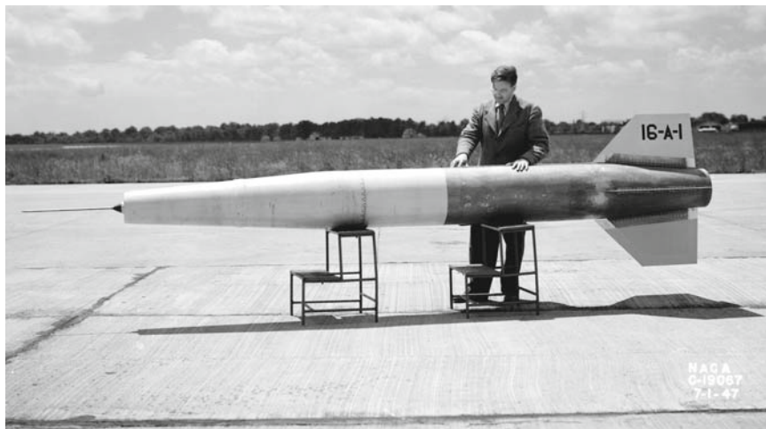
Fig. 8.2 Ramjet missile showing simple tubelike construction (courtesy NASA)
