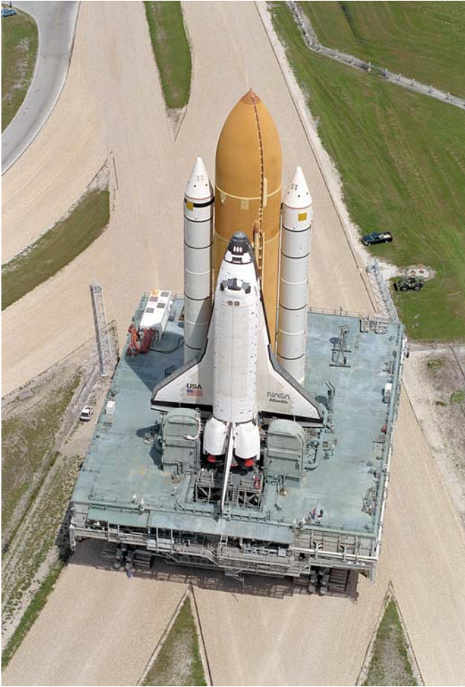
Fig. 9.2 The Space Shuttle on its mobile launch platform and crawler-transporter, inching its way toward the launchpad. The Shuttle carries virtually all its propellants in an external liquid fuel tank and two solid rocket boosters (courtesy NASA)
