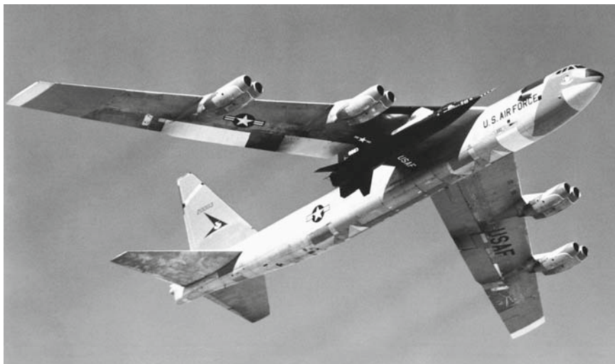
Fig. 9.1 The X-15 rocketplane mated to its mothership carrier, the venerable B-52, during a captive flight in 1959. This baby spaceplane never took off under its own power (courtesy NASA)
