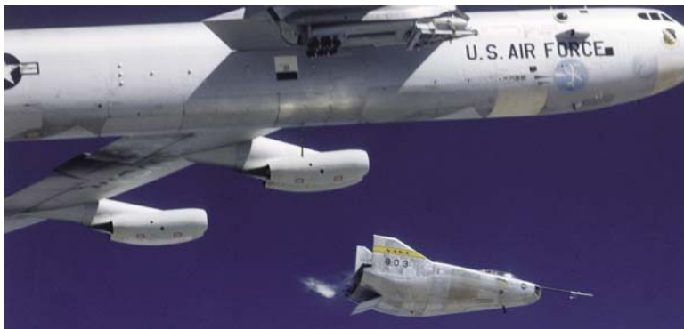
Fig. 1.16 M2-F3 in-flight launch from B-52 mothership in 1971 (courtesy NASA)
