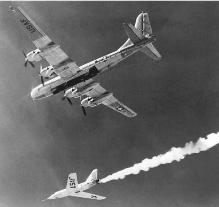
Fig. 1.11 Bell X-2 ignites rocket engine after drop from B-50 mothership, 1955 (courtesy NASA)
