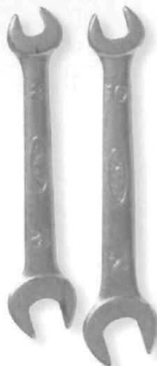
Open-ended spanner wrenches These tools have different sizes at each end.
