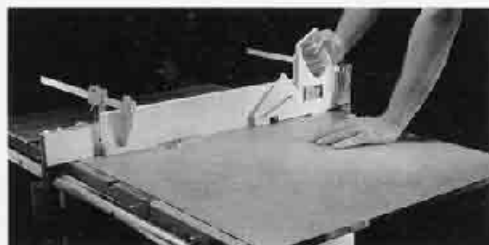
2. Table Saw. Cut laminate face up, using a carbide-tipped blade. Clamp hold-down strip to fence to avoid chatter.
