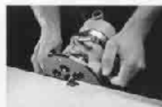
5. Trim the excess laminate with a straight flush carbide cutter in a router or laminate trimmer.
