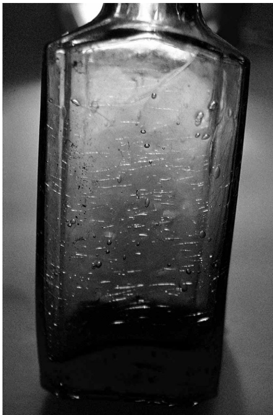
Figure 4.20 Spontaneous cracking of glass during burial, termed frosting, since the overall effect, resembles frost on windows.
