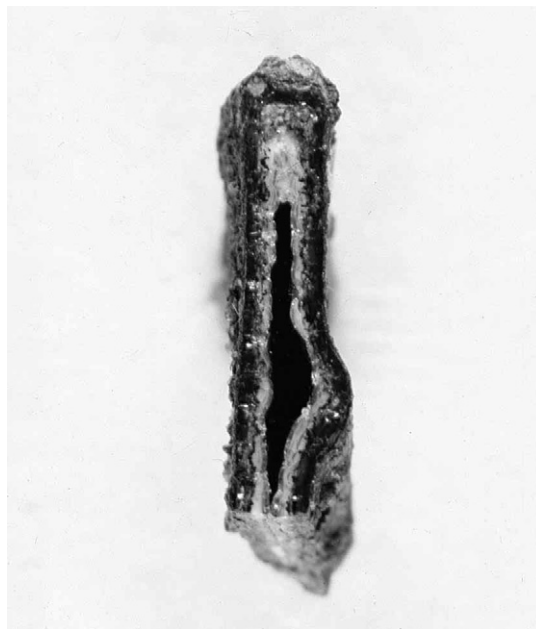
Figure 4.23 Section through a fragment of deteriorated glass, showing the invasion of the interior. (Courtesy of J.M. Cronyn).
