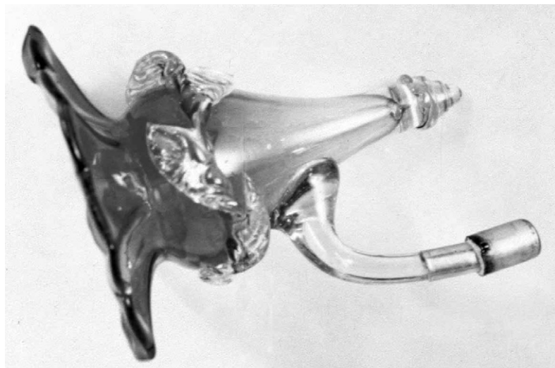
Figure 7.60 A broken glass arm from an épergne repaired by extending the metal pot into which it had fitted. The pot extension replaces the missing end of the arm. Similar repairs are carried out on chandelier arms. (Courtesy of K. van Lookeren Campagne).
