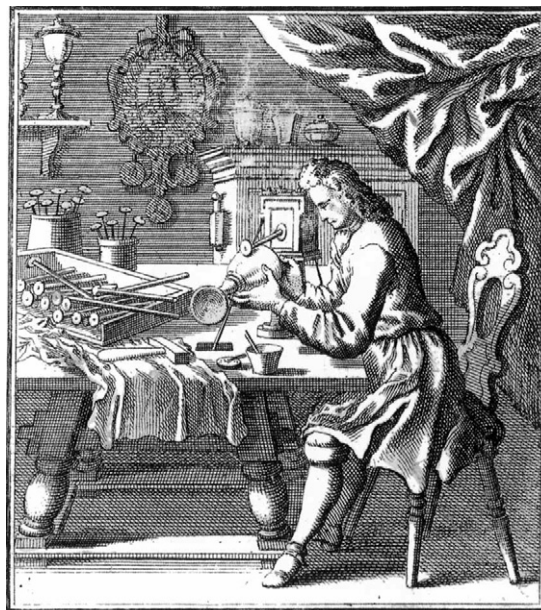
Figure 3.20 Glass cutting and engraving. An engraver holds a goblet beneath a copper wheel powered by a treadle (omitted from the print). On the table are several other wheels, and bowls of abrasive paste. (© V&A Picture Library).
