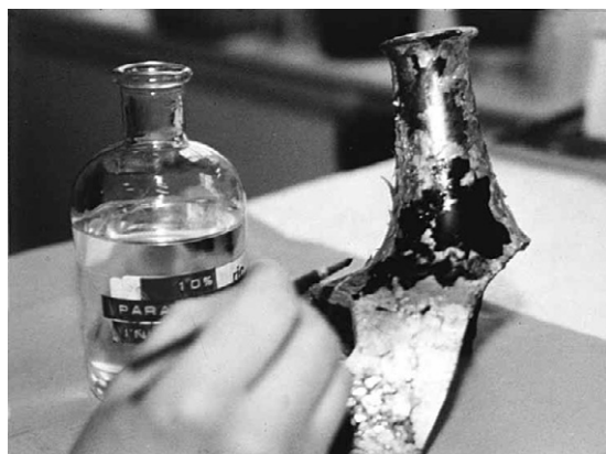
Figure 7.15 Application of a consolidant (10 per cent Paraloid B-72 in toluene) to flaking glass by brush.
