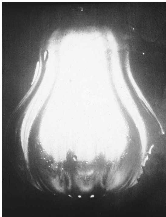
Figure 4.15 Close-up view of a weeping glass vessel, showing the drops of alkaline moisture, which form on the surface. (© Copyright The British Museum, London).
