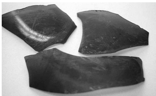
Figure 4.4 Fragments of glass deliberately scratched by filing during a damaging attempt at repair.
