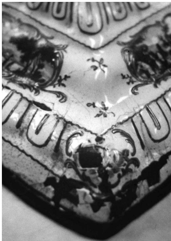
Figure 7.57 A damaged enamelled candlestick showing loss of the enamel surface and damage to the copper substrate.
