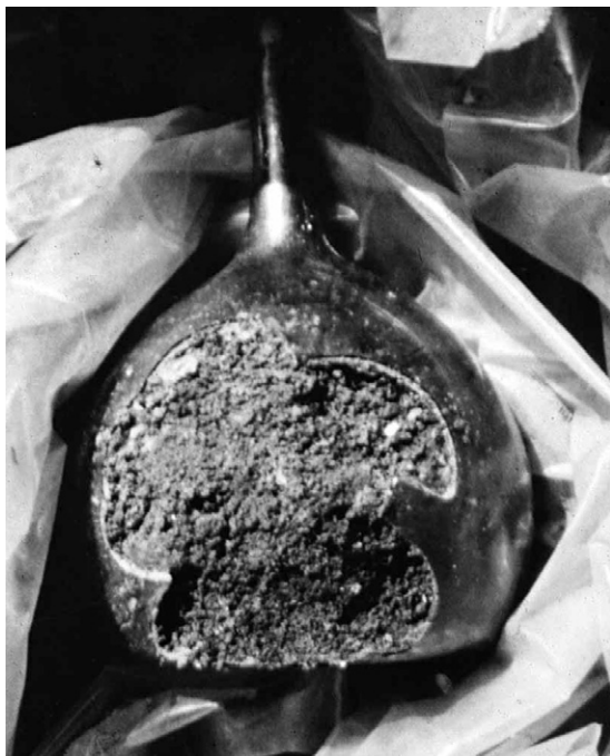
Figure 4.27 Marine concretion inside a glass flask, which has hardened on drying. Soluble salt crystals have formed on the surface of the concretion. (Courtesy of the Institute of Nautical Archaeology, Texas).
