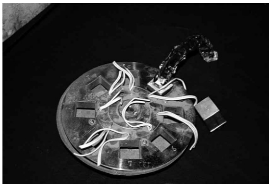
Figure 7.62 A receiving plate for chandelier arms. In this example the holes to receive the metal pots into which the glass arms are fitted, are square.
