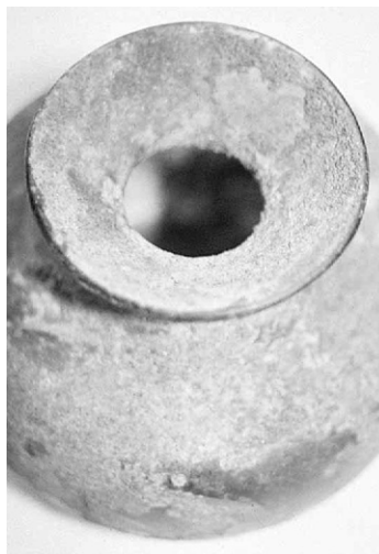
Figure 4.9 Iron corrosion products deposited on a glass flask, during prolonged burial next to an iron object.
