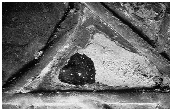
Figure 4.13 Medieval glass which has formed an encrustation due to prolonged exposure to the atmosphere. Part of the crust has fallen away, exposing the blue glass beneath. (Courtesy of S. Strobl).
