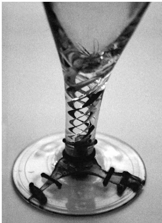
Figure 4.10 Rivets used to repair the foot of a wineglass, which have subsequently corroded.
