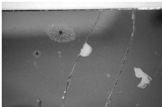
Figure 7.65 Chemical and physical damage of a mirrored glass: deterioration of the amalgam, beginning as dark spots, loss of amalgam, and cracks in the glass.
