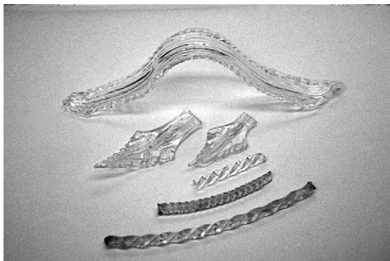
Figure 3.27 Examples of hot-worked (tooled) glass: leaves and canes.
