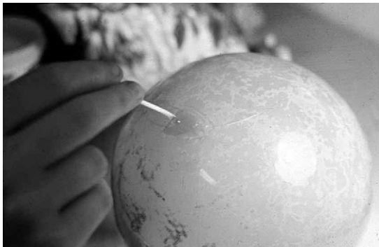
Figure 7.35 A hole in a globular glass lampshade, restored by dripping resin through a small hole in the outer side of a two-piece wax mould.
