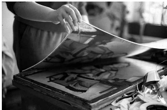
Figure 7.67 Sheet of Scotchint placed behind a deteriorated mirror, to impart a reflective appearance.
