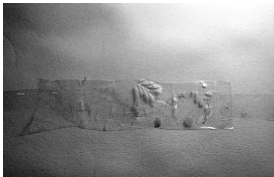
Figure 4.11 Gilding removed from the surface of a glass vessel, on Sellotape used to tape fragments together.
