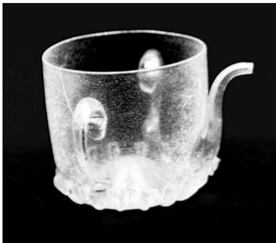
Figure 4.17 A crizzled posset pot, on which the network of fine surface cracks can be seen. (© Copyright The British Museum).
