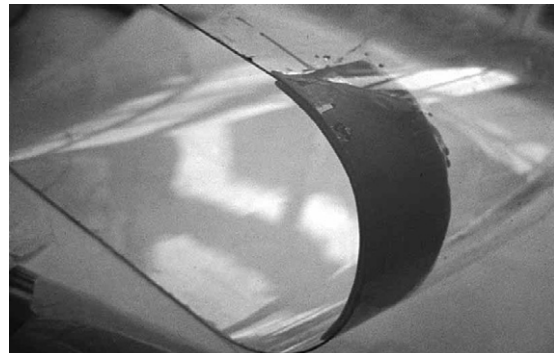
Figure 7.36 Missing section of a glass dome restored by casting resin into a mould made of a double thickness of dental wax.
