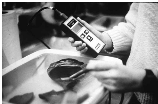
Figure 7.6 Use of a conductivity meter to monitor the desalination process.
