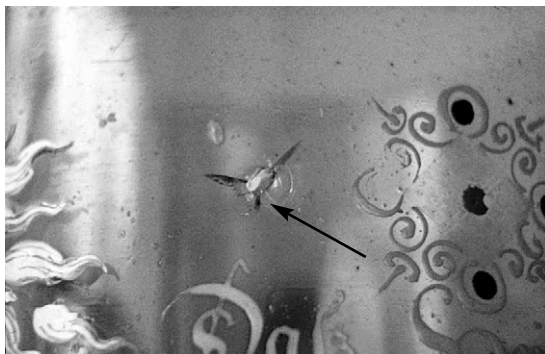
Figure 4.1 A stone in glass, which has subsequently caused the glass to crack.
