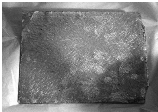
Figure 7.66 Fingerprints formed by acid from fingers, in an amalgam surface.
