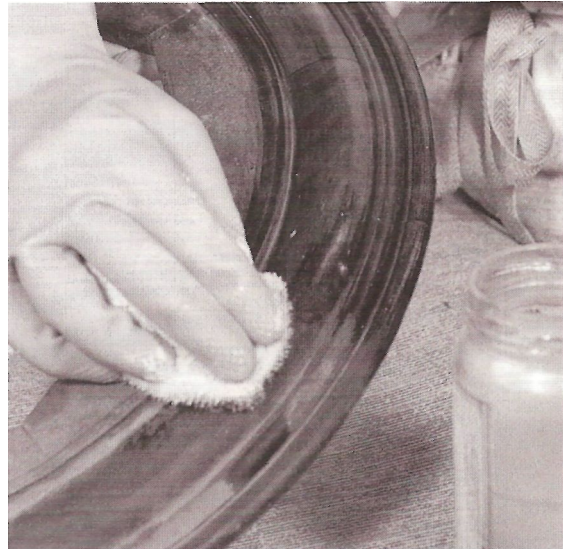
Fig 100 Raw linseed oil, pure turpentine and methylated spirit in equal measures is a mild cleaner which is ideal for use on an item that is very dirty. Keep the mixture well-shaken as it will settle out. Do not clean too large an area at a time. If the job is particularly dirty a piece of grade 0000 steel wool can be used after the mixture has been applied
