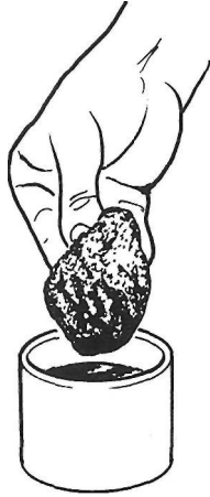
Fig 71 Totally immerse the wadding in thinned polish. Squeeze out about 50 per cent so that the wadding holds the shape of the half pear
