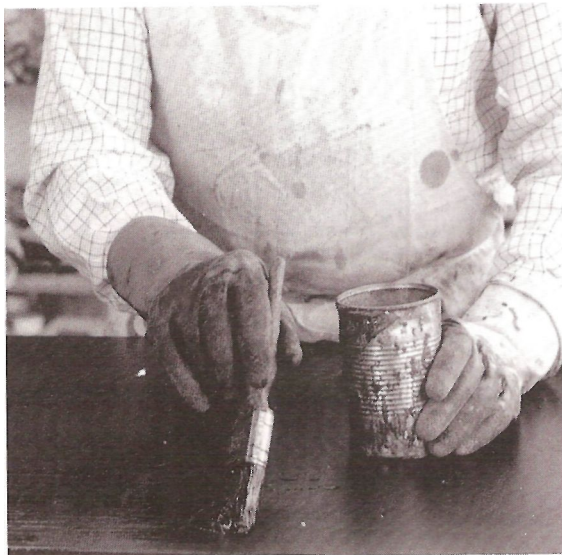
Fig 21 Wear rubber gloves and a long-sleeved shirt to protect against stripper splashes. Apply the stripper liberally with an old paint brush
