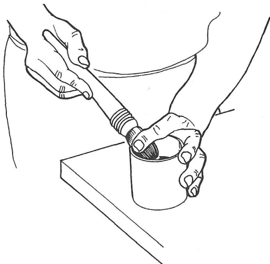
Fig 62 When removing excess polish from a Zorino mop hold it against the side of the container, apply pressure with the index finger and withdraw the brush gently
