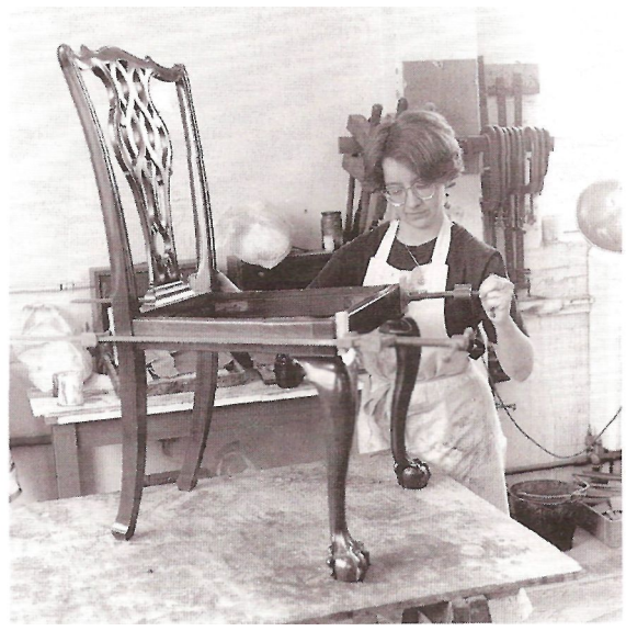
Fig 35 Cramping up a chair with sash cramps - note the use of blocks to protect the wood, Ensure the chair is square before fully tightening
