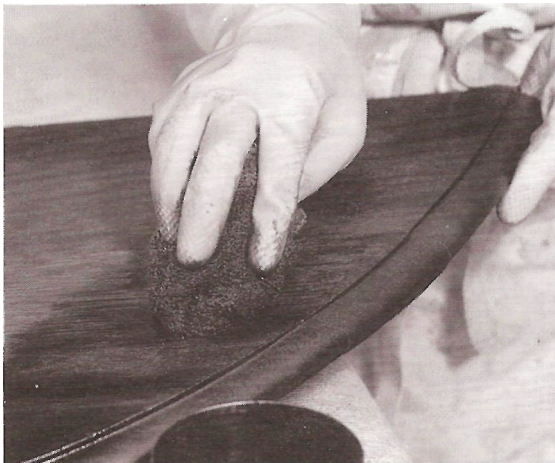
Fig 50 Shading can look effective on the right piece of furniture. Ensure that the line between the light and dark stain is gradual so that it looks more natural
