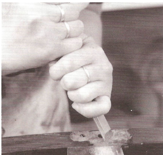
Fig 30 Chiselling the joint clean ready to apply glue
