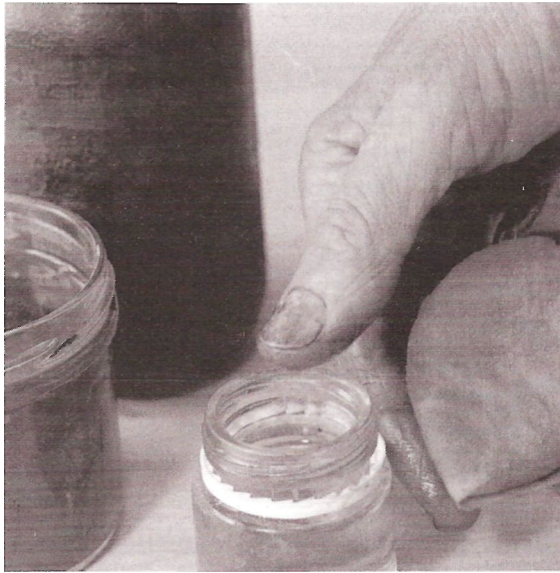
Fig 93 When using oil to lubricate during bodying up or finishing off it should be applied to the base of the rubber. Dip the thumb into the pot of oil
