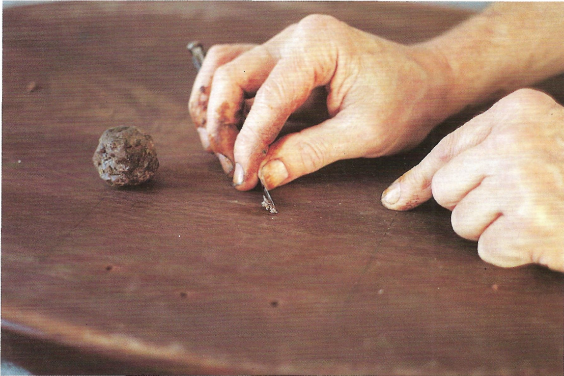
Fig 102 Using the back of the knife excess wax should be removed to leave the surface flat. It can now be polished over if necessary
