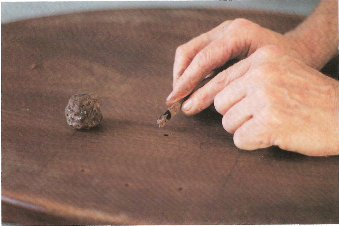
Fig 101 When filling a hole on a piece of furniture that has polish on it a coloured beeswax should be used. Wax can be made or bought in a range of colours
