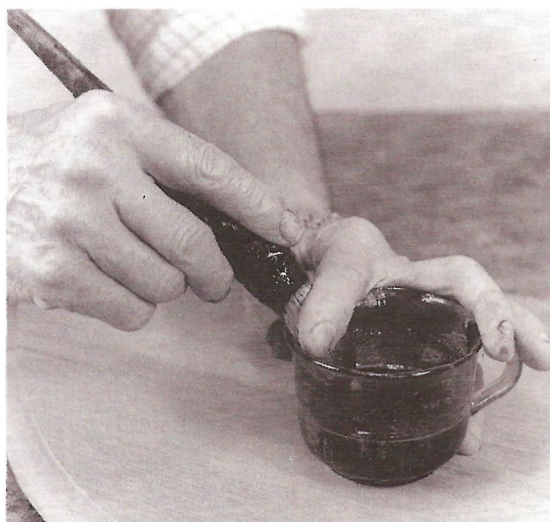
Fig 63 Remove excess polish by holding the brush against the side of the container with the index finger and withdraw the brush
