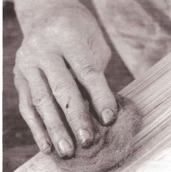
Fig 115 With a piece of grade 0000 steel wool rub gently in the direction of the grain to dull the surface
