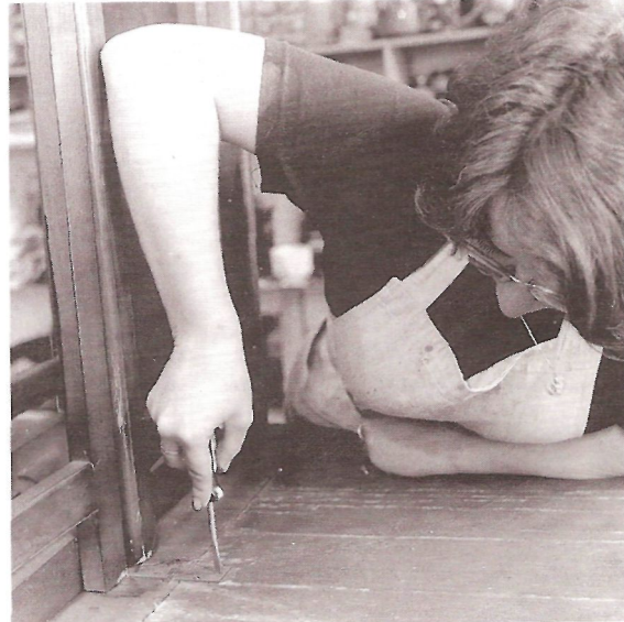
Fig 16 The correct way to use a screw driver. All the pressure should come through the shoulder, and having the screwdriver and the arm in line is essential
