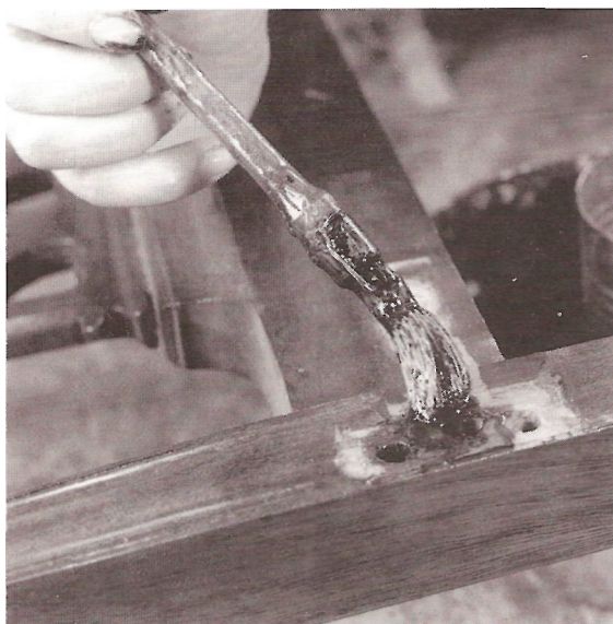
Fig 32 Apply animal glue whilst hot - it should run from the brush without forming drops
