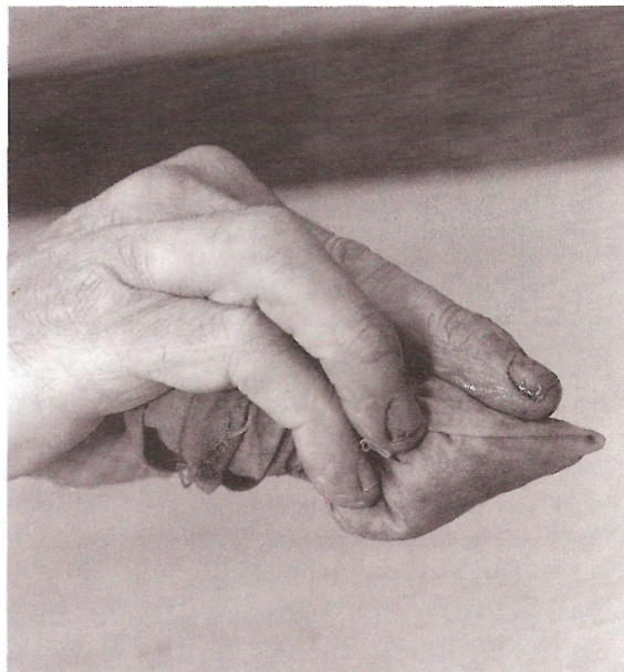
Fig 83 When holding the rubber the third and small fingers are tucked up and help keep the 'tail' in place
