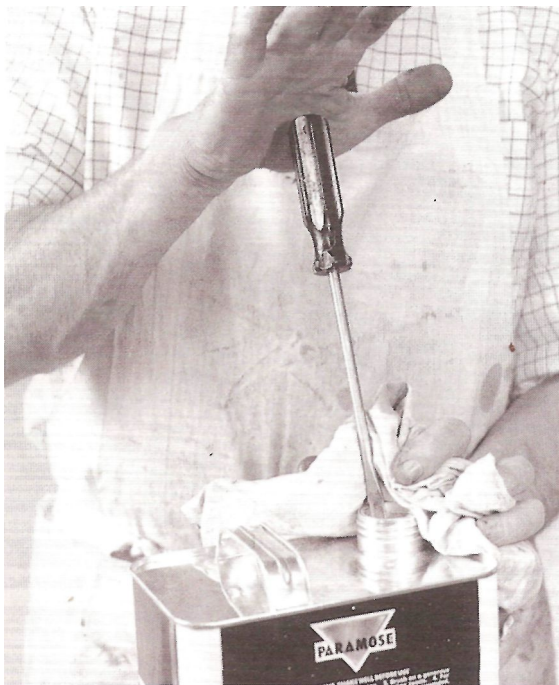
Fig 20 Opening a new can of methyl chloride stripper -- note the rag to stop the fumes escaping
