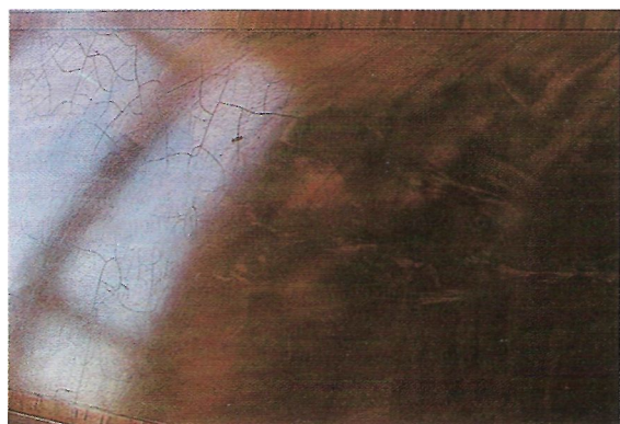
Fig 117 Part of an Edwardian wardrobe showing how polish can crack to produce Chinese writing. This is usually the result of using two incompatible polishes
