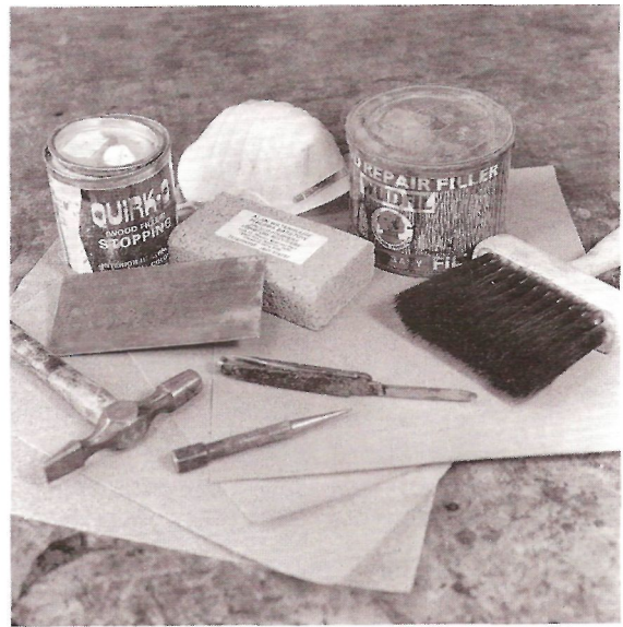
Fig 37 All the materials you will need for timber preparation
