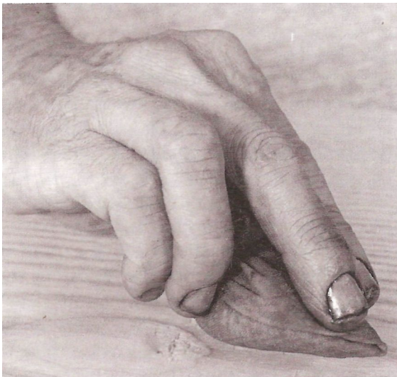
Fig 81 Hold a rubber with the index and second finger at the front - do not apply pressure with the thumb
