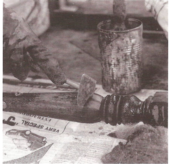
Fig 26 A moulding scraper can be used on shaped pieces
