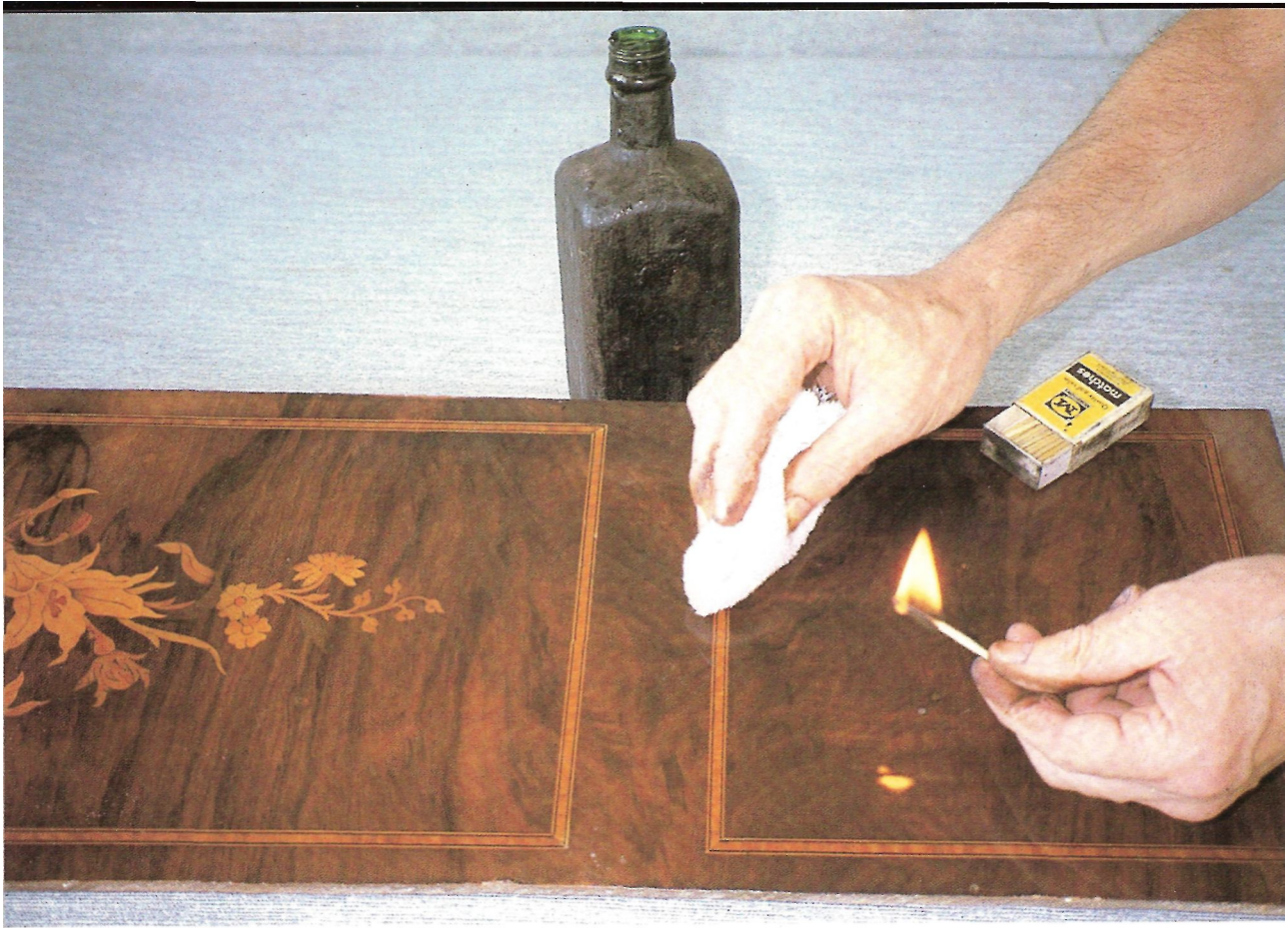
Fig 119 The most dramatic way to remove a white ring mark is to drive it out with heat. Slightly dampen a cloth with methylated spirit and wipe it over the area of the ring, then immediately apply a lighted match to it - this will drive the trapped moisture out. The flames should go out almost immediately because there should be very little methylated spirit on the surface. You may blow out the flame if you wish. The mark will normally be removed at the first attempt but if it has only partly gone the process can be repeated several times. Always allow several minutes between attempts so that the polish does not become soft
