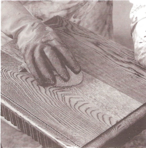
Fig 28 Neutralize stripper with hot ammonia water, applied liberally with a piece of towelling
