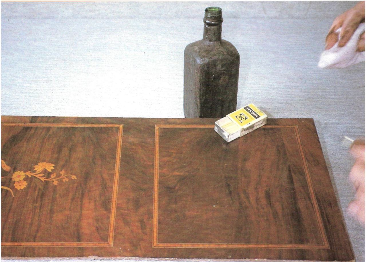
Fig 120 After the white mark has been removed it should be left for a short while and can then be waxed with a soft beeswax. It is not usually necessary to repolish the area
