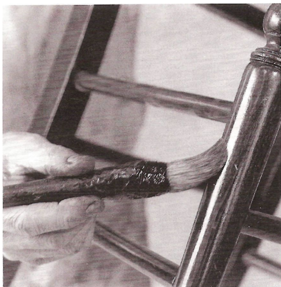
Fig 64 Always coat in the direction of the grain whether the area is small or large
