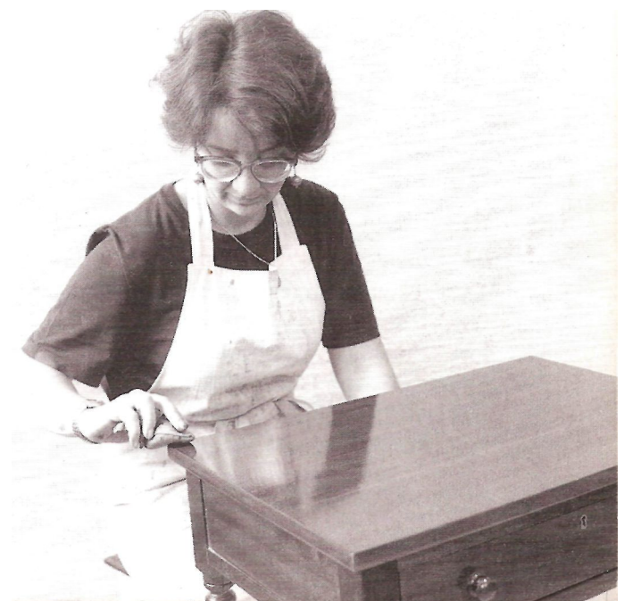
Fig 95 Always come on at a corner, and alternate the corners so you do not get a build up of polish at any one corner
