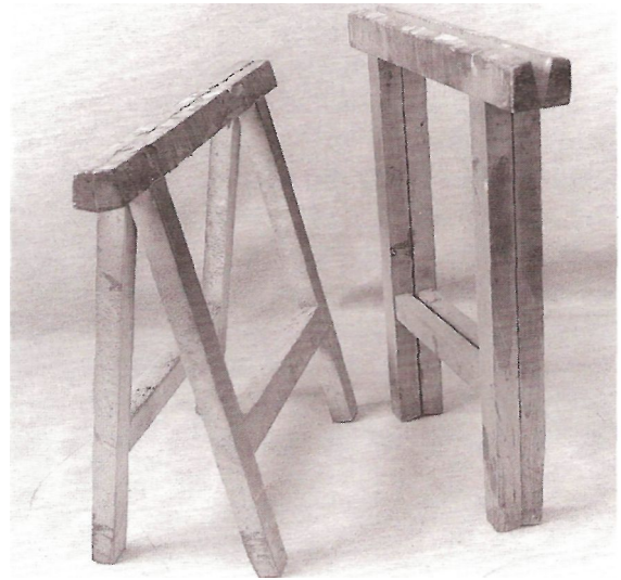
Fig 7 Collapsible trestles: because of the top rail they will not 'walk'
