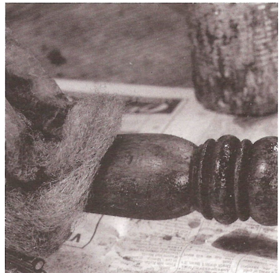
Fig 27 Shape grade 3 steel wool to the job to remove the last traces of old polish
