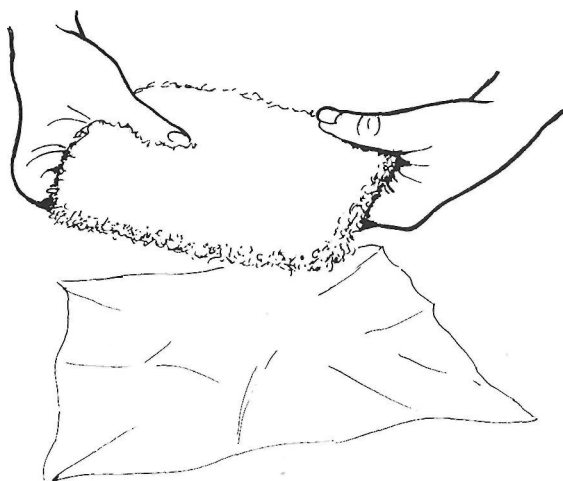
Fig 67 Take a piece of polisher's wadding approximately 200 x 130mm (8 X 5in) long
