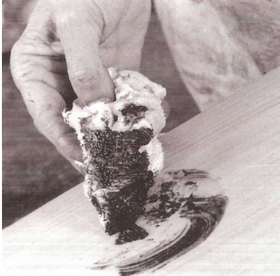
Fig 114 Apply wax with a piece of towelling. A darker wax is used here for emphasis, though we normally select a colour of wax closest to the colour of the wood
