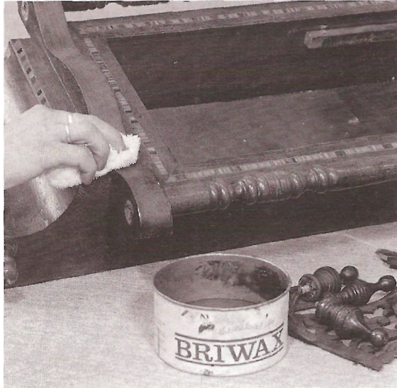
Fig 99 Briwax is a good general cleaner as it is a mild abrasive wax. When using Briwax only tackle small areas as it is a hard wax that is difficult to spread. It is ideal for use on items that are dirty but where the polish is still in a good condition and does not require stripping
