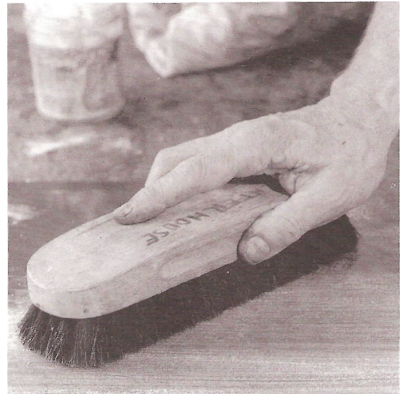
Fig 113 Gently and evenly brush the pumice with a dulling brush to abrade the surface and so dull it
