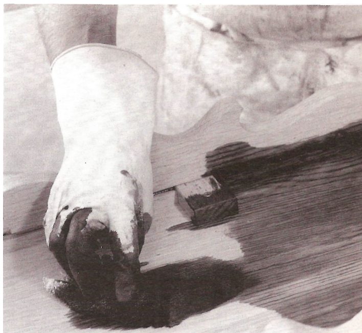
Fig 57 An old piece of towelling can be used to stain large areas. Apply liberally and wipe of excess stain with a clean rag in the direction of the grain
