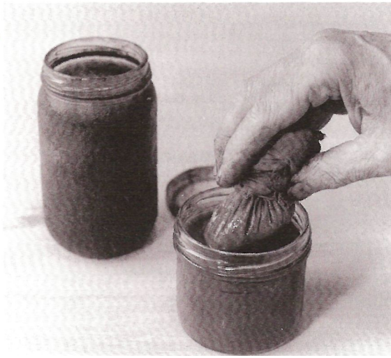
Fig 86 Charge the rubber by dipping it into the container of polish. Do not remove the cloth
