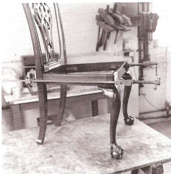
Fig 36 The sash cramps can safely be left in place. Be careful not to walk into the projecting cramps, and always place the cramped piece out of the way until the cramps are ready to remove
