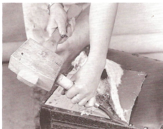
Fig 14 Use a ripping chisel and mallet to remove old upholstery. Work in the direction of the grain
