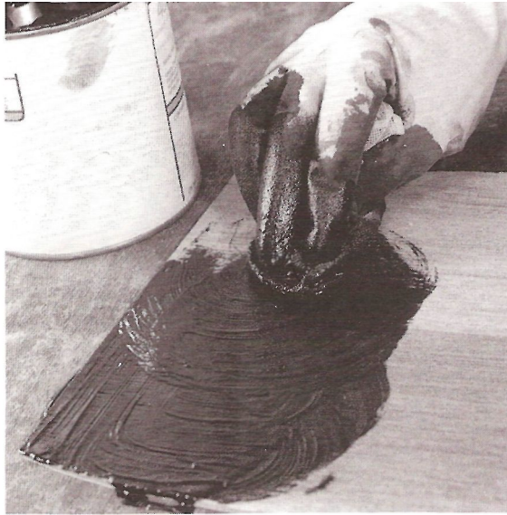
Fig 58 Apply grain filler by rubbing in circles, pushing it into the grain
