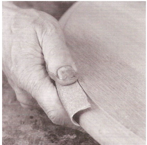
Fig 44 Shape the garnet paper around the mould
