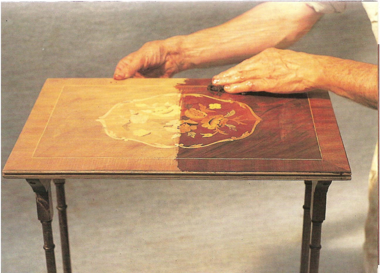
Fig 103 Using raw linseed oil and pure turpentine as a stain on a reproduction inlaid table
