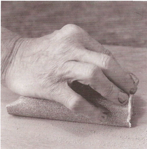
Fig 42 Wrap the garnet paper round the cork block. The heel of the hand applies pressure
