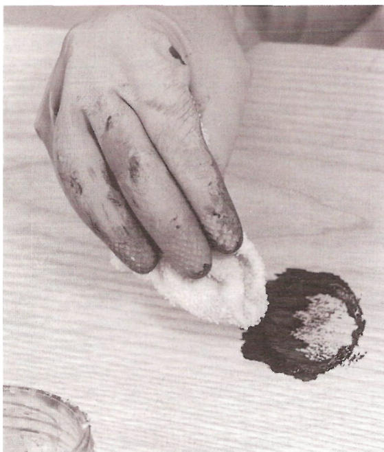
Fig 45 When removing an ink stain with bleach (the best being oxalic acid) wear rubber gloves and use a piece of towelling to apply it. Apply the bleach to the area of the stain very liberally and allow it to dry naturally — the mark will fade as the bleach dries. If the mark has not been removed by one application keep applying it until it is no longer obvious. After the mark has been removed it is wise to bleach the whole area around it to ensure you are not left with a very light patch. Once all bleaching has been carried out the area should be wiped down with clean water to ensure that all traces of bleach have been removed
