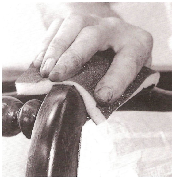
Fig 66 When using a sanding pad it can be shaped to the piece being smoothed
