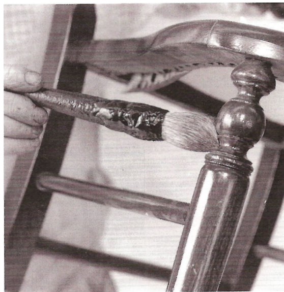
Fig 65 When coating turnings hold the brush lightly at the end and flick it gently, thus avoiding getting the turnings too wet
