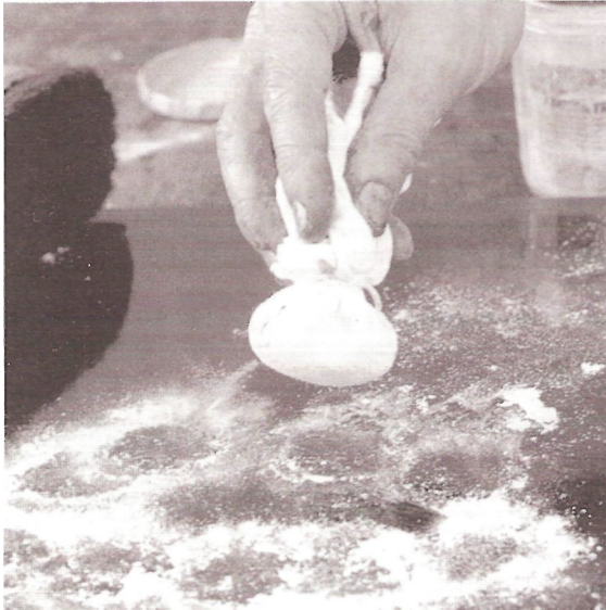
Fig 112 Apply pumice powder to the job using the pumice bag
