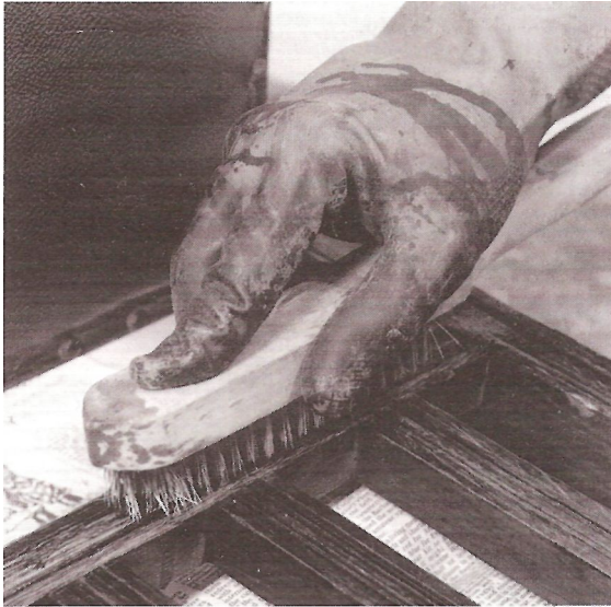
Fig 25 A wire brush can be used to get into grooves and carvings
