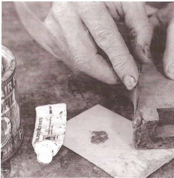
Fig38 Filling a corner with epoxy resin filler. Do not mix too much as it hardens quickly
