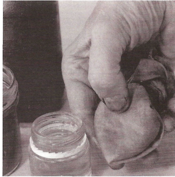
Fig 94 Put a small amount of oil onto the bottom of the rubber and then spread it evenly over the polished surface
