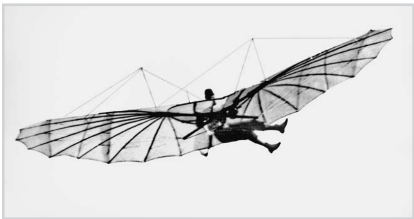
Otto Lilienthal controlled his gliders by shifting his weight to change the craft's center of gravity.
