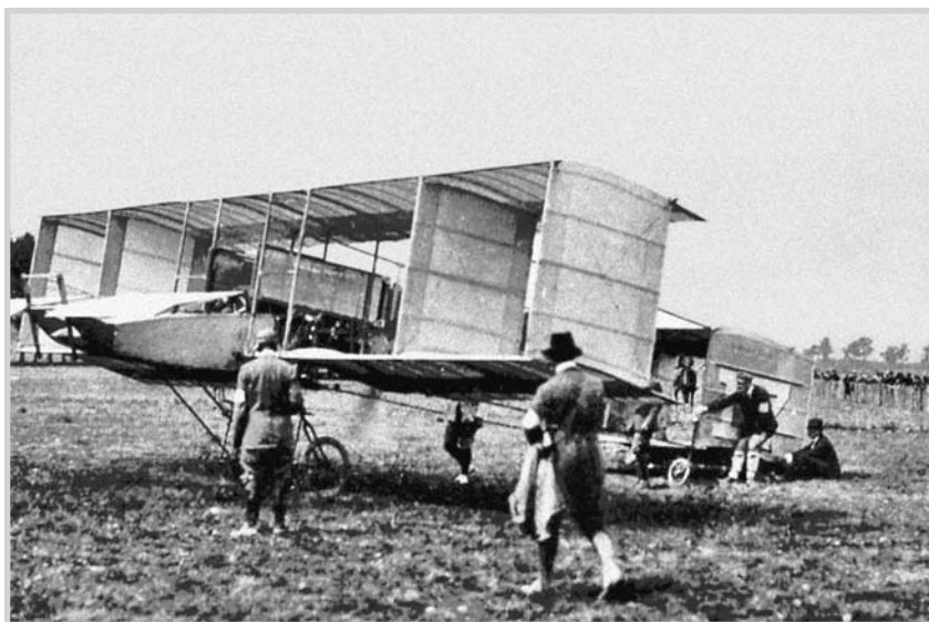
Afraid of falling off to either side, Gabriel Voisin equipped his biplanes with fabric panels between the wings to prevent sideslips.
