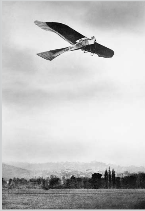
The Rumpler Taube shows off its thin, bird-inspired airfoil. Although Taube is German for dove, Austrian designer Igo Etrich reportedly modeled this airplane's graceful wing after the zanonía seed.
