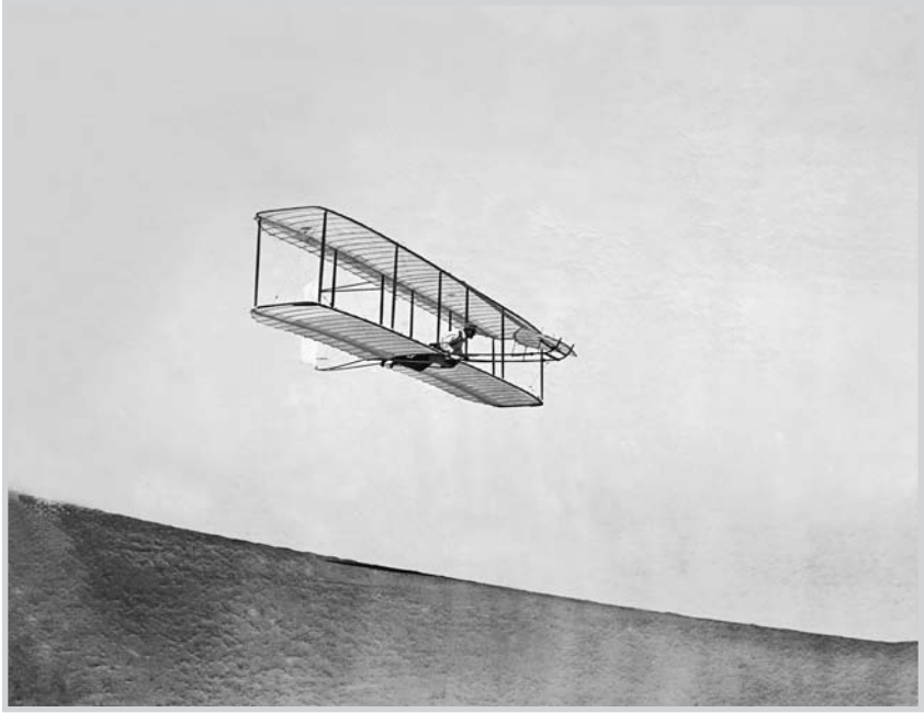
Controllable with the addition of a movable rudder, the Wright 1902 Glider set the stage for the Wright brothers' invention of the airplane the following year.
