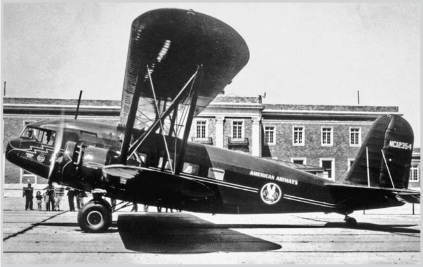
Engine cowlings and retractable wheels could not help the Curtiss T-32 Condor, a 1933 airliner rendered instantly obsolete by the Boeing 247.
