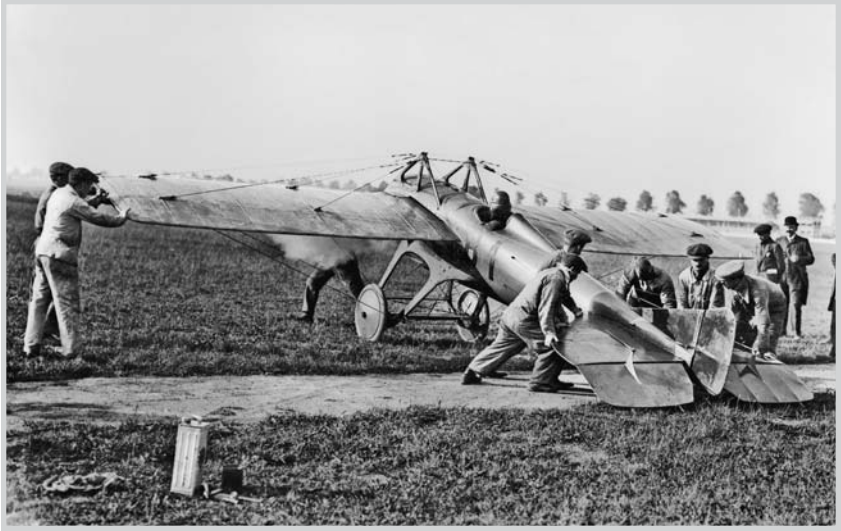
With its streamlined fuselage, the Deperdussin racer achieved a speed of 125 mph (200 km/h) in 1913.
