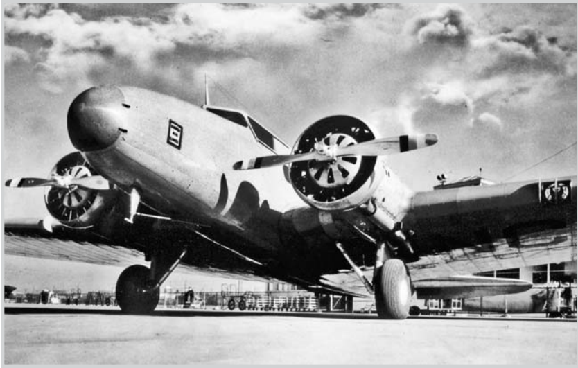
The Boeing 247 was initially delivered with two-bladed, fixed-pitch propellers.
