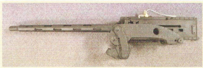
Colt MG40 7.7mm aircraft machine gun, one of several such weapons held by the Broome Museum. This is identical to the weapon used by Gus Winckel on 3 March 1942. When fired from aircraft the barrel is designed to be cooled by the slipstream. In Winckel's case it would have been too hot to hold after just a few seconds of firing. He rested the barrel on his forearm which was badly burnt. (Authors' collection)
