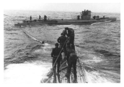
U-116 takes on fuel at sea, photographed from the deck of the supply-vessel U-406. These operations, usually carried out near the Azores (far out in the Atlantic and beyond the range of Allied aircraft) enabled submarines to extend their stay in the hunting-grounds. Enigma informed the Allies of the location of these rendezvous and made possible the sinking of the supply-ships.
