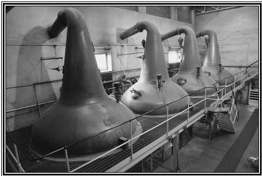
Traditional copper pot-stills are the heart of a distillery.
