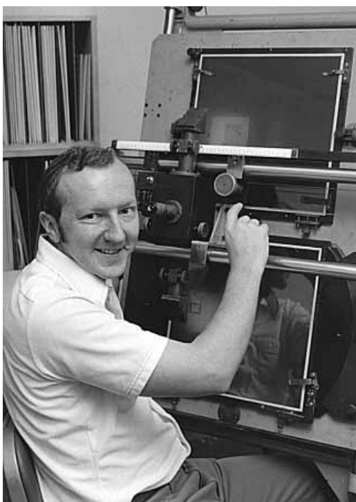
Figure 2.1 Charles Kowal at the blink comparator which he used to discover the first Centaur, Chiron. (California Institute of Technology.)
