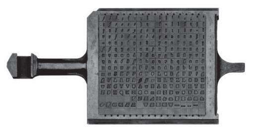
Figure 20.7 A Monotype matrix case. Department of Typography and Graphic Communication, University of Reading.
