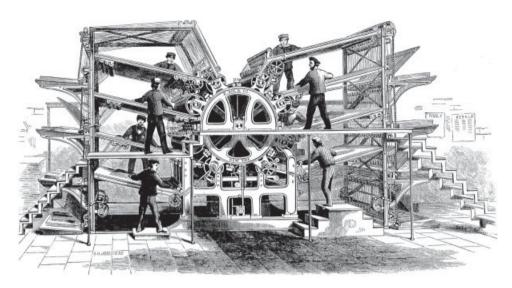
Figure 20.3 Hoe's eight-cylinder printing machine. From Typographic Messenger, September 1866 (St. Bride negative 313).
