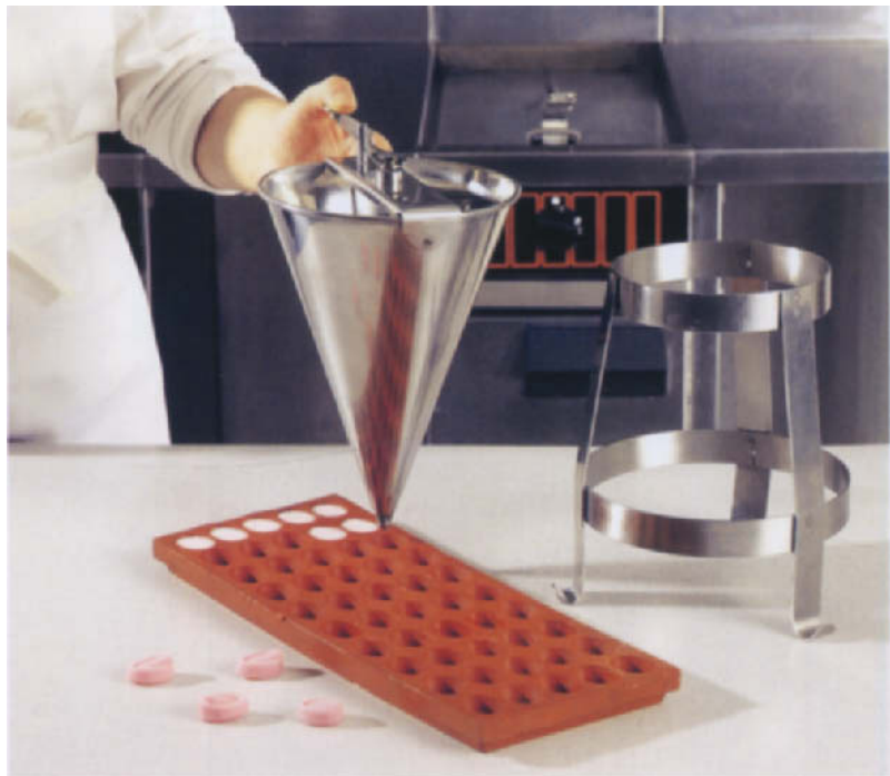
Figure 70 Fondant sweets and centres. Depositing warm fondant into rubber moulds for making sweets and centres
