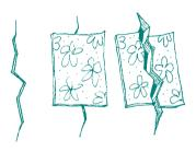
**Cracking Up?...** To determine if a crack in the wall is getting larger, simply glue a piece of wallpaper over the crack. If the crack widens it'll tear the wallpaper as it does so.
