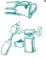
Soldering Pipes... When soldering copper or gluing plastic waterpipes, keep them dry by stuffing a piece of bread into the pipe in either side of where you're working. The bread will soak up any water before it can reach your work area. When finished, turn the water on and the bread plugs will be washed away.
