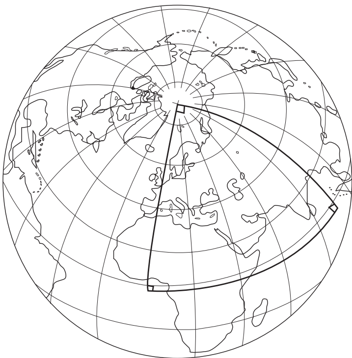
Figure 6. A view of the earth with a triangle superposed. One side is from equator to N. pole along Greenwich meridian; the base is along the equator running from Greenwich meridian to 90 degrees east (or west); the third side goes from equator to N. pole along the 90-degree east (or west) line of longitude.
