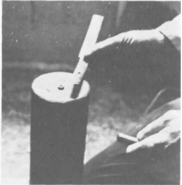
PLATE 16 Now Tedra marks the steel where the holes will be cut for the rivets that hold the handle to the blade.
