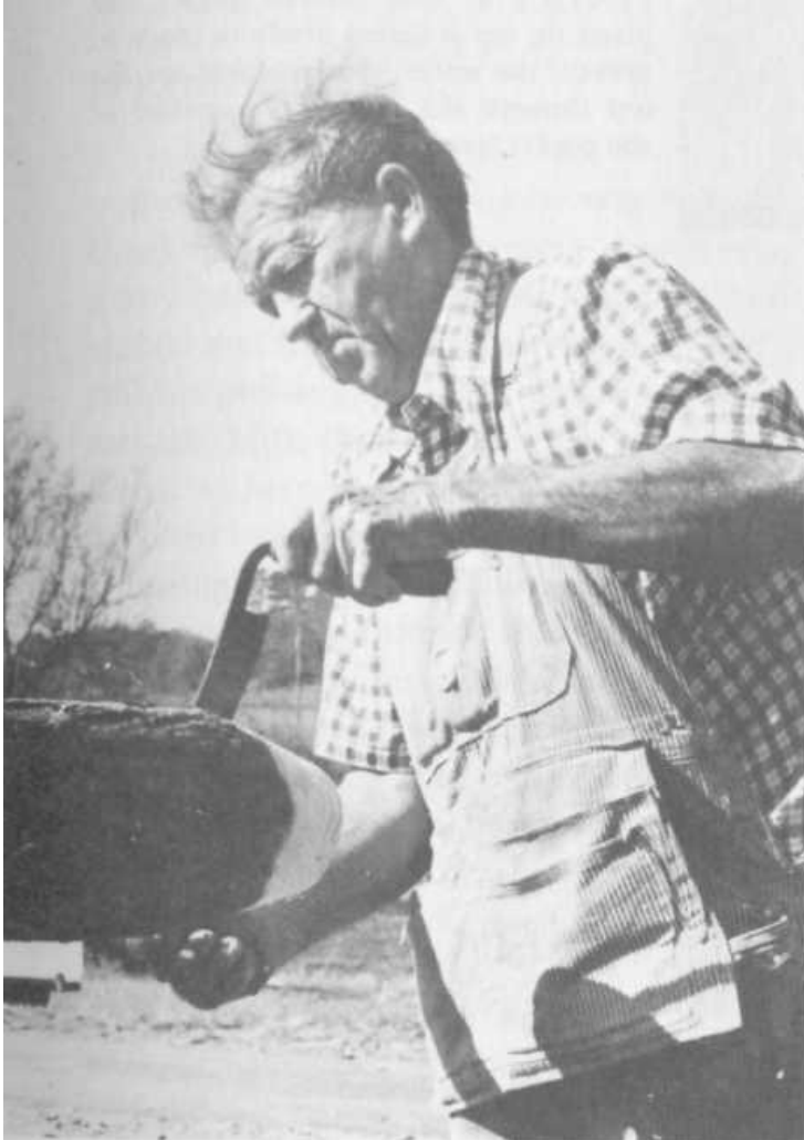
PLATE 313 He then takes another auger and bores a concave hole in the other end of the pipe.
