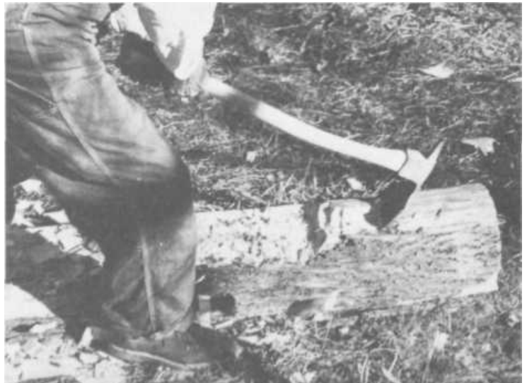
PLATE 407 Then he turns the log flat side down, and, straddling it, begins to smooth the rounded side with powerful strokes. He works forward, taking out large chunks in 4" bites and leaving a trail of chips behind him.
