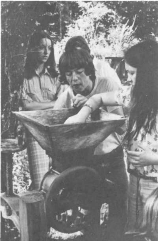
PLATE 395 The wooden disc is placed over the pulp in the slatted tub, and the tub is positioned under the screw.
