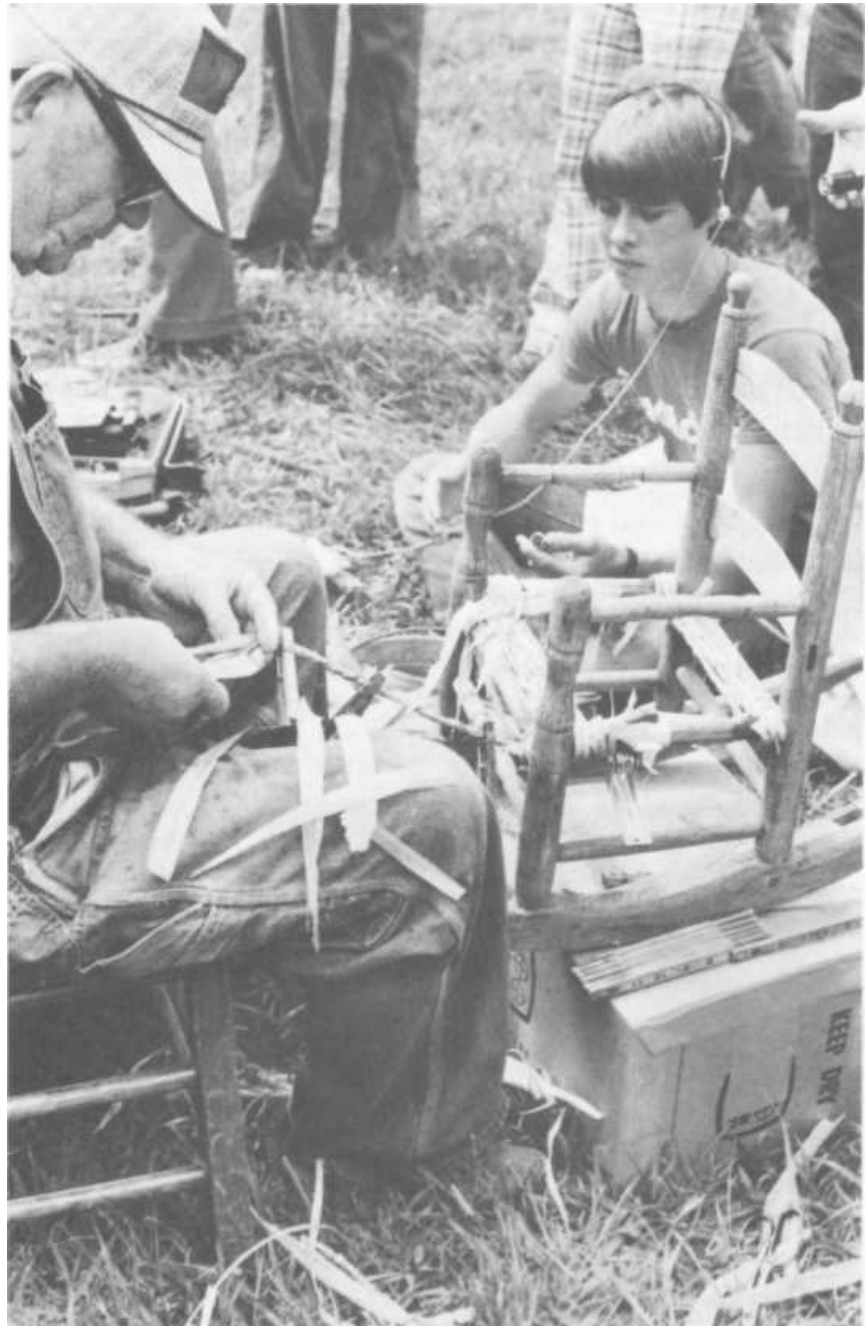
PLATE 416 He makes a long section of rope, clipping it at intervals with clothespins to help hold it together, and then weaves another round.
