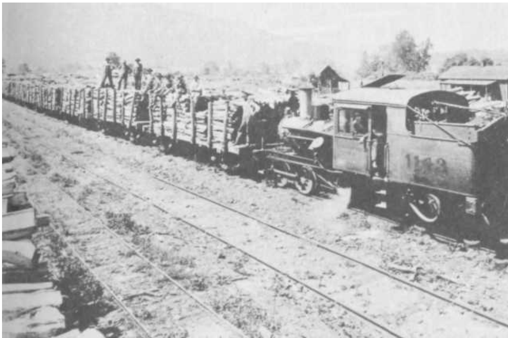
PLATE 273 This photograph shows acid wood being moved into the plant's yard by narrow-gauge railroad. The engine, called a "little Shay," pushes twenty-five to thirty "dinky cars" at a time, each loaded with six to eight cords of wood. (Photo courtesy of Champion Paper.)
