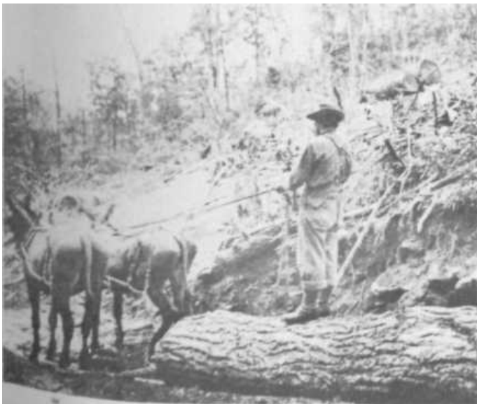
PLATE 276 More often than not, this was the only method of getting a log to the point where it could be reached by the cable from the overhead skidder, or loaded onto a wagon or railroad car. Logs such as this would be dragged down a skid trail from the places where they were cut to the loading area. (Photo courtesy of Champion Paper.)
