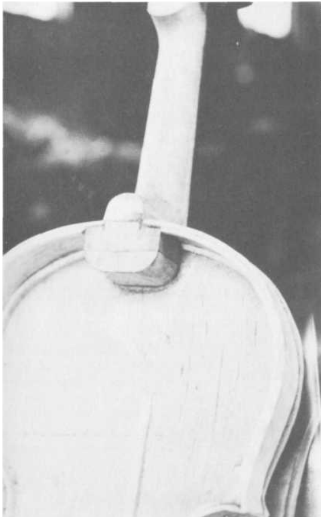
PLATE 117 The neck of the fiddle has been cut out of a block of maple 9"X2 1/4"X2 1/4". It is shaped with a pocketknife and sandpaper. The end may have any design you want. Pegs are tapered so they will tighten in their holes.
