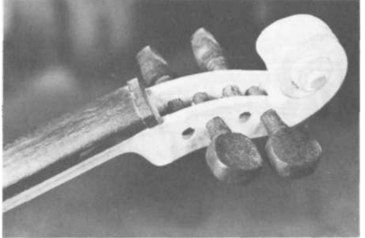
PLATE 117 The neck of the fiddle has been cut out of a block of maple 9"X2 1/4"X2 1/4". It is shaped with a pocketknife and sandpaper. The end may have any design you want. Pegs are tapered so they will tighten in their holes.
