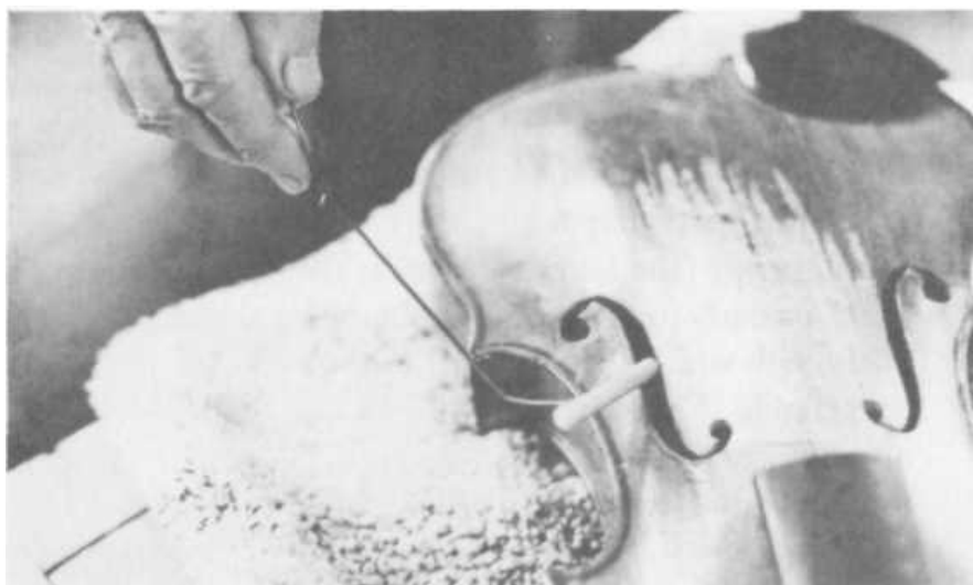
PLATE 139 Garrett adds the sound post with the help of a curved, sharpened wire. He slips it into the middle of the instrument and wedges the post into place, then pulls the wire out.
