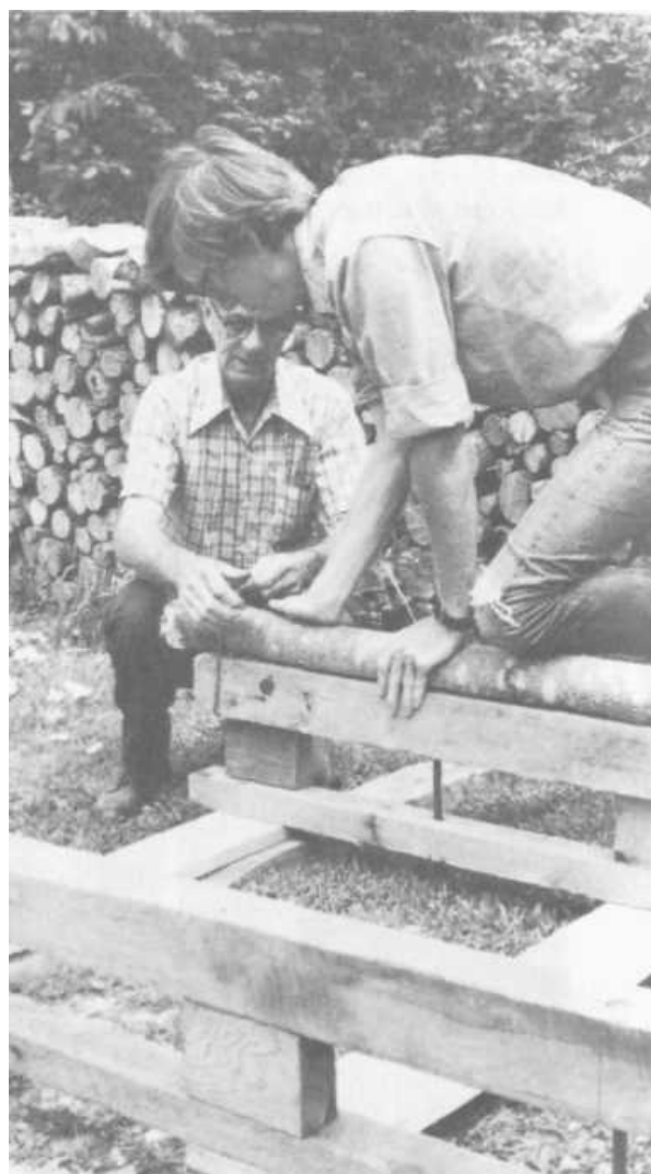
PLATE 178 Wig holds the half sole down while Tedra ties it temporarily with twine.
