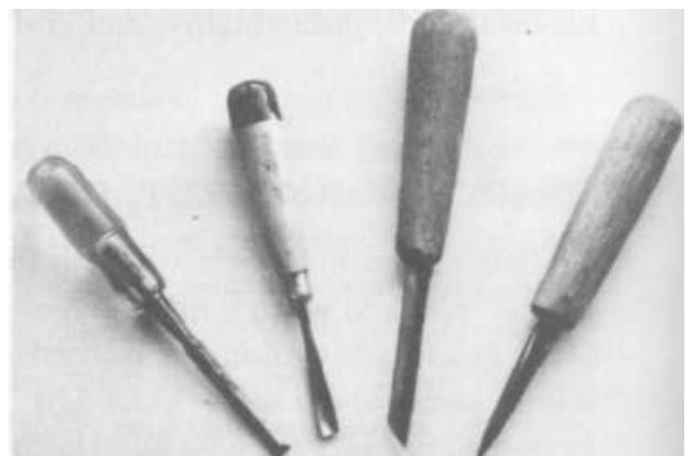
PLATE 42 These are Charles' favorite tools—the knife blades are made from a straight razor blade and a pair of barber's scissors.
