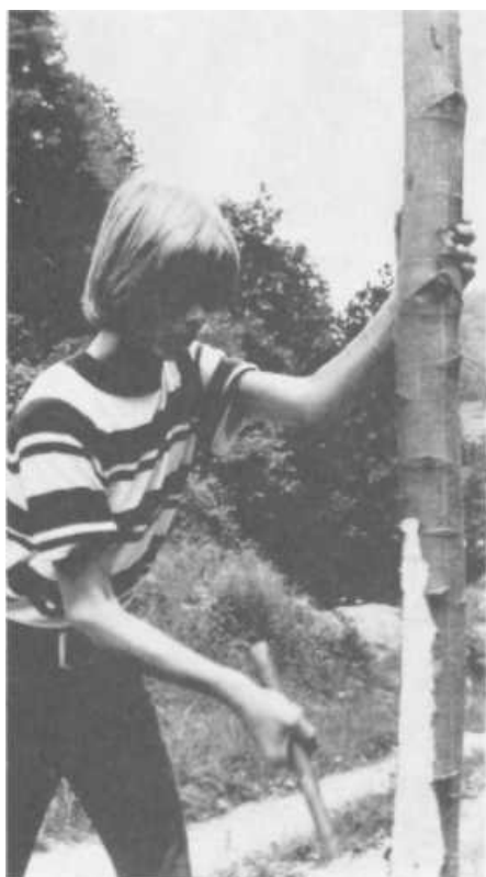
PLATE 174 Now Tedra removes the dowels/standards, turns the sled over, sets a pole in place, and marks where it will have to bend to fit the bend of the runner.
