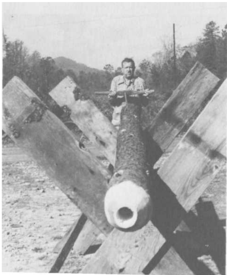
PLATE 311 To make a twenty-foot section of wooden pipe with a ten-foot auger, Garnett bores into one end as far as the auger will go, and then switches ends. He has to be careful not to let the auger bore out the side of the log as it gets in deeper and deeper. He constantly sights along the shaft to make sure it's going straight.
