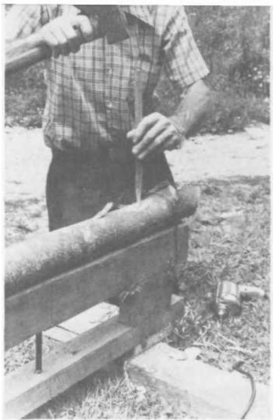
PLATE 180 Then Tedra carves a seasoned half-inch yellow locust peg for each hole (the holes go through the half sole and completely through the runner) and drives them in. As the green half sole seasons, it grips the peg. The excess peg length is cut off with a hatchet or saw.
