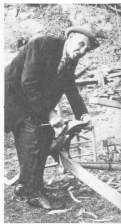
PLATE 155 Here Tom attaches the metal plow point to the foot with a bolt.
