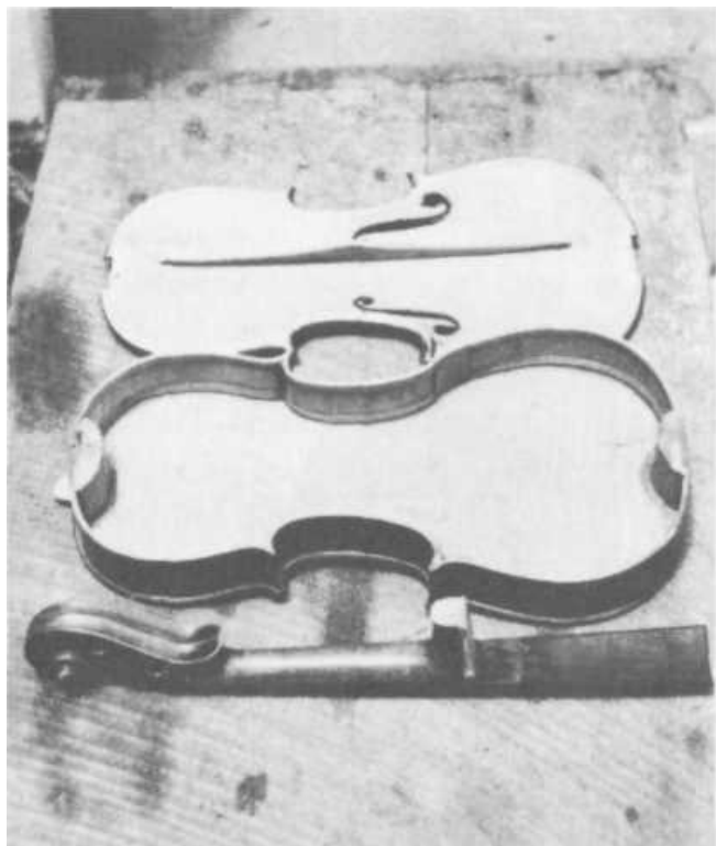
PLATE 137 The top is ready to be glued to the back and sides. Note the blocks at either end of the back to which the sides are glued, the double lining, and the triangular support blocks where the sides come together in the middle.
