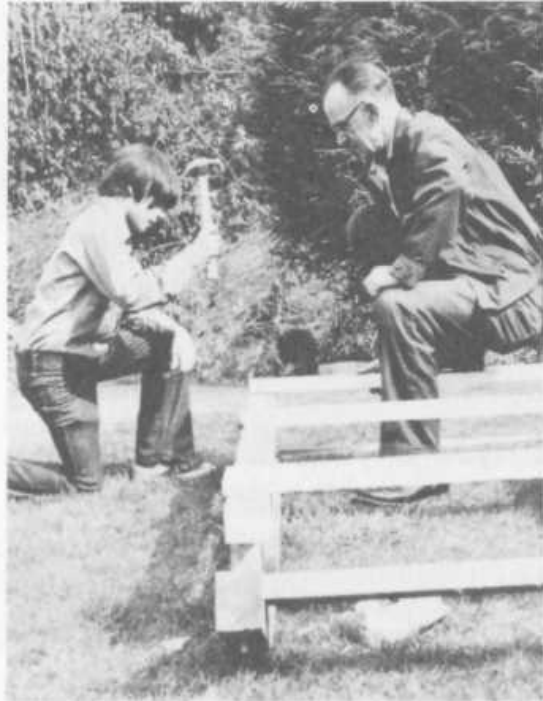
PLATE 171 With the sled upright again, the seasoned oak crosspieces are placed. Tedra first drills holes for the nails to keep them from bending in the hard wood. Then Dwayne drives one nail in each end of the crosspieces and places them off center so they won't interfere with the i" auger used next.
