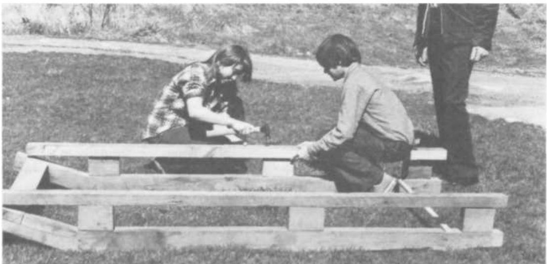
PLATE 167 Now the hemlock sills are tacked into place. They will be set permanently later. They hold the floor of the sled up off the ground so that it can be pulled over rocks and stumps without hanging up.
