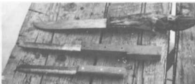
PLATE 25 The knife at the top has a handle made from a deer's foot. The other three knives show various stages of construction of the knife we just saw Tedra make.
