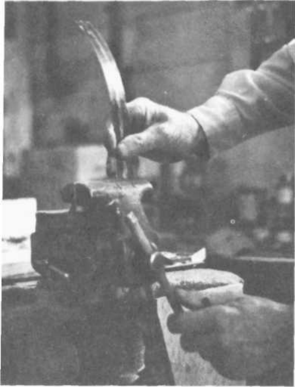
PLATE 10 Tedra places a piece of steel from a phonograph spring in a vice, clamping it at a point that allows the proper length for the knife blade.
