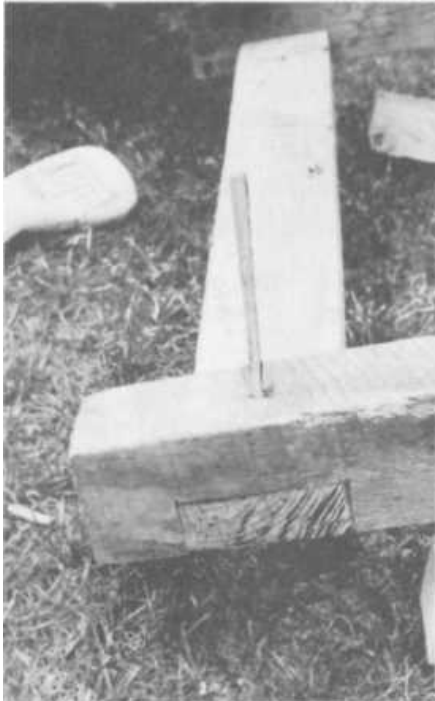
PLATE 170 When the wedge is in place, as shown here, again a saw is used to cut it off flush with the bottom of the runner.
