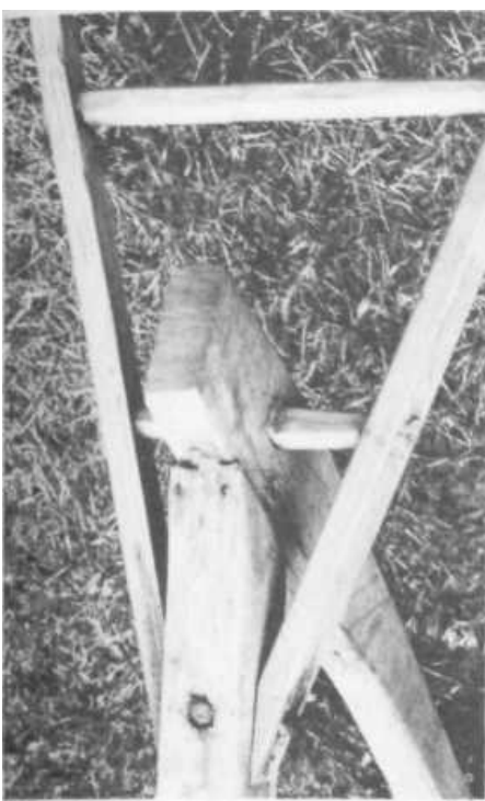
PLATE 153 'This shot, from underneath the plow, shows how the foot is mortised into the underside of the oak beam. Note also the crosspiece that goes through the beam (and thus through the foot's tenon) and through each of the handles.
