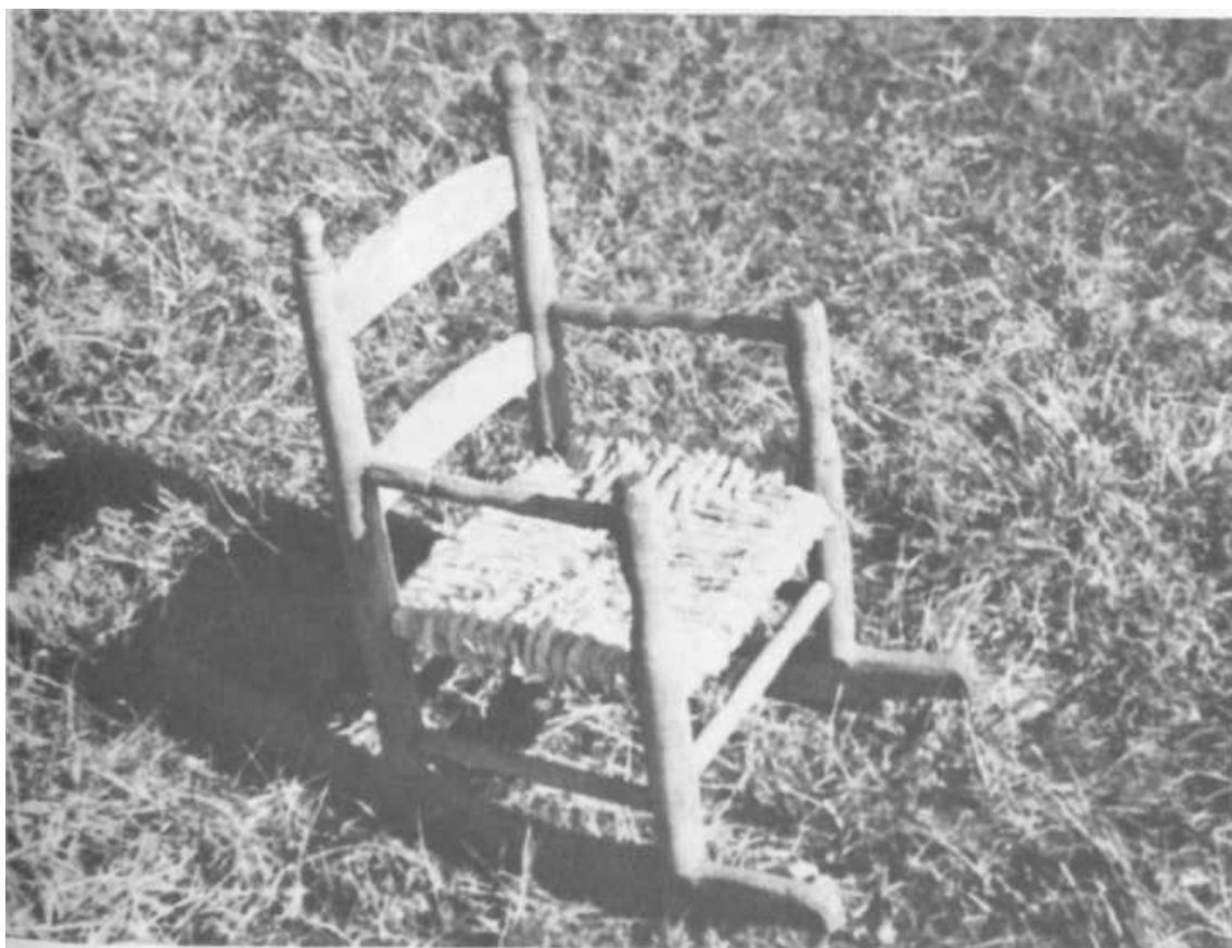
PLATE 418 The finished bottom. When completed, the pattern the shuck rope makes on the top of the chair is an "X".
