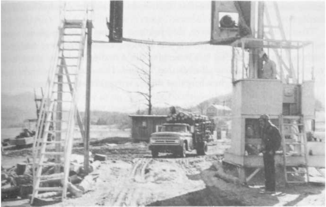
PLATE 280 A loaded truck approaches a saw that cuts the logs in half while they are still on the truck.
