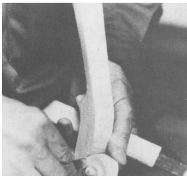
PLATES 133-134 The sides are clamped into forms as shown.
