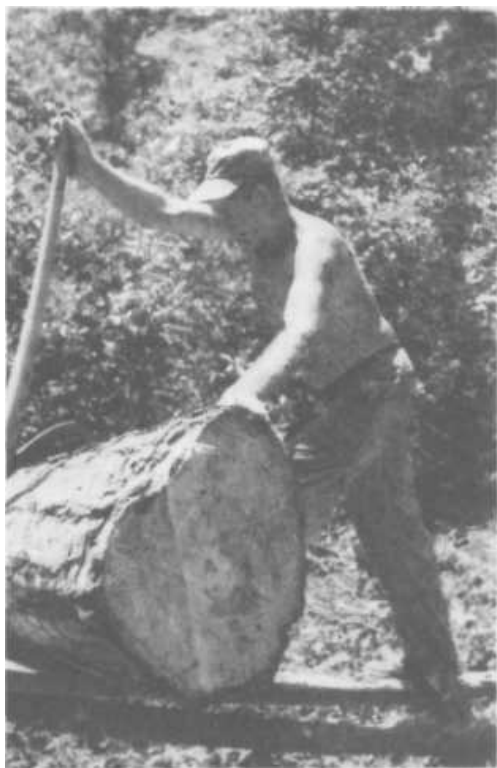
PLATE 268 At the truck, the logs are loaded by rolling them over skid poles onto the bed. They were often loaded onto wagons, years before, in the same manner.
