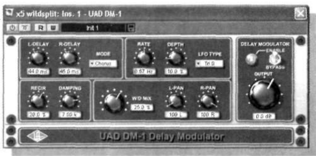
Figure 12.36. Universal Audio DM-1 Delay Modulator plug-in. (Courtesy of Universal Audio, www.uaudio.com .)
