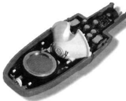
Figure 4.7. Inner detail of an AKG C3000 B condenser microphone. (Courtesy of AKG Acoustics, Inc., www.ake.com .)
