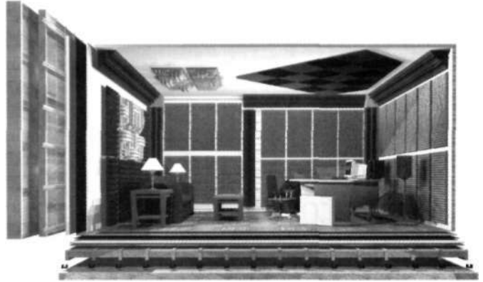
Figure 3.6. Various isolation and acoustical treatments for a recording/monitoring environment, (Courtesy of Auralex Acoustics, www.auralex.com .)
