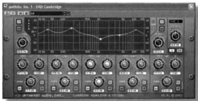
Figure 6.79. Universal Audio Cambridge EQ plug-in for the UAD-1. (Courtesy of Universal Audio, www.uaudio.com .)
