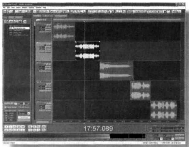
Figure 18.10. A digital audio program or burner can be used to edit, sequence, and process the final takes into a finished project. (Courtesy of Adobe Systems Inc., www.adobe.com .)
