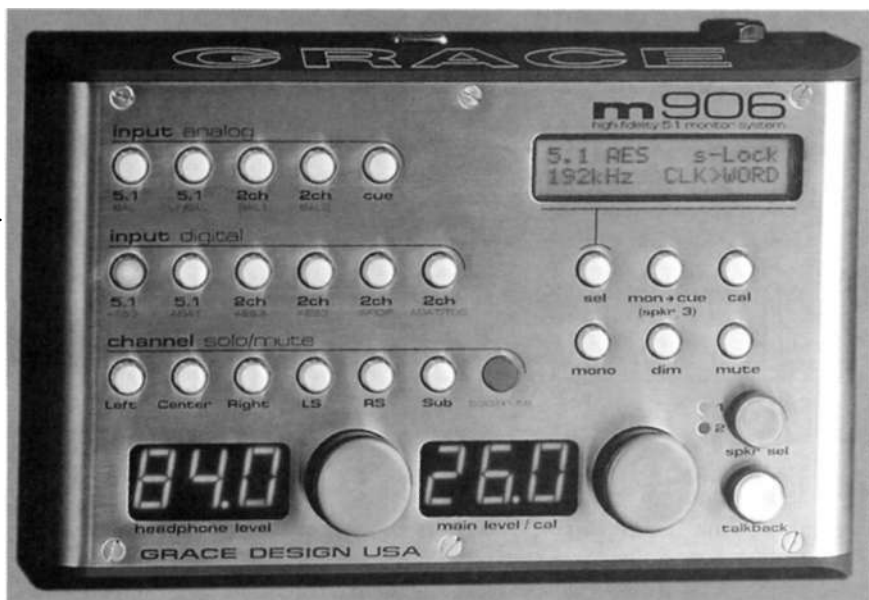
Figure 14.17. Grace Design M906 surround monitor control system. (Courtesy of Grace Design, www.gracedesign. com.)
