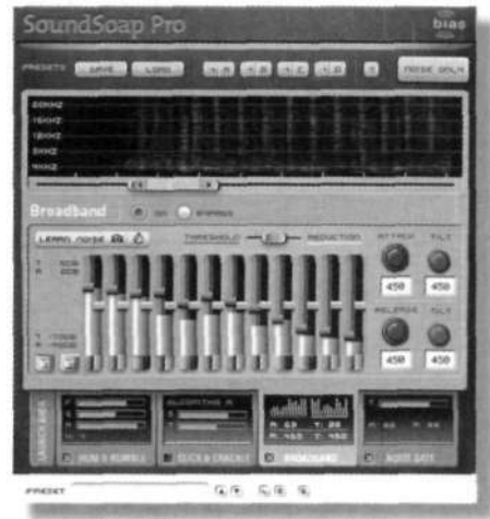
Figure 16.7. Bias Sound Soap Pro Audio restoration/cleaning plug-in. (Courtesy of Bias, Inc., www.bias-inc.com .)
