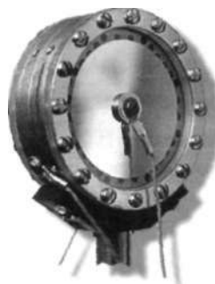
Figure 4.6. Exposed example of a condenser diaphragm. (Courtesy of ADK, www.adkmic.com ; photograph by K. Bujack.)
