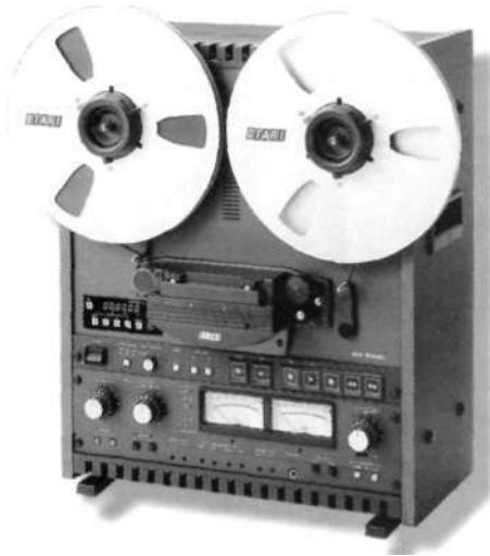
Figure 5-4. Otari MX-5050 B3 two-channel recorder. (Courtesy of Otari Corporation, www.otari.com .)
