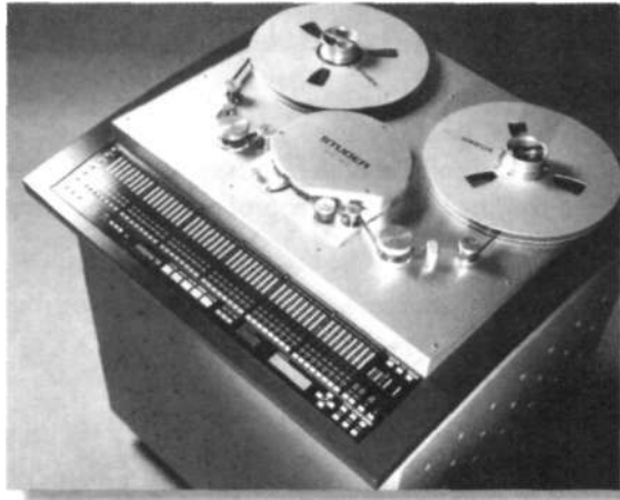
Figure 6.26. The Studer D 827 Mark II MCH 24-148-track digital audio multitrack recorder. (Courtesy of Studer Professional Audio AG, www.studer.ch .)
