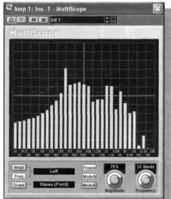
Figure 14.18. Software spectral display. (Courtesy of Steinberg Media Technologies GmbH, www.steinberg.de .)
