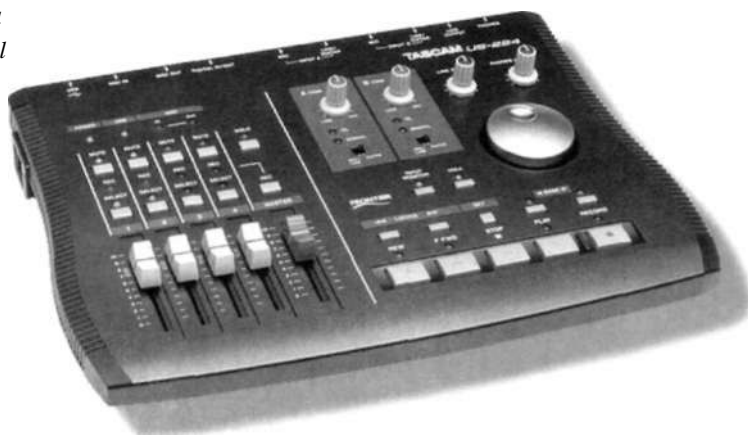
Figure 6.49. Tascam US-224 computer interface and control surface. (Courtesy of Tascam, www.tascam.com .)
