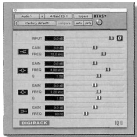
Figure 6.77. Pro Tools EQ screen. (Courtesy of Digidesign, a division of Avid Technology, Inc., www.digidesign.com .)
