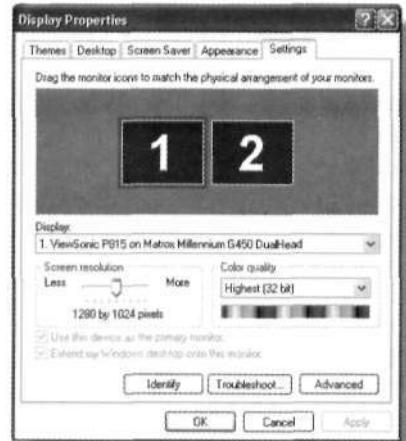
Figure 8.8. The Windows Display Properties Box is used to change screen sizing and pixel resolution.
