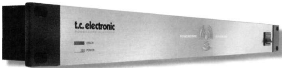
Figure 6.89. The tc electronic PowerCore FireWire rack-mountable effects accelerator, (Courtesy of tc electronic, www.tcelectronic.com .)
