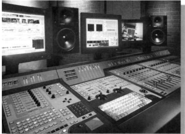
Figure 19.6. Digidesign's Control console/Pro Tools-based recording system. (Courtesy of Digidesign, a division of Avid Technology, Inc., www.digidesign.com .)
