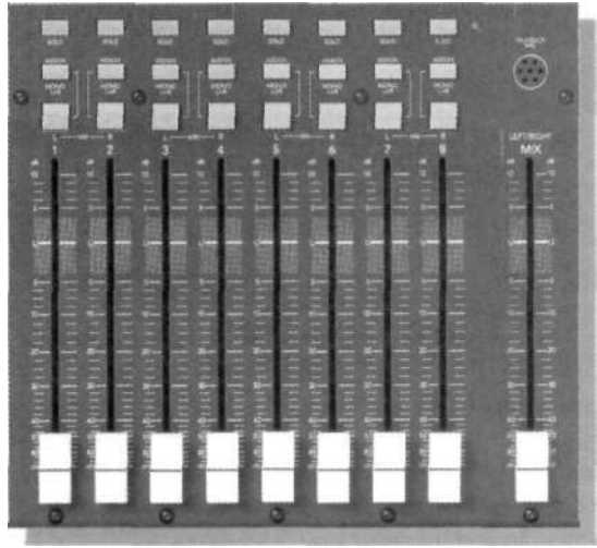
Figure 11.24. Mackie 8-bus master output fader section. (Courtesy of Loud Technologies, Inc., www.mackie.com .)
