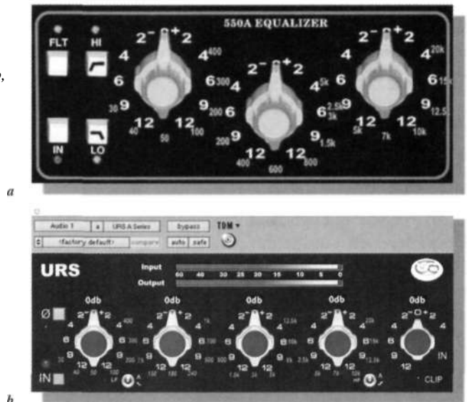
Figure 12.17. The selectable frequency equalizer: (a) venerable API 550A switchable equalizer within the 7600 outboard module (courtesy of API Audio, www.apiaudio.com ); (b) plug-in emulation of the API 550B for TDM, RTAS, and AudioSuite (courtesy of Unique Recording Software, www.ursplugins.com ).
