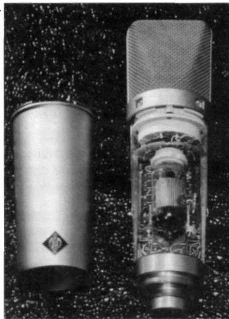
Figure 4.10. Inner detail of a Neumann U-67 condenser microphone. (Courtesy of Neumann USA, www.neumannusa.com .)
