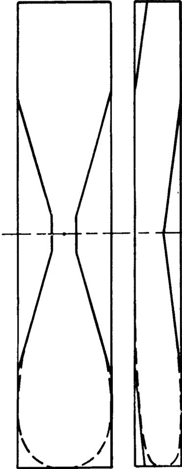
PROPELLER BLOCK —  $\frac{1}{2}$ " x  $1\frac{1}{2}$ " x 5" MED. HARD
