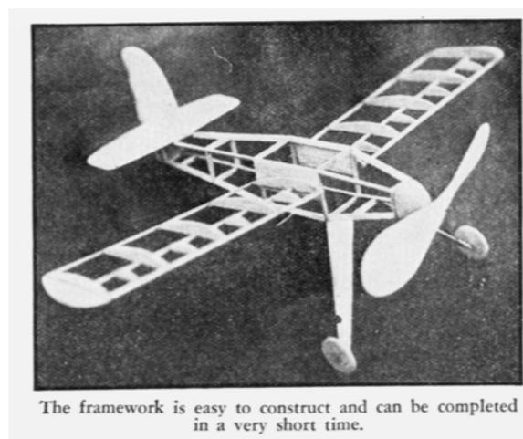
The fuselage now may be covered with a good grade of Jap tissue and doped or sprayed with water. Do not cover the side pieces, H, but cut the paper to fit around them. Cement the paper to the front, rear and bottom edges of H.
