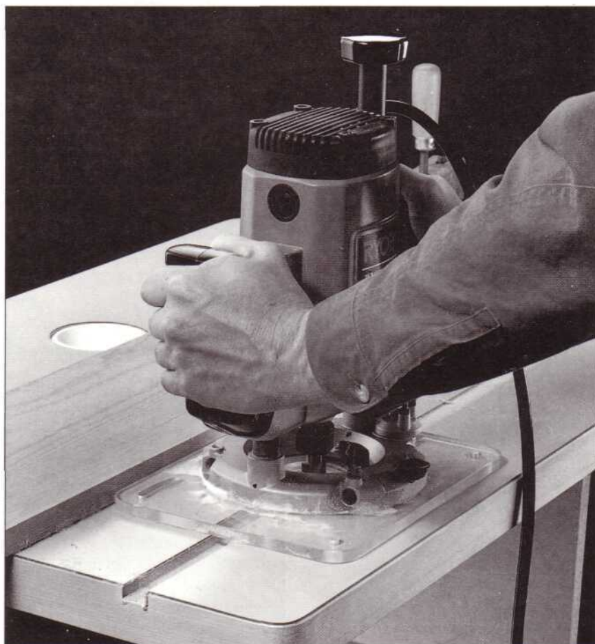
Rout a miter-gauge groove in the worktop.
