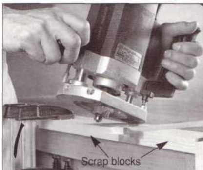
Scrap blocks (one with a rabbet) provide a straight, continuous surface for the bit's pilot to ride on.
