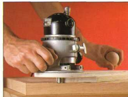
A flush-trimming jig saves you hours of planning and scraping.
