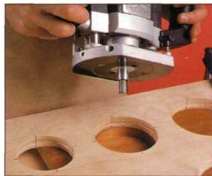
A circle template makes fast work of flat-bottom holes, such as the one above, as well as through-holes.
