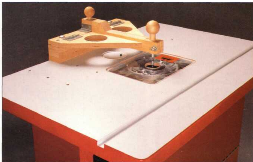
Router table fitted with a pin-routing attachment (see page 75).
