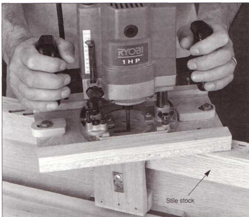
You can size the louver jig to accept any plunge router.
