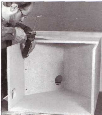
Screw the dust shoot in place, and caulk all joints for a tight seal.
