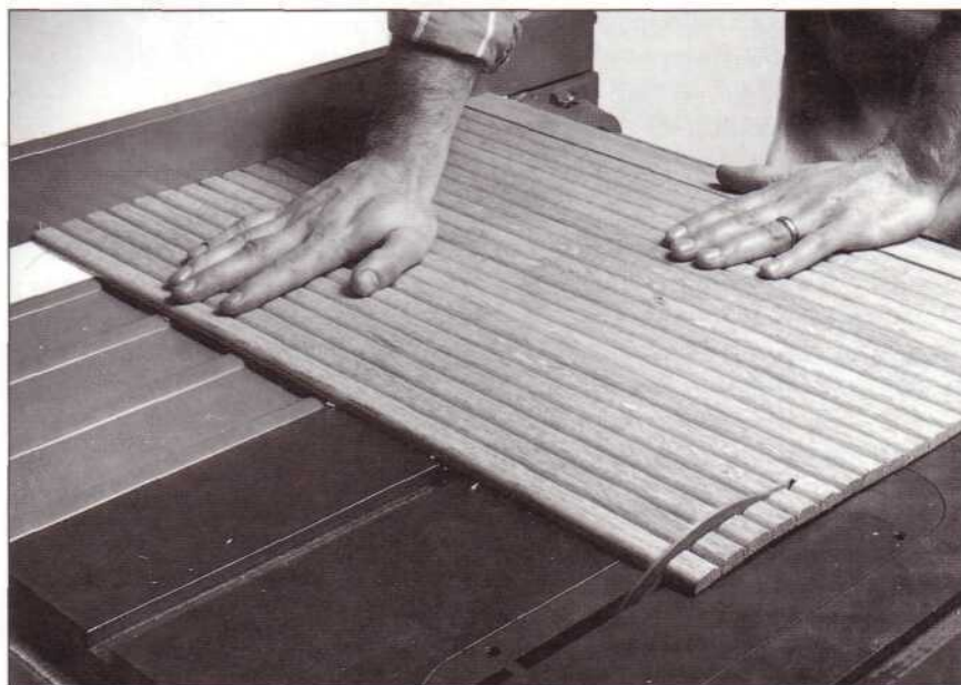
Trim the curtain with your tablesaw and stand to the side of the blade in case it ejects small slat pieces.
