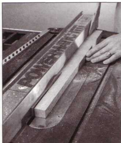
Rip both stiles from one workpiece, then rip the rails.
