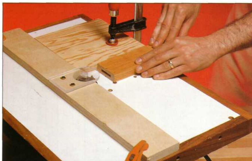
A router table can handle many of a plate joiner's jobs.
