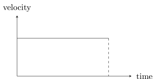
Figure 1.1: A velocity-time graph for an object moving at constant speed.
