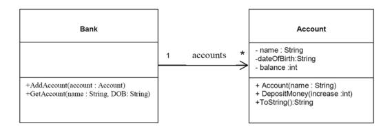
The diagram above represents the basics of a banking system (admittedly a very simplistic banking system). In this system a class is used to simulate a Bank and maintain a collection of Accounts... for the moment we will use a List to manage this collection.
