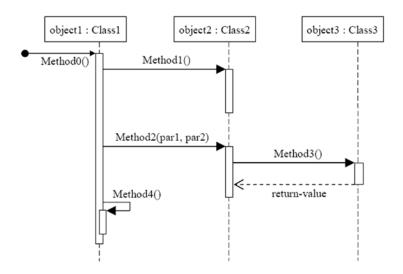
We have three objects in this scenario. Time runs from top to bottom, and the vertical dashed lines (lifelines) indicate the objects' continued existence through time.
