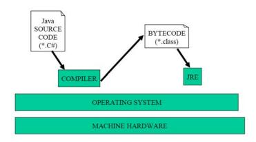
A version of the Java Runtime Environment (JRE), which incorporates a Java Virtual machine (VM), is required to execute the bytecode and the Java library packages. Thus a JRE must be present on any machine which is to run Java programs.
