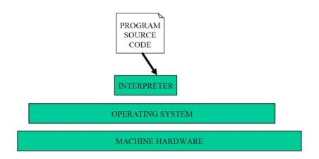
Interpreted programs can be slow but can work on any machine that has an appropriate interpreter. They do not need to be complied for different machines.
