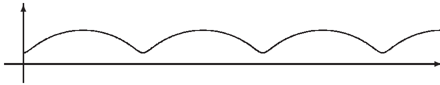
Figure 4.12: Curtate Cycloid Drawn with \writecurve similar to Fig. 4.14 ( r = 5 , a = 3 , 3.5 revs)
