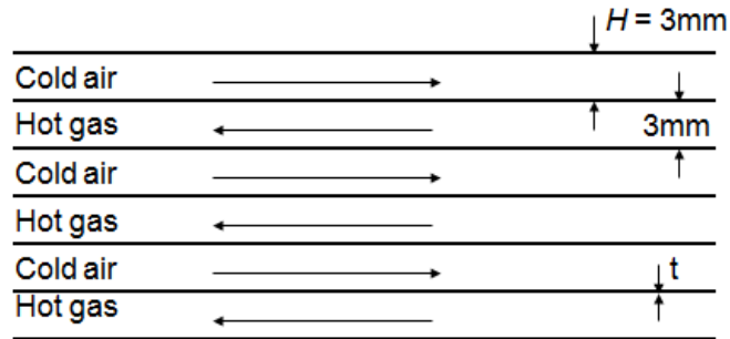
(a) Cross sectional view through part of the Heat Exchanger
