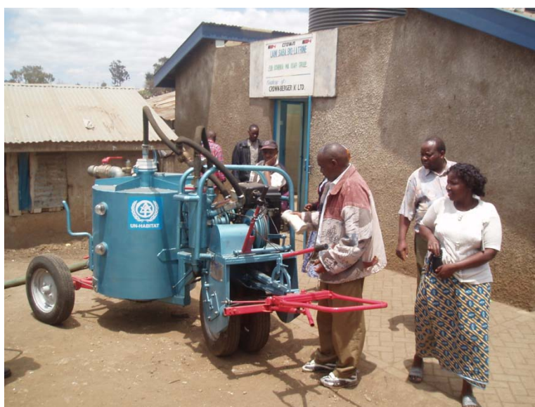
Figure 3.9: The 'Vacutug' developed by UN-Habitat.
