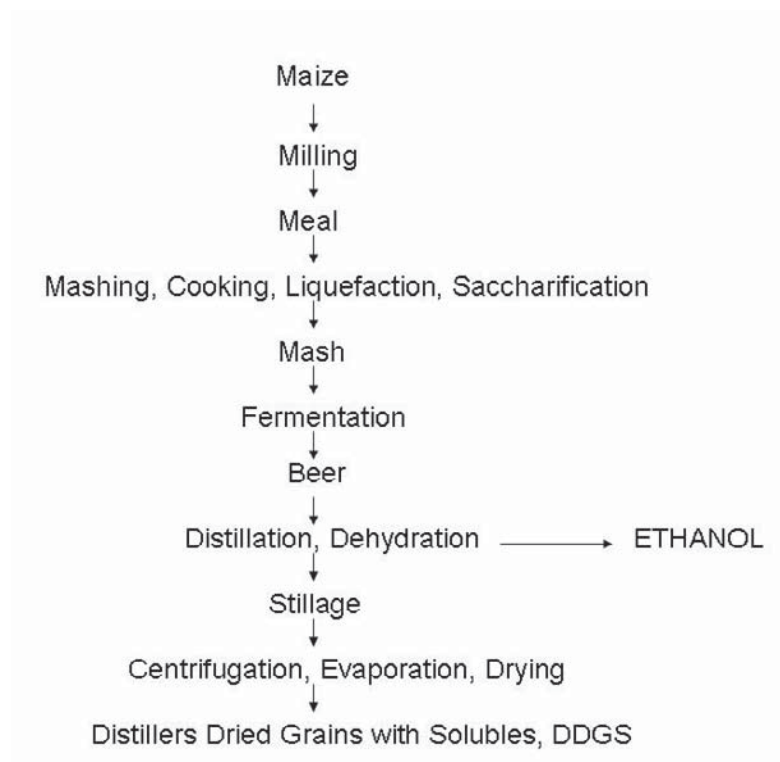
Fig 4.5 Ethanol production from maize (dry-grind process)
