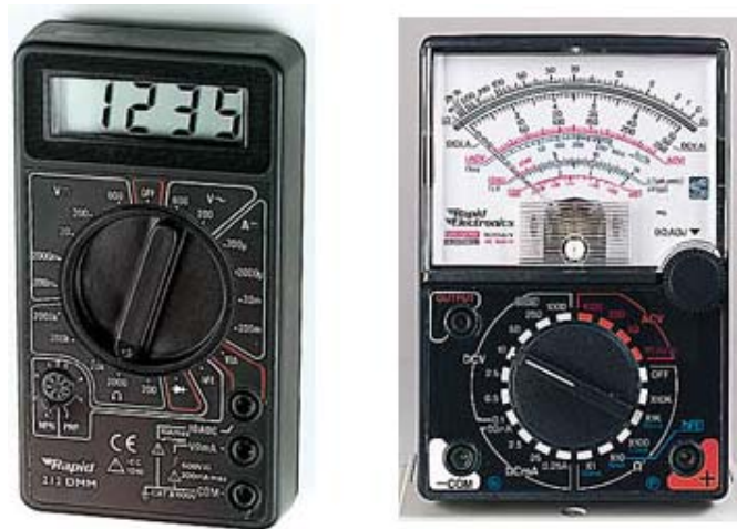
Figure 5.3 Digital and Analog Multimeters
