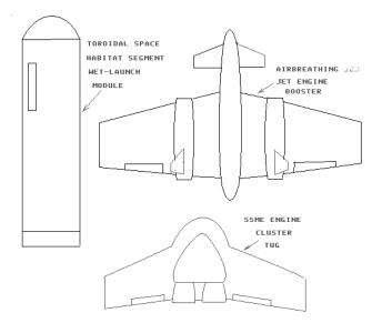
The insides of your kitchen, or whatever habitat module being launched in the moment, will be filled with fuel and oxidizer, each in its own section, separated by that inner bulkhead you mentioned."
