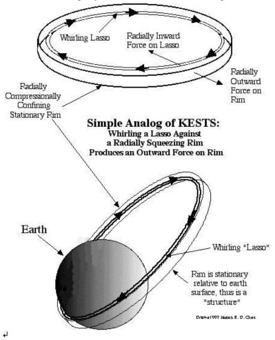
squeeze the lasso into a smaller radius than it would naturally assume, thus the lasso's centrifugal force is producing a small outward radial force on the compressing rim.
