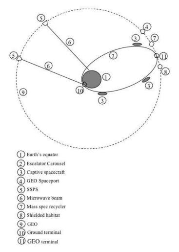
Figure 3. Overall shape of the transportation structure around the earth, along with some of its important applications it could enable construction in GEO
