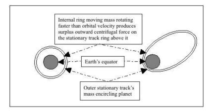
Figure 1.Visualization of imaginary experiment illustrating the upward supportive force on a stationary ring by an orbital ring sliding along beneath it faster than it's altitude's orbital velocity; then transferring to an elliptical structure.
