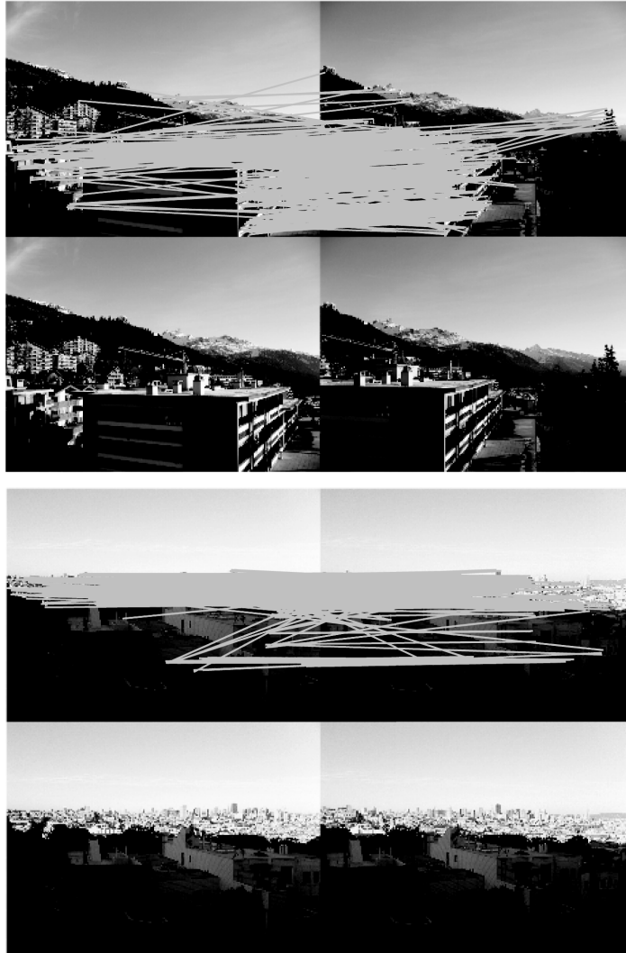
Figure 2-2. Example of matches resulting from applying normalized cross-correlation to patches around Harris corner points.
