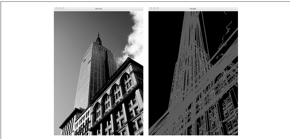
Figure 10-10. An example of detecting lines using a Hough transform. The left image is the source in grayscale. The right image shows an edge map with detected lines.
