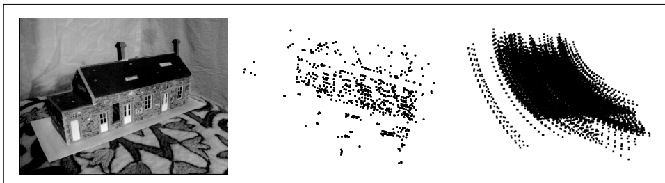
Figure 4-2. An example of projecting 3D points: sample image (left); projected points into a view (middle); trajectory of projected points under camera rotation (right). Data from the Oxford “Model House” dataset.
