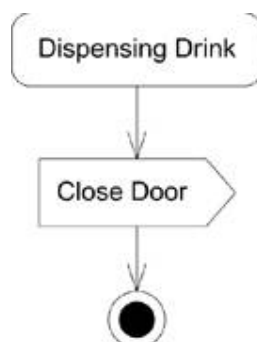
Figure 8-14. Transition-oriented view of a signal being dispatched
