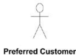
Figure 7-4. An actor using the stick figure representation
