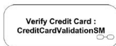
Figure 8-11. A submachine state showing the composite icon
