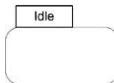
Figure 8-4. A state with its name in a tab
