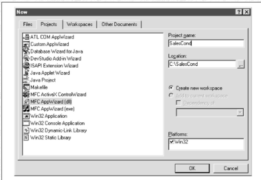
Figure 11- 5. Selecting the type of MFC DLL
