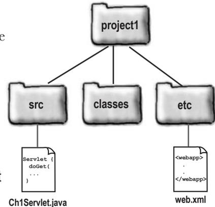
**2** Write a servlet named Ch1Servlet.java and put it in the src directory (to keep this example simple, we aren't putting the servlet in a package, but after this, all other servlet examples in the book will be in packages).
