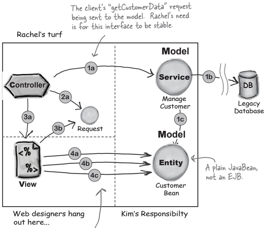
The JSP uses EL to access the Customer Bean properties. The web designer's need is for this interface to be stable.
