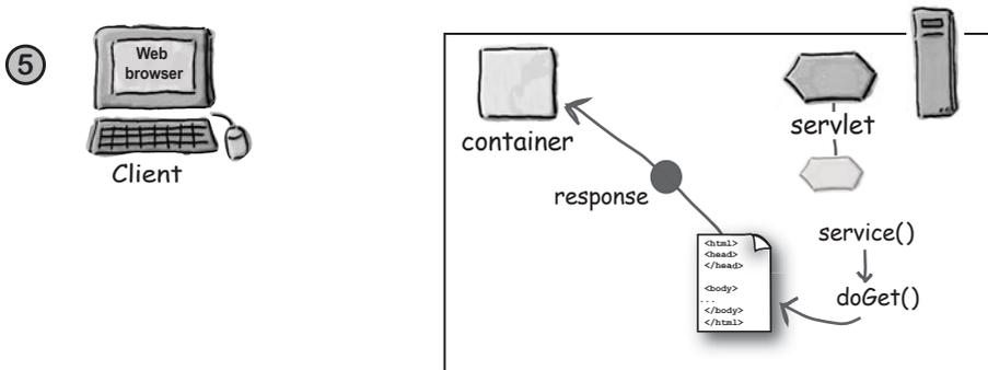
The `doGet()` method generates the dynamic page and stuffs the page into the response object. Remember, the container still has a reference to the response object!
