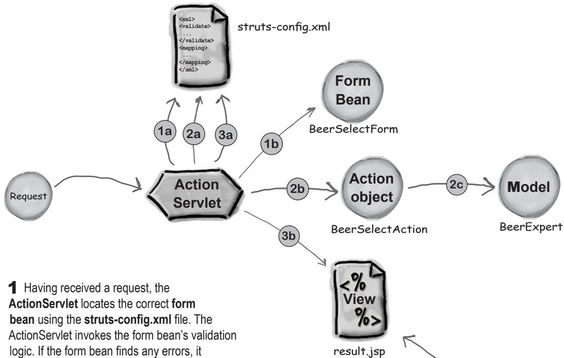
**1** Having received a request, the **ActionServlet** locates the correct **form bean** using the **struts-config.xml** file. The ActionServlet invokes the form bean's validation logic. If the form bean finds any errors, it populates an **ActionErrors** object.
