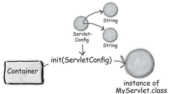
Since the Container reads the servlet init parameters only *once*, you *still* can't change your email address during the life of the servlet. So this is a dumb solution.
