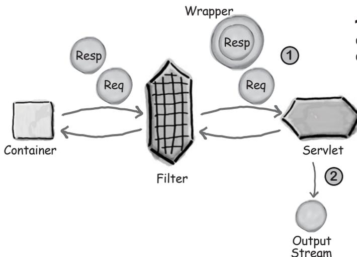
**1** The filter passes the request object and a **custom** response object to the servlet.
