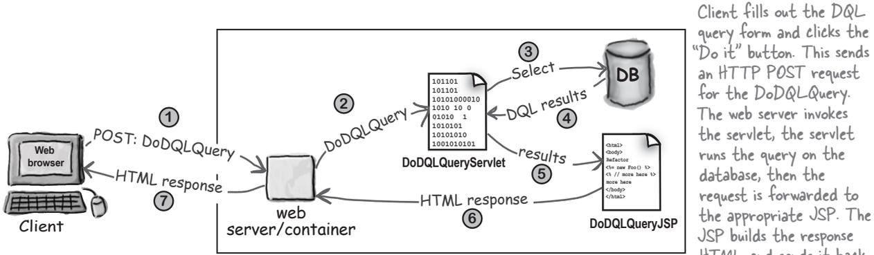
Client fills out the DQL query form and clicks the "Do it" button. This sends an HTTP POST request for the `DoDQLQuery`. The web server invokes the servlet, the servlet runs the query on the database, then the request is forwarded to the appropriate JSP. The JSP builds the response HTML and sends it back.
