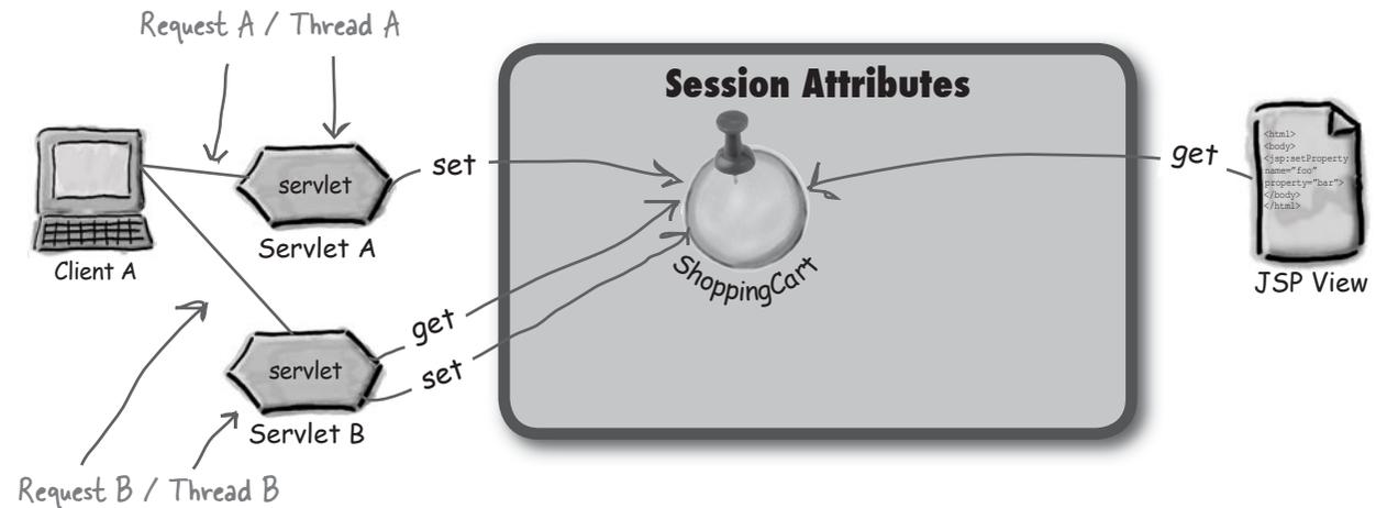
Even though both servlets can access the Session attributes in separate threads, each thread is a separate request. So it looks safe.
