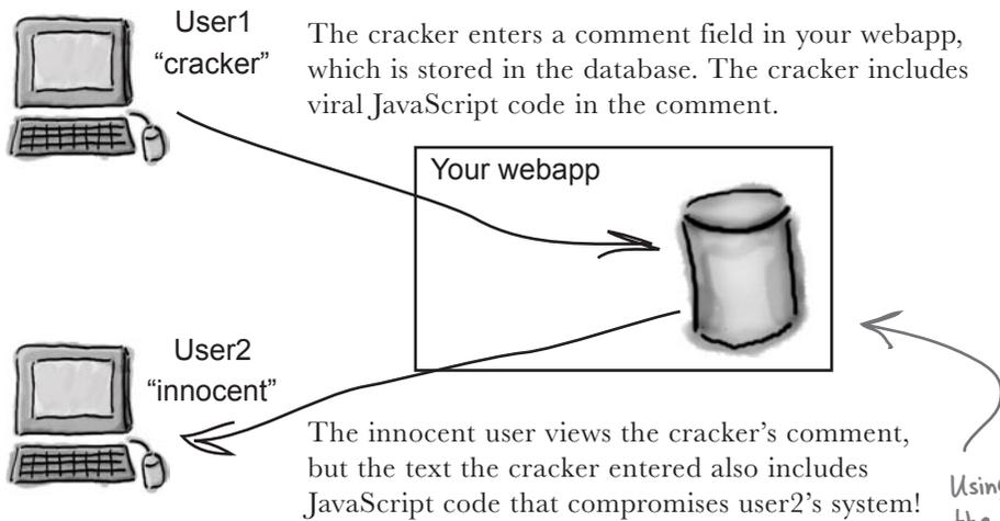
*Using the c:out tag to render the text of users prevents cross-site hacking of this form by displaying the <script> tags and the JS code in user2's web browser. This prevents the JS code from being interpreted by the browser, foils the attack from user1.*
