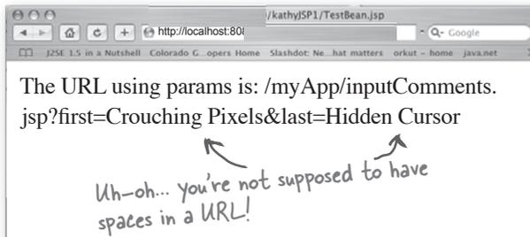
Yikes! Query string parameters have to be encoded... spaces, for example, must be replaced with a plus "+" sign.
