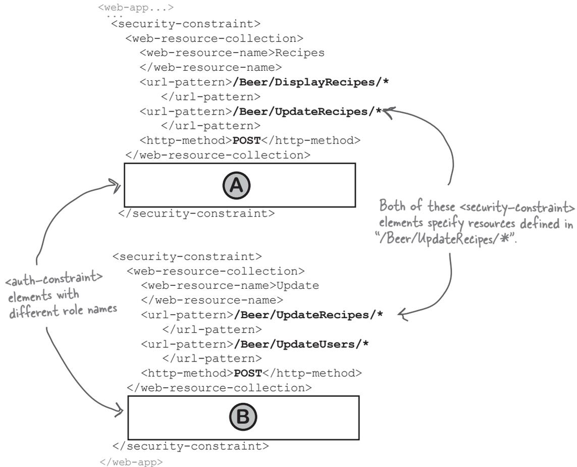
**How should the container handle authorization when the same resource is used by more than one `<security-constraint>`?**
