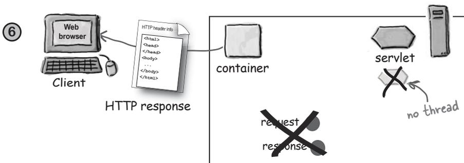
The thread completes, the container converts the response object into an HTTP response, sends it back to the client, then deletes the request and response objects.
