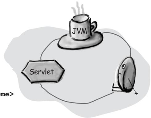
A **LOCAL** bean means the client (in this case, a servlet) and the bean must be running in the same JVM.
