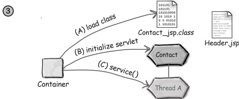
The Container compiles the translated source file into a servlet class. It's just like any other servlet at this point. The generated servlet class file is loaded into the Container's JVM and is initialized. Next, the Container allocates a thread for the request and calls the JSP's \_jspService() method.
