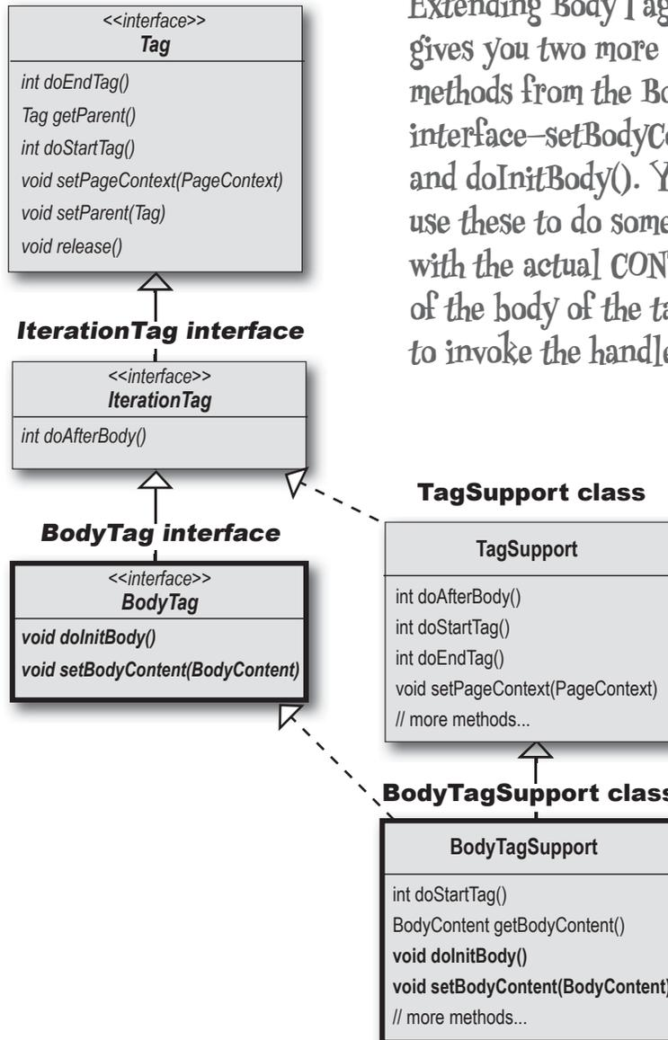
Extending **BodyTagSupport** gives you two more lifecycle methods from the **BodyTag** interface—`setBodyContent()` and `doInitBody()`. You can use these to do something with the actual CONTENTS of the body of the tag used to invoke the handler.
