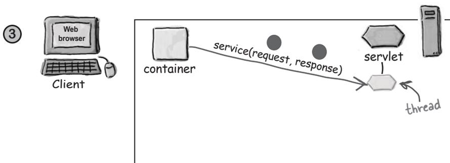
The Container finds the correct servlet based on the URL in the request, creates or allocates a thread for that request, and calls the servlet's `service()` method, passing the request and response objects as arguments.
