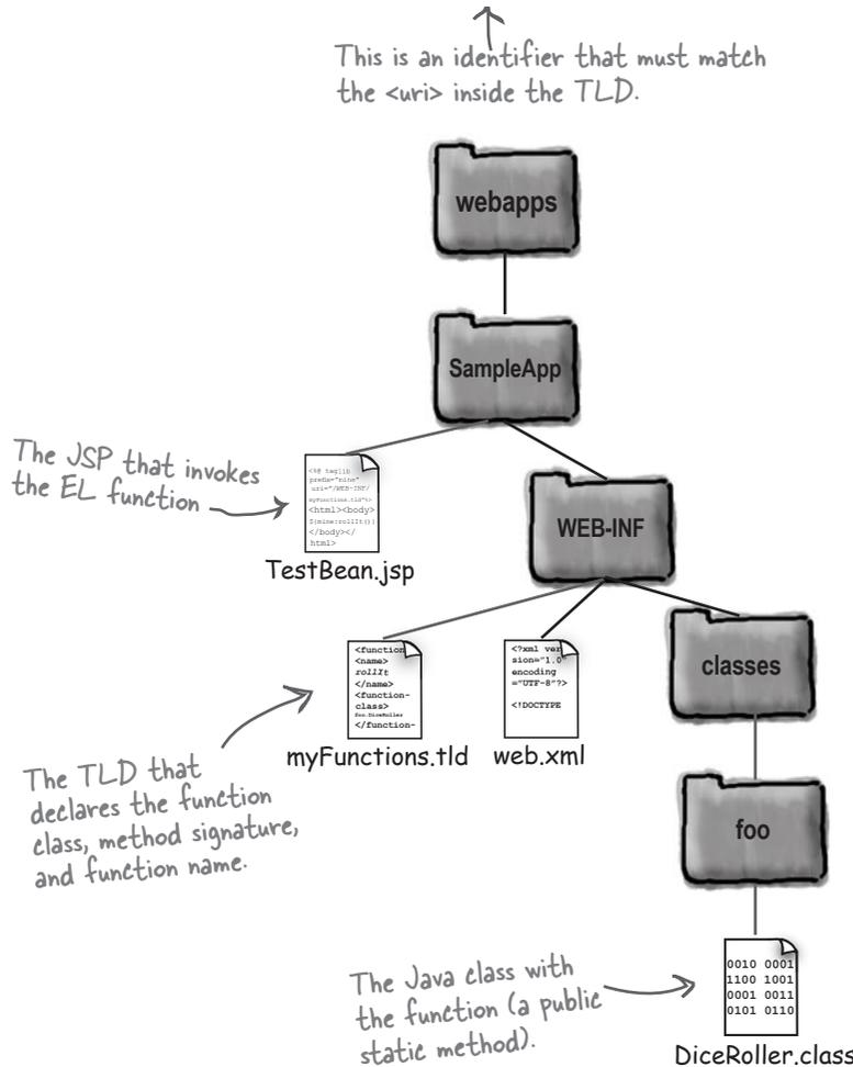
The class with the function (the public static method) must be available to the web app just like servlet, bean, and listener classes. That means somewhere in WEB-INF/classes...
