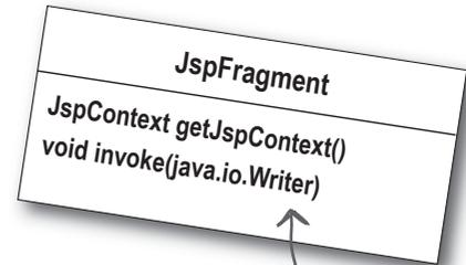
The `invoke()` method takes a *Writer*... pass null to send the body to the response output, or a *Writer* if you want direct access to the actual body contents.
