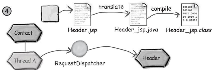
The Contact servlet hits the method that does the dynamic include, and something vendor-specific happens! All we care about is that the response generated by the Header servlet is combined with the response from the Contact servlet (at the appropriate place). (NOT SHOWN: at some point the Header.jsp is translated and compiled, then the generated servlet class is loaded and initialized.)
