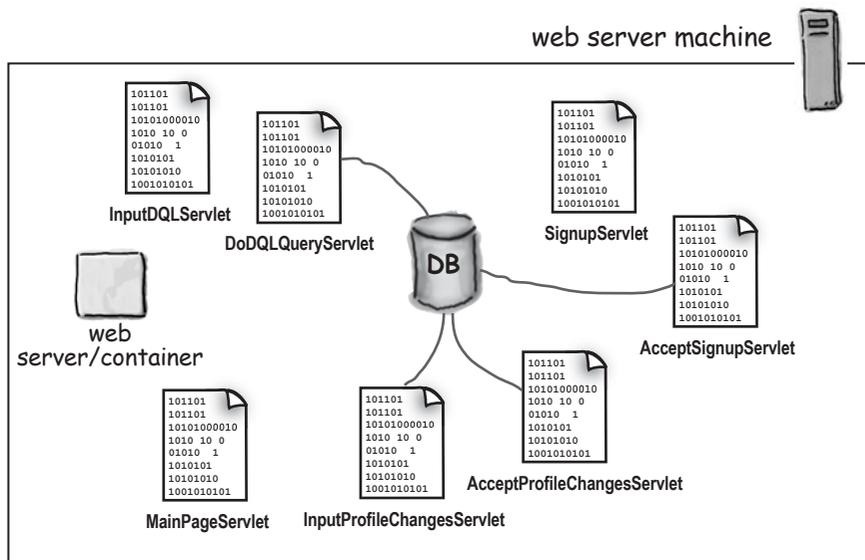
The servlet does whatever it needs to do to process the request (like insert or search the database) and returns the HTML page in the HTTP response.
