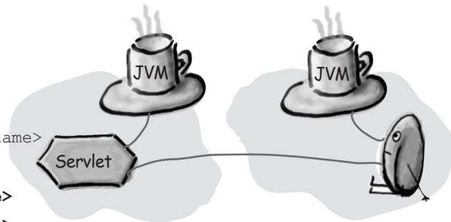
A **REMOTE** bean means the client (in this case, a servlet) and the bean can be running in different JVMs (possibly on different physical machines as well).
