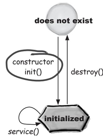
The `init()` runs only once in a servlet's life, so don't blow it! And don't try to do things too soon... the constructor is too early to do servlet-specific things.
