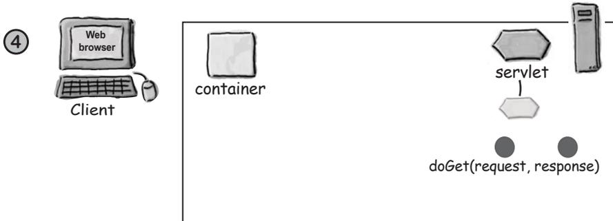
The service() method figures out which servlet method to call based on the HTTP Method (GET, POST, etc.) sent by the client.
