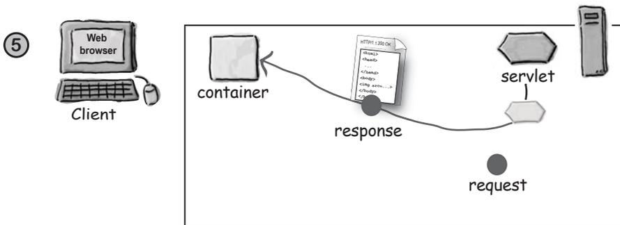
The servlet uses the response object to write out the response to the client. The response goes back through the Container.
