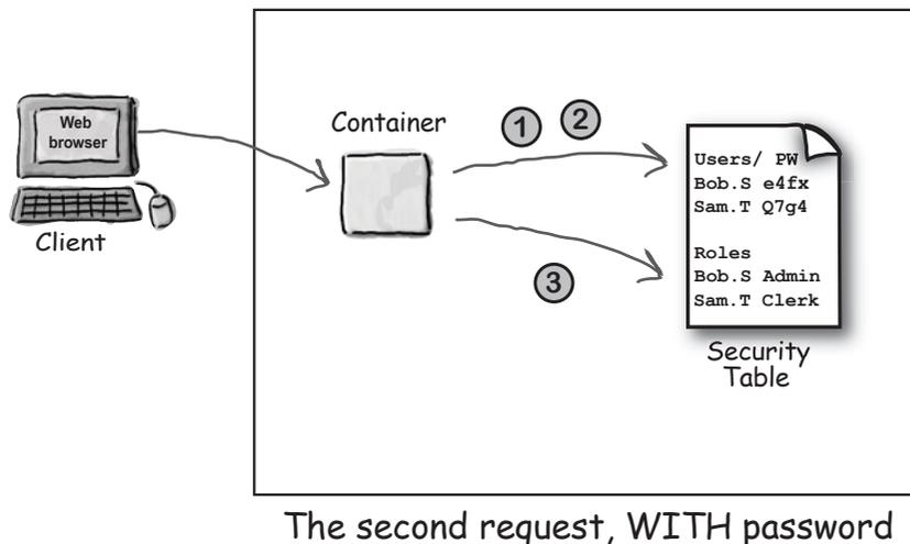
**1** When the Container receives a request with a username and password, it checks the URL in the security table.
