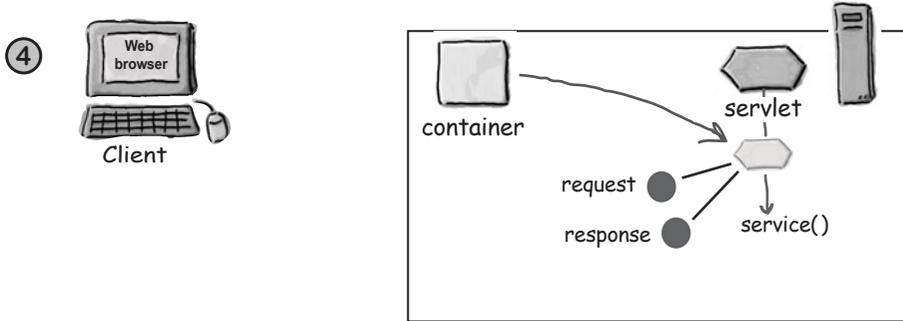
The container calls the servlet's `service()` method. Depending on the type of request, the `service()` method calls either the `doGet()` or `doPost()` method.
