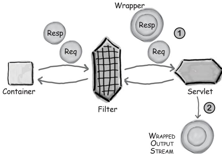
**1** The filter passes the request object and a **custom** response object to the servlet. The custom response has a special **getOutputStream** method.
