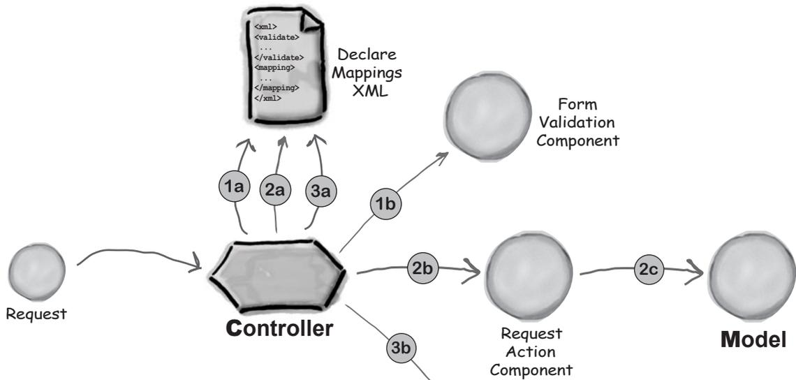
**1** Having received a request, the **Controller** locates the correct **Form Validation Component** in the **Declarations XML** file. The Controller invokes the Form validator, sending it the request. If the validator finds any errors, it tells the controller which view to return.
