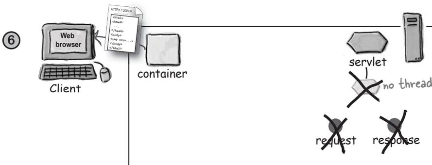
The service() method completes, so the thread either dies or returns to a Container-managed thread pool. The request and response object references fall out of scope, so these objects are toast (ready for garbage collection).
