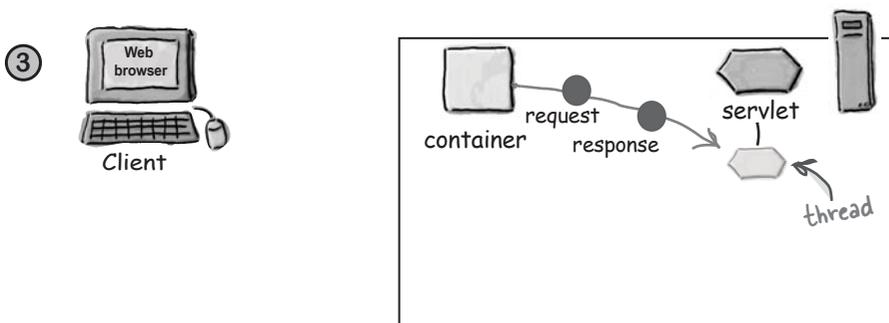
The container finds the correct servlet based on the URL in the request, creates or allocates a thread for that request, and passes the request and response objects to the servlet thread.
