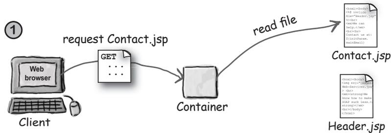
The client makes a request for Contact.jsp, which has not been translated. The Container reads the Contact.jsp page to start the translation process.
