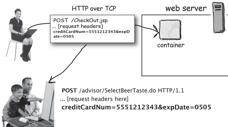
The Bad Eavesdropper gets a copy of the HTTP request that contains the client’s credit card info. The data isn’t protected, so it comes over in the body of the POST in a nice readable form. *The Eavesdropper is happy.*
