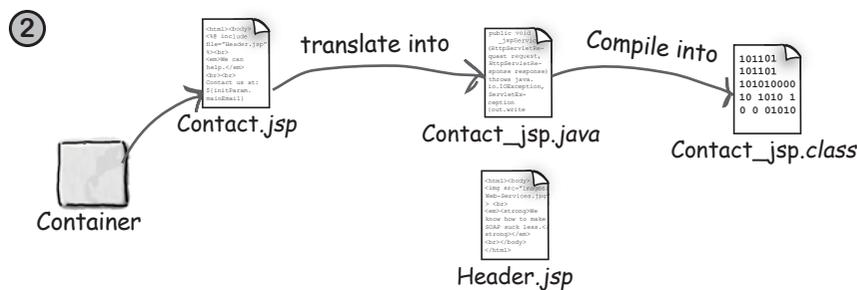
The container sees the include standard action, and uses that to insert a method call in the generated servlet code that—at runtime—will dynamically combine the response from Header.jsp into the response from Contact.jsp. The Container generates servlets for both JSP files. (This is not dictated by the spec, so we're showing only an example of how it *could* work.)
