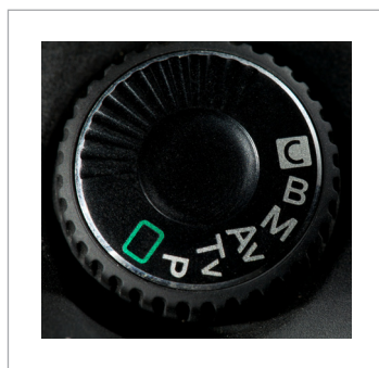
Fig 5-1. a typical camera dial with the “green box” that indicates automatic mode.
