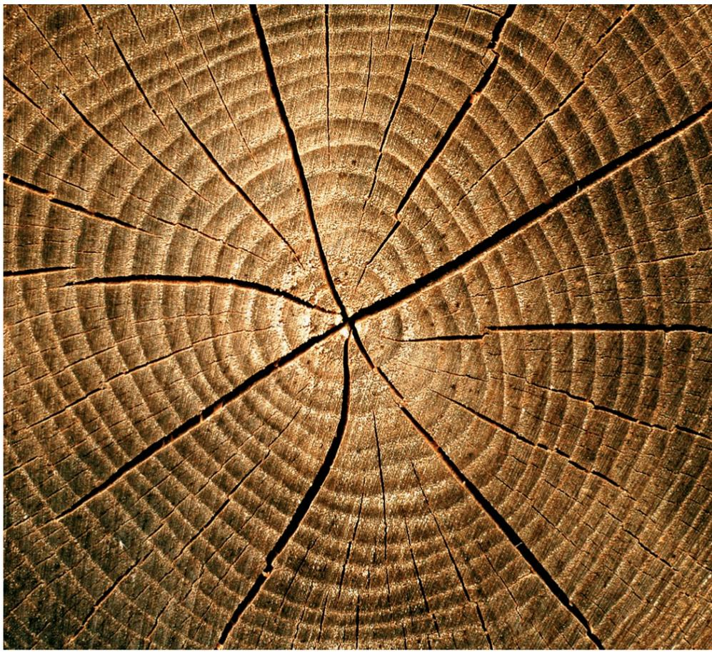
**Up to half the weight** of a freshly cut tree may be water, and as this water evaporates out the wood shrinks, cracks and warps. Controlled drying of wood can minimize these problems and produce a larger number of solid, furniture-grade boards.
