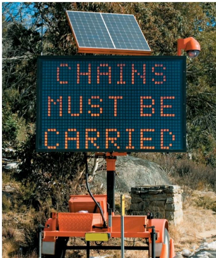
**Solar power road signs** are a common sight on highways. The light is plugged into a battery, which stores power produced by the PV panel. A charge controller keeps the battery from overcharging.
