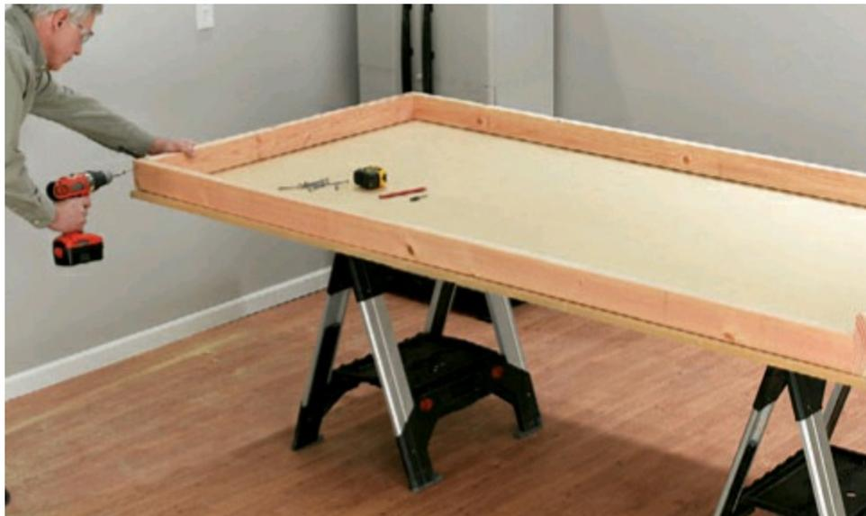
**1** The frame that houses this solar water heater is constructed from  $2 \times 4$  and  $2 \times 6$  dimensional lumber. Cut the pieces of the frame to length, then join them with  $2\text{-}1/2$ " deck screws driven into pilot holes.
