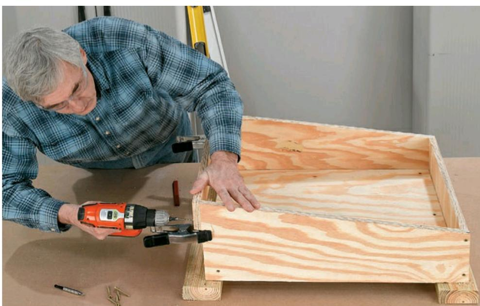
**3** Screw the **first layer** of front and side pieces to the base and to each other, then add the back piece. Pre-drill the screws with a countersink bit.
