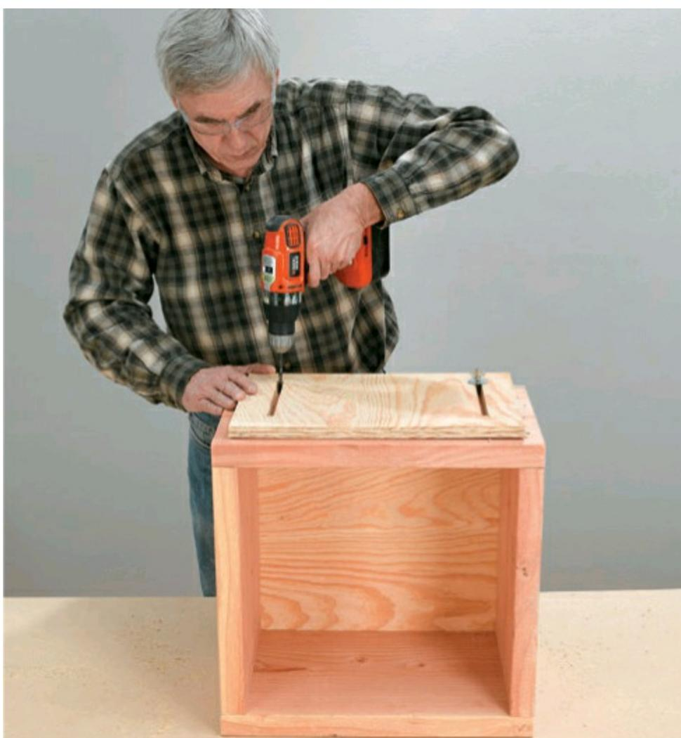
**8** Screw the base and the plywood bottom together. Set the adjustable leg against one side of the base, then drill guide holes and install the hanger bolts so they will align with the slots. The centers of the bolts should be at the same height: roughly 2-1/2" up from the bottom of the box. Use large fender washers and wingnuts to lock the adjustable leg in position.
