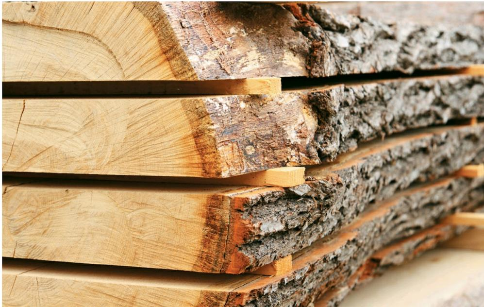
**Fresh-cut hardwood** from your own wood lot, like this old-growth oak, has a special appeal. Drying these planks in a solar kiln helps bring out the character of the wood, without drying it so quickly that it cracks.
