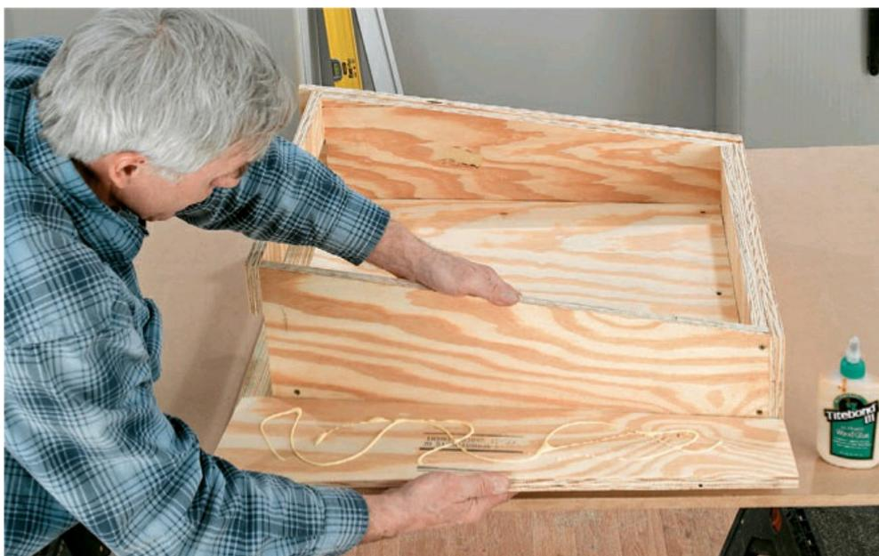
**4** **Glue and screw** the remaining front and side pieces on, using clamps to hold them together as you pre-drill and screw. Use 1/4" screws to laminate the pieces together and 2" screws to join the corners.
