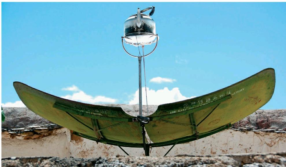
**It looks like some strange metal bird**, but it's actually a solar cooker boiling water for tea. The panel is shaped so that all the reflected sunlight is focused on the base of the pot.
