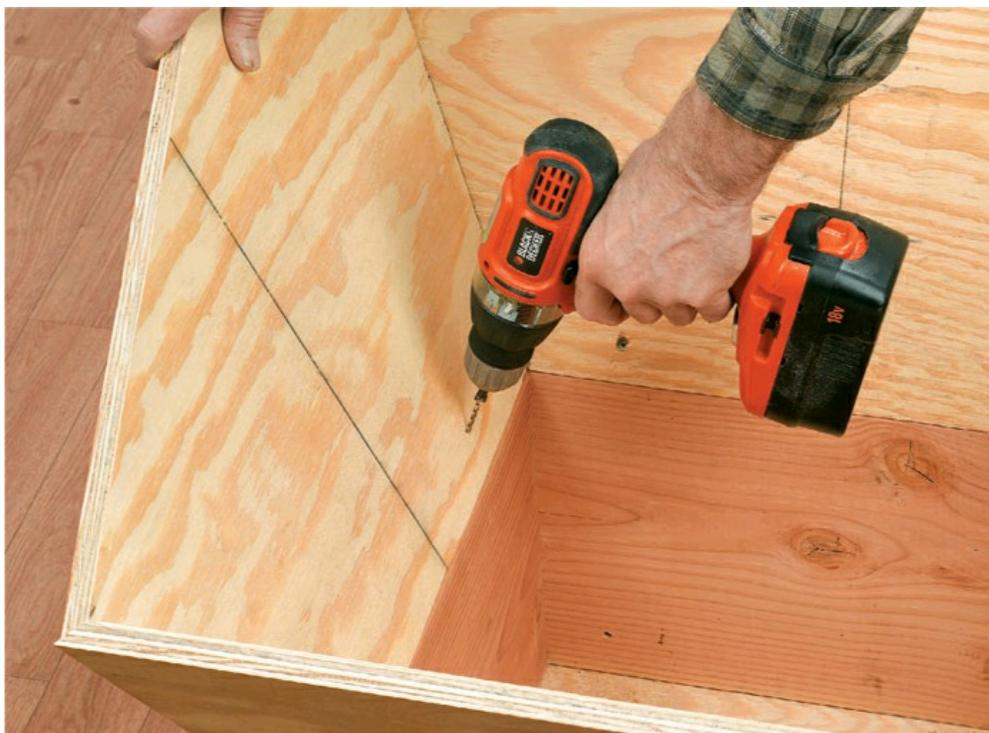
**9** Fasten the reflector to the base with countersunk 2-1/2" screws. Angle the drill bit slightly as you drill to avoid breaking the plywood edge. Use two screws per side.
