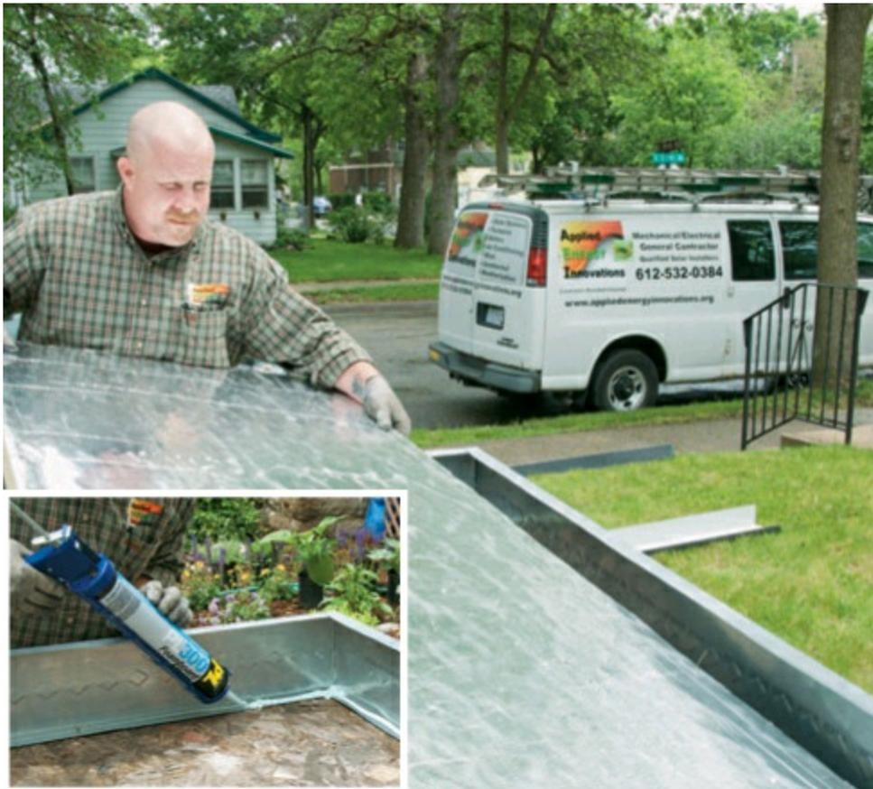
**5 Apply high-temperature silicone** to the bottom flanges of the box (inset). Fit the 1" foil-faced foam into the back of the frame, then close up the box and secure the open corner. Cut 5"-wide strips of foam insulation to the length and width of the panel. Place a thick bead of silicone around the outside perimeter of the unit. Insert the strips into the silicone and press tightly against the sides of the panel to hold the backing firmly in place. The foil should be facing into the box.
