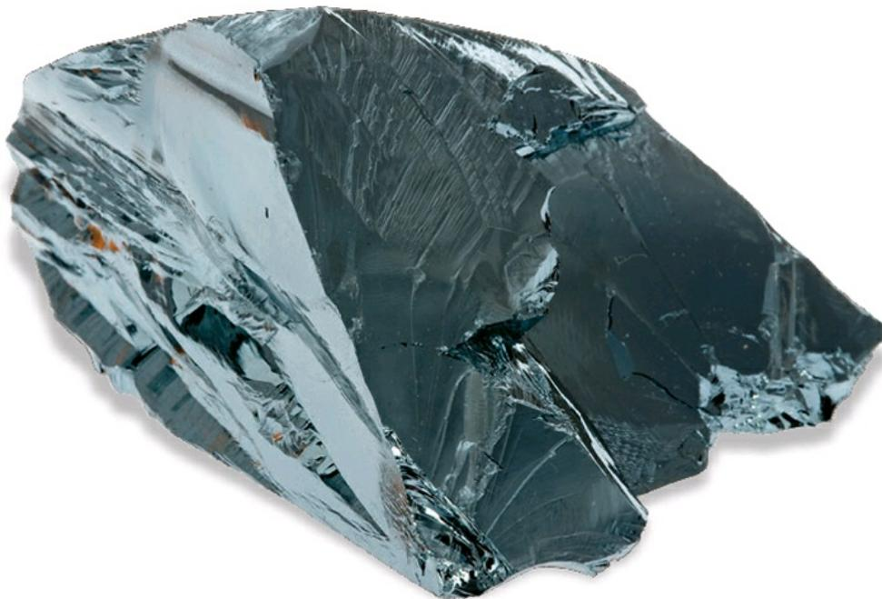
**Polycrystalline silicon** is used in almost all photovoltaic panels to convert photons of light into electricity.
