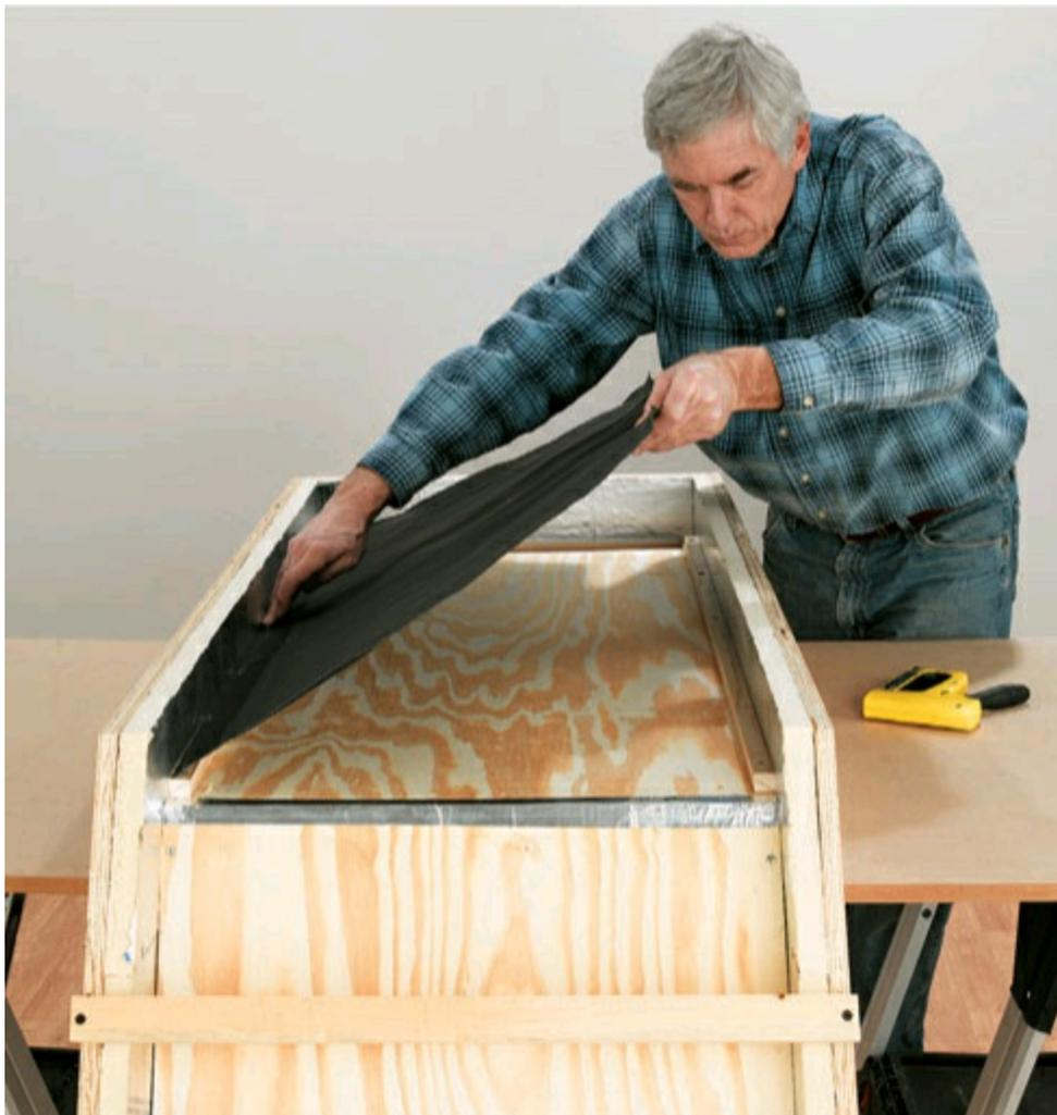
**8** Cut two 3/4" nailers an inch shorter than the plywood divider, then fasten them to the plywood and the 1 × 3 to create an air channel above and below the heat-absorbing aluminum. Cut the aluminum to fit across the box, then attach it to the nailers with stainless-steel staples or 1/2" sheet-metal screws. (Note: We used a thick, pre-painted aluminum sheet that's available online. If you use aluminum coil stock, paint it black after installing it. See Resources on p. 152.)
