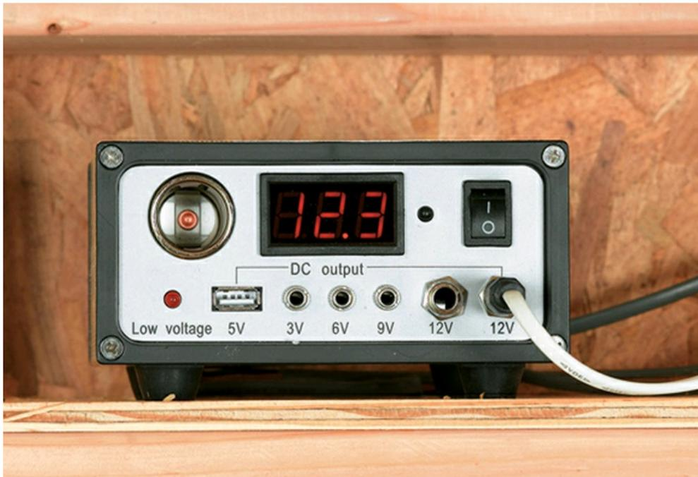
**10** This kit includes two DC lights. To install them (or other DC appliances), just plug the cord in to the proper port (or adapter) and turn the power on. Hang the 12-volt light fixtures from the rafters and then staple the cords to keep them secure and out of the way. Make sure to leave enough cord that the plug end is easy to insert and remove from the port. You'll plug and unplug the lights to turn them on and off.
