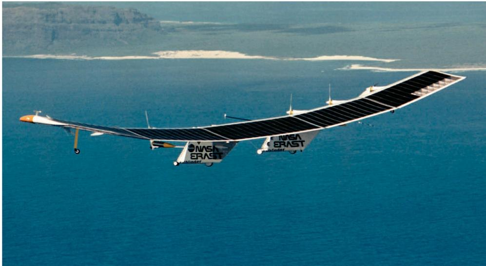
**Remotely piloted, solar-powered** aircraft are being developed by NASA as part of research into airplanes of the future. Here a prototype is being put to use photographing coastal ecosystems in Hawaii.
