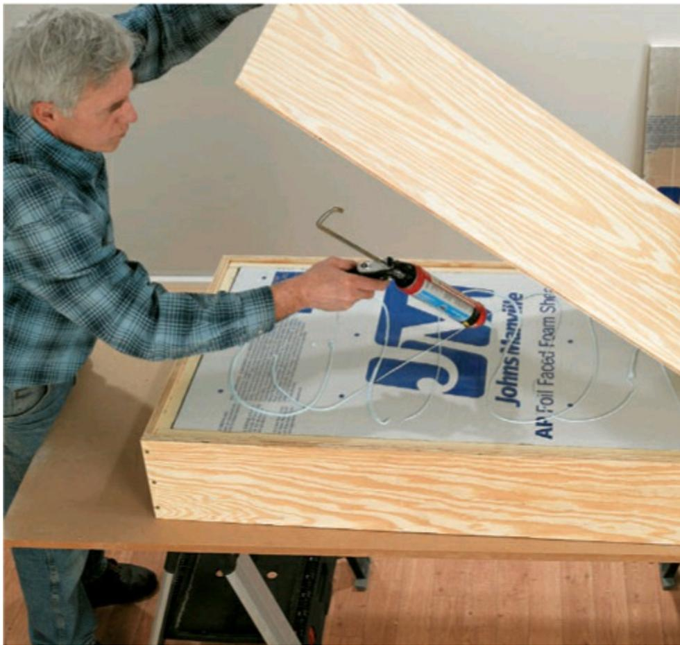
**7** Turn the box over, then add the 1" insulation to the bottom of the box, then cover it with the 1/4" plywood. Glue the plywood to the insulation and screw it to the 1 × 3 nailer with 2-1/4" screws.
