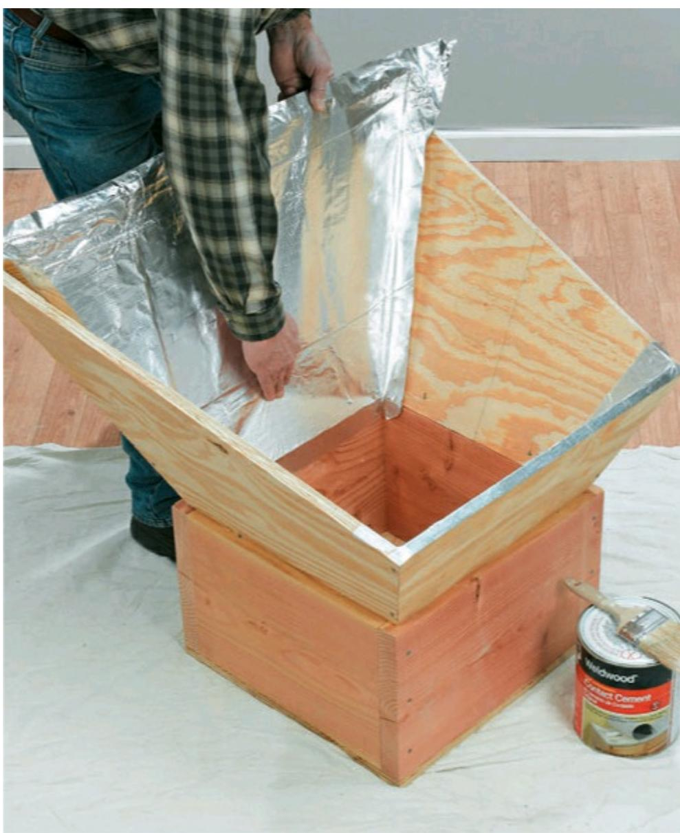
**1 Glue the reflective sheeting** inside the base and reflector, overlapping the corners so all bare wood is covered. Use contact cement or silicone caulk to adhere solar foil, and staple the edges to reinforce the glue; use diluted white glue with a paint brush instead of contact cement if you're using aluminum foil. Pull or smooth out the reflective material as much as possible; the smoother the surface is, the better it will reflect light.
