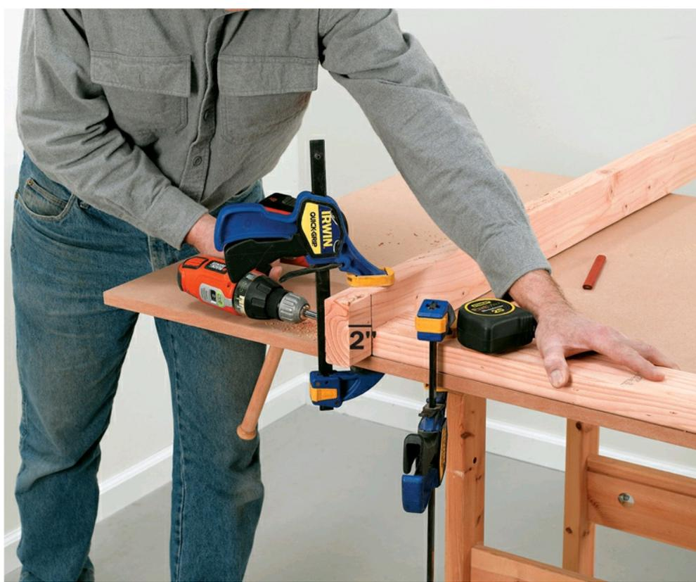
**2** Assemble the remaining sides, but instead of aligning the horizontal studs with the edge, fasten them 2" in from the edges. Place the third stud in the center.
