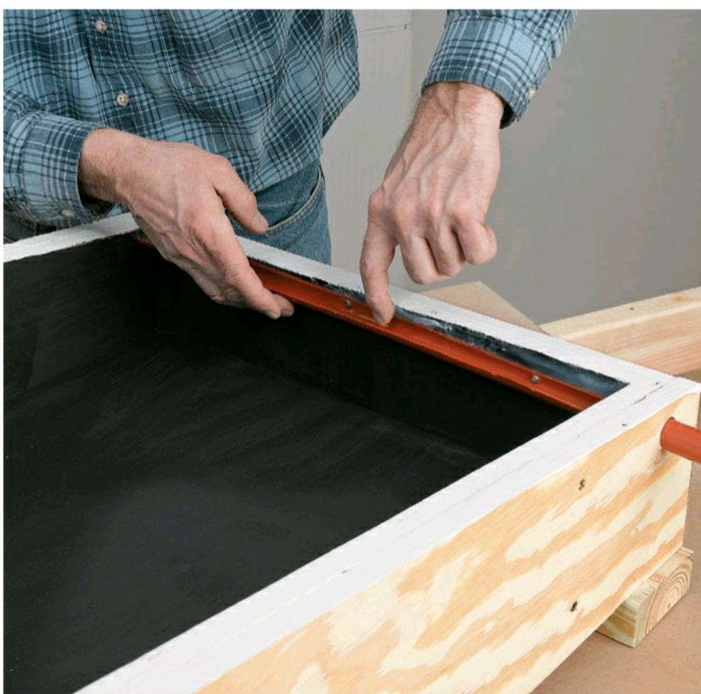
**11** Wipe a thick bead of silicone caulk along the top edge of the PEX to seal it against the plywood.
