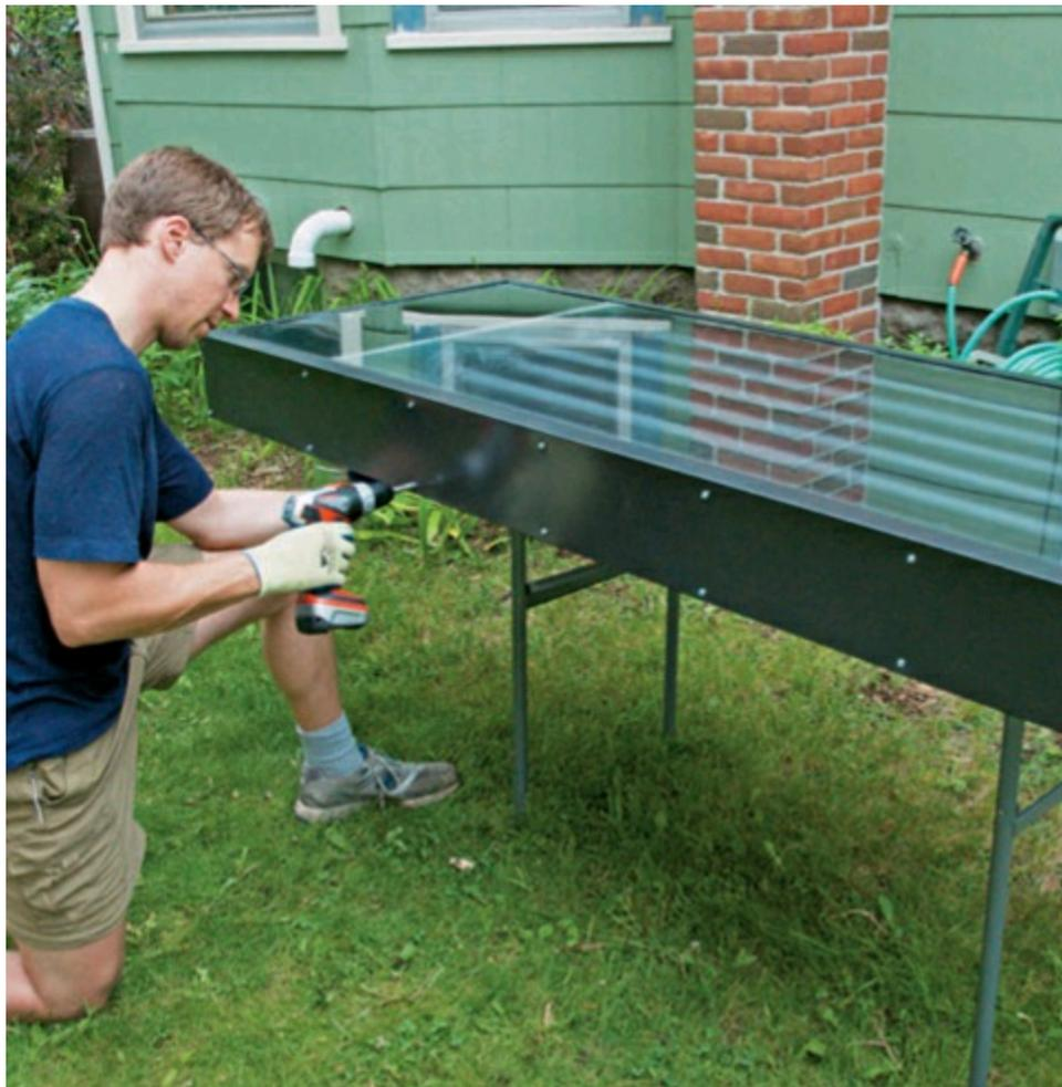
**13 Attach the casing.** Work with a local metal shop to bend metal flashing that will wrap your panel box. Attach it around the perimeter of the panel with sheet-metal screws with rubber washer heads.
