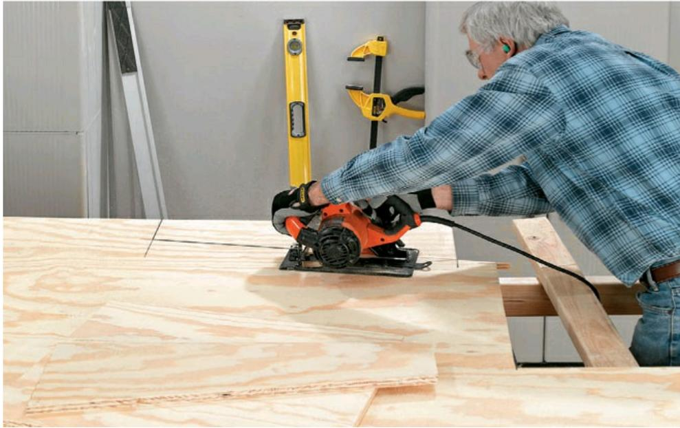
**1** Mark and cut the plywood pieces according to the cutting list, p. 133. Cut the angled end pieces with a circular saw or tablesaw set to a 9° angle.
