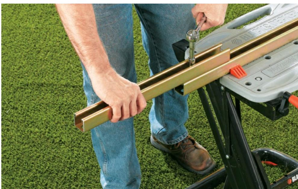
**3** Cut two additional pieces of strut to 4" less than the length of the expandable brace. Cut the expandable brace in half, then bolt both halves to the long center leg with four bolts. To expand the brace to the fall or winter position, just remove the bolts on one side, push the frame up, and then bolt the pieces back together. (Note that solar collectors usually stay in a fixed position year round, while PV panels benefit from being moved to summer and winter positions.)
