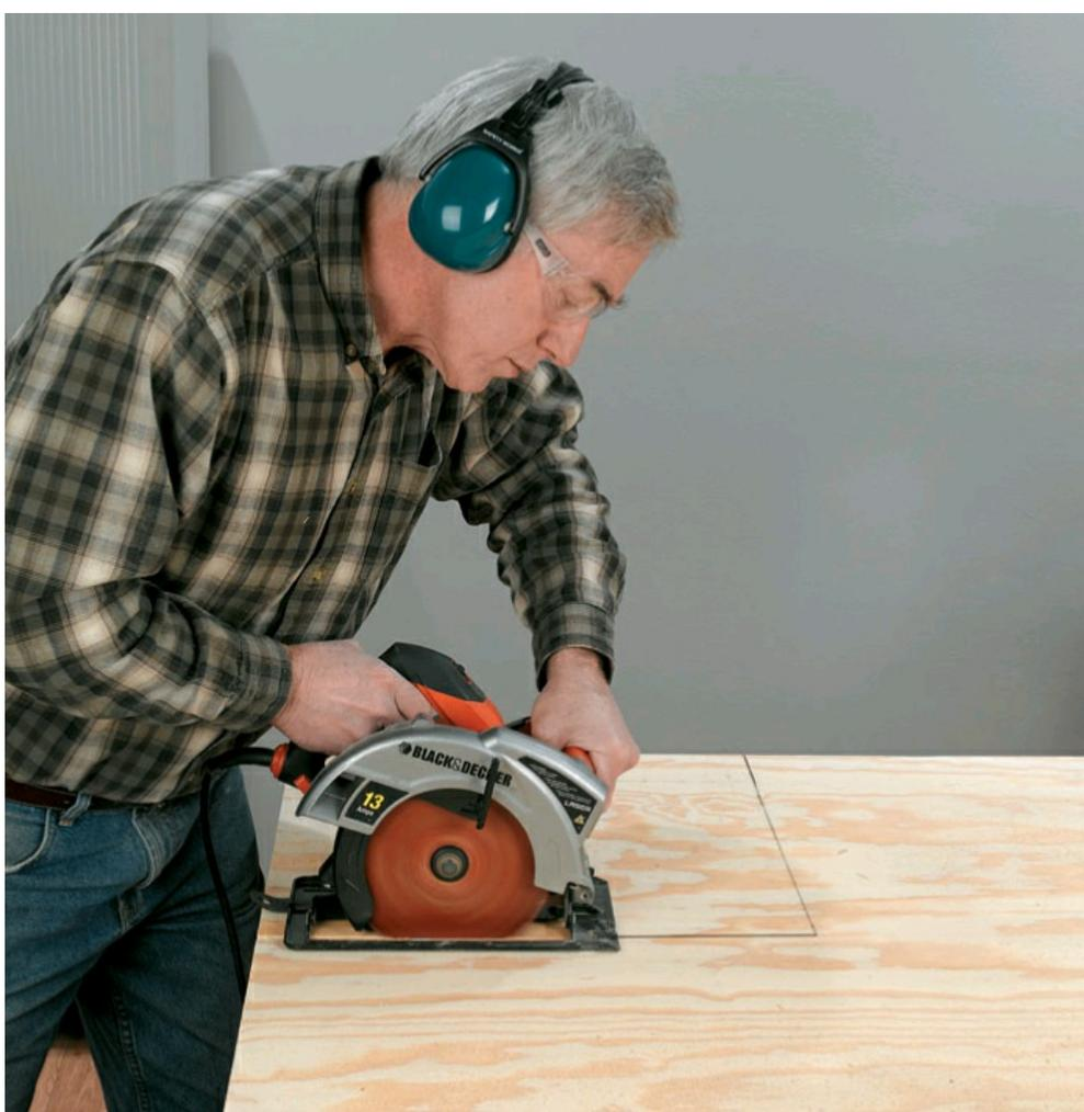
**2** Lay a 4 × 8-ft. sheet of plywood on the worksurface with the better side facing up. Select a good grade of 3/4" plywood (we used BC) or you're likely to have issues with parts warping, and you'll find it difficult to drive screws into the edge grain of the plywood. Mark and cut the 19 × 19" bottom piece first. Rest the full sheet of plywood on a couple of old 2 × 4s—you can cut through them as you make your cuts without any need to move them out of the way.
