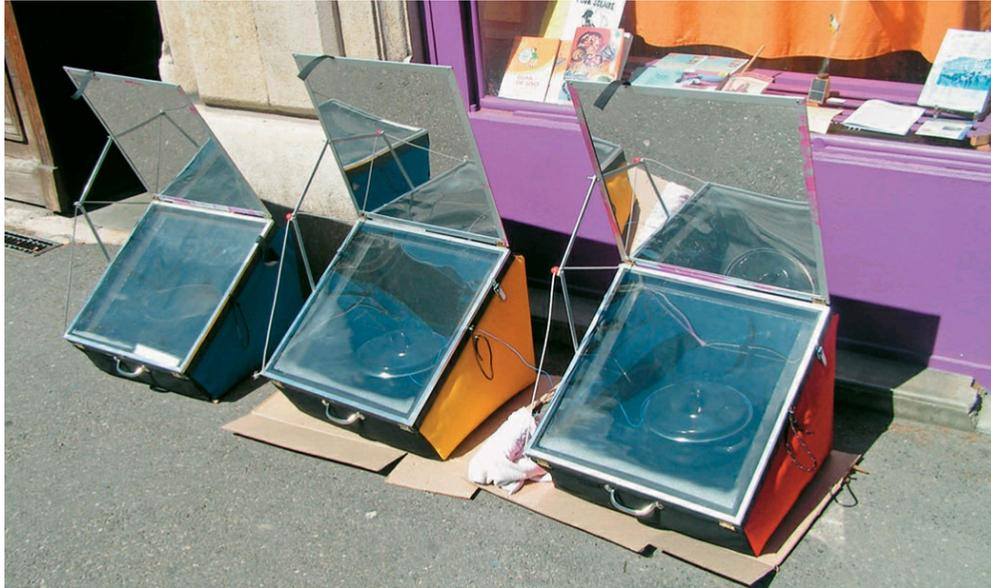
**Solar cookers can be made** in a wide variety of designs. The main criteria is that they have a reflective side or sides that focus sunlight toward a heat-absorbing (usually black) pot or base.
