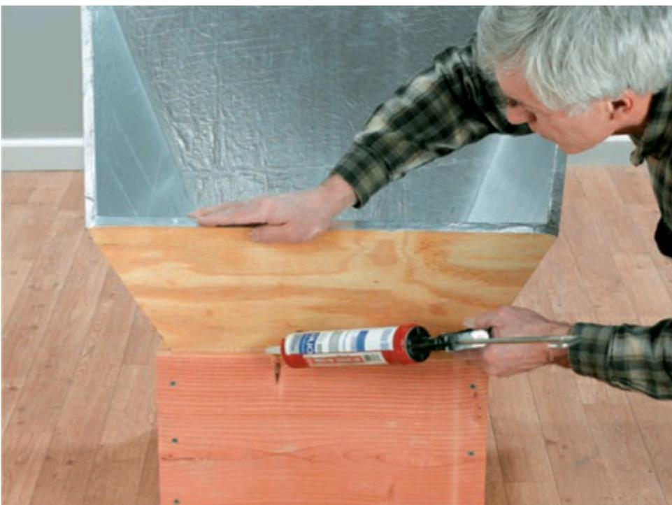
**3** Caulk the joint between the angled top and the base with clear, 100% silicone caulk. Set a wire rack inside the oven to keep the cooking pot slightly elevated and allow airflow beneath it.
