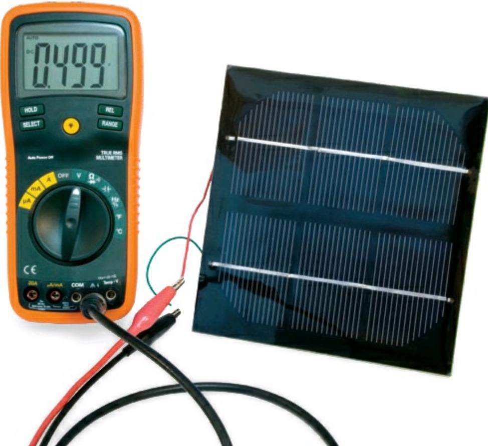
**A multimeter is a good diagnostic tool** for checking a photovoltaic panel to ensure it is working properly. It also allows you to check the power generated at different angles and locations.
