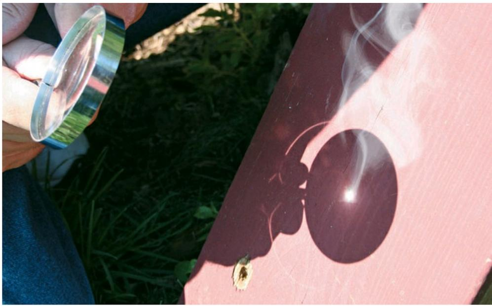
**The ability of a magnifying glass** to concentrate solar heat enough to start a fire has been known since at least 700 B.C. Solar collectors that concentrate sunlight use the same basic principle.
