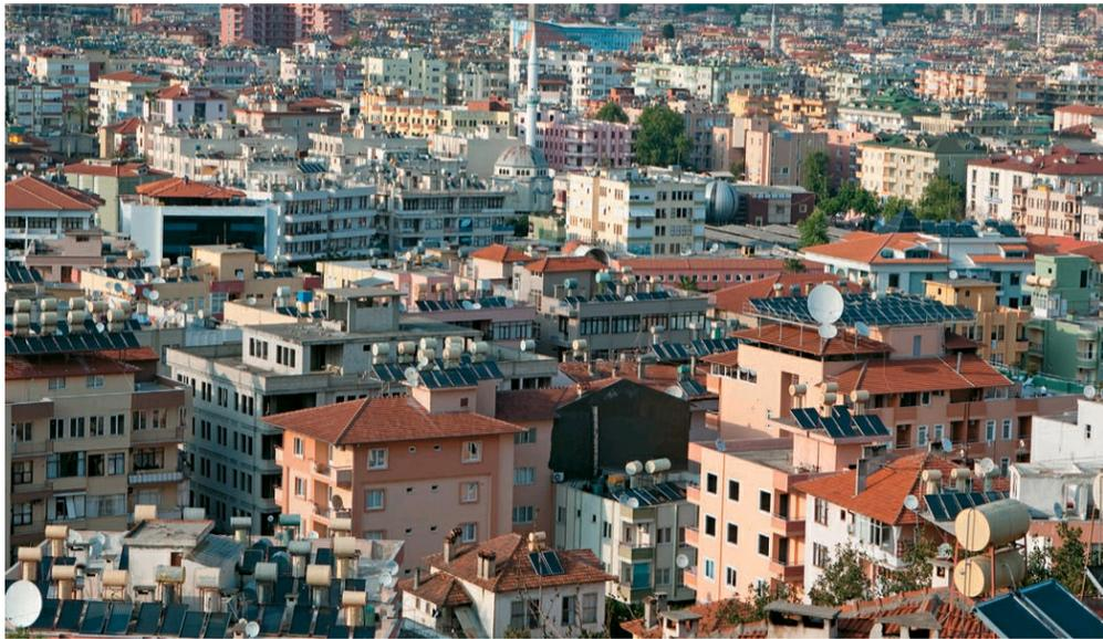
**Under the right conditions**—sunny climate, high energy prices, political support—solar hot water collectors can catch on fast. Notice all the black rectangular collectors on the roofs in this city on the Mediterranean coast of Turkey.
