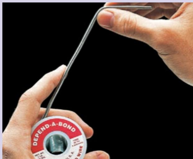
**Prepare the wire solder** by unwinding 8" to 10" of wire from spool. Bend the first 2" of the wire to a 90° angle.
