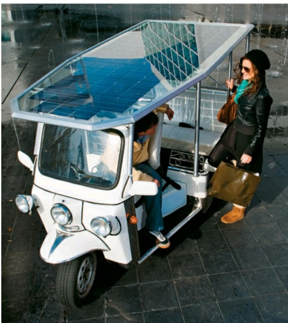
**This lightweight “tuk-tuk”**—a motorized rickshaw popular throughout Asia—uses solar panels and a bank of batteries for power. Extremely maneuverable and capable of speeds up to 30 mph, this non-polluting vehicle is perfect for crowded city streets.
