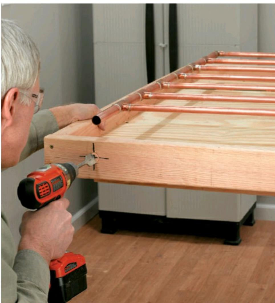
**8** Mark the location of the cold-water inlet and the warm-water outlet on the sides of the box by setting the copper grid into the box and extending the inlet and outlet port locations onto the outside of the frame. Drill the holes with a 1'-diameter bit.
