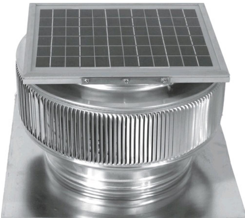
**A solar-powered roof vent fan** draws hot air from the attic during the day when the sun is out-the time when the attic is hottest. This type of fan generally does not include a battery, and is powered directly by the solar panel (although some manufacturers offer models with backup wind or AC power).
