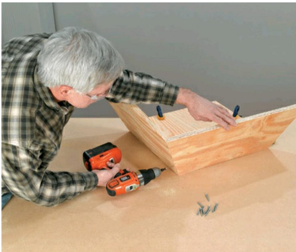
**6 Assemble the reflector.** Brace two of the reflector sides against a square piece of scrap plywood clamped to the work surface, then join the edges with screws driven into countersunk pilot holes. Repeat for the other two pieces, then join the two halves together with four screws at each corner, completing the reflector. The bottom edges should be aligned. The top edges won't match perfectly, so sand them smooth.
