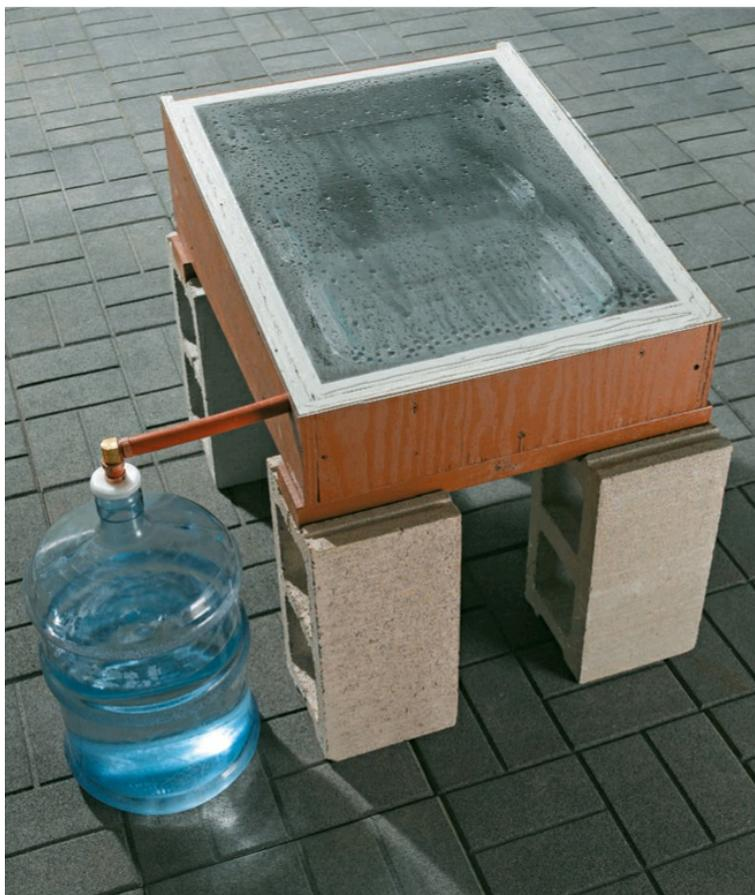
**Turn undrinkable water** into pure, crystal-clear distilled water with a home-built solar still.
