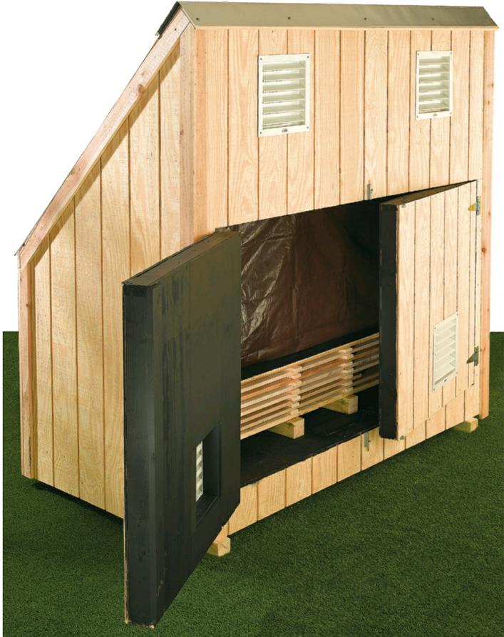
**Solar kilns dry lumber** as quickly and effectively as traditional kilns, but save money by using substantially less energy.
