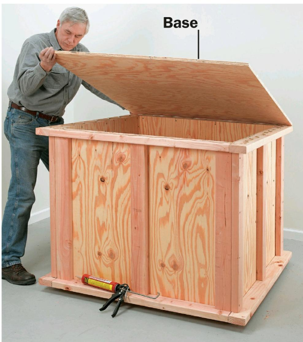
**5** Tip the box over, then glue and screw the plywood base to the 2 × 4 frame, aligning all the edges.
