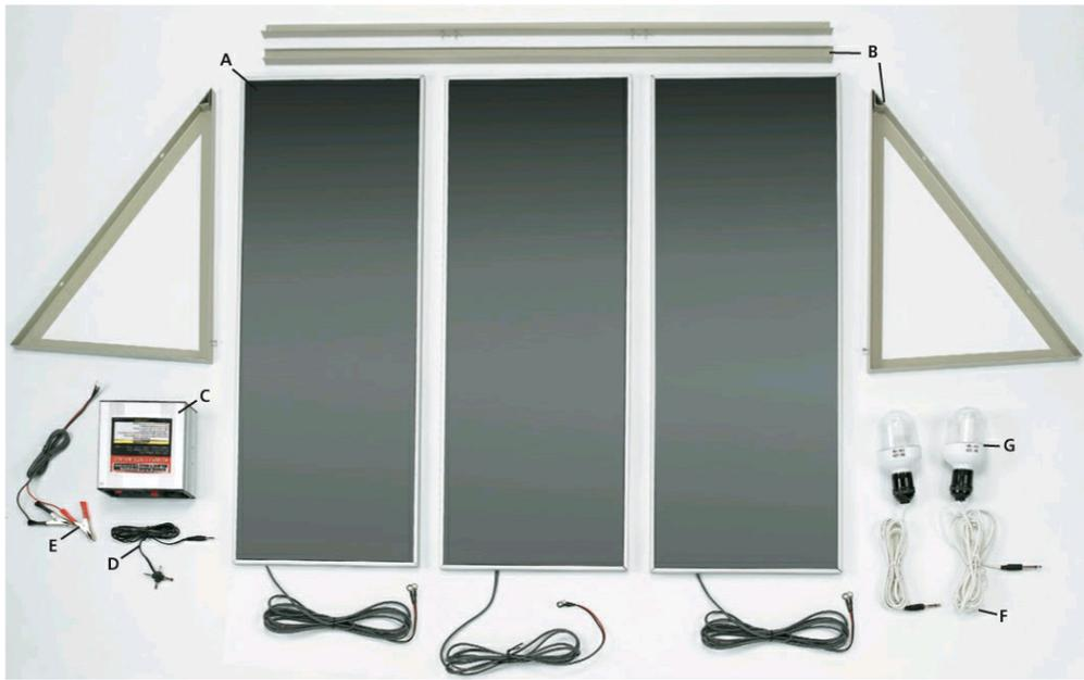
**Parts of this** solar light kit include: Three 15-watt photovoltaic panels (A); snap-in mounting stand (B); regulator (C); multi-purpose adapter (D); battery connectors (E); light wires (F); 12-volt LED lights (G). A 12-volt battery is required but not included with the kit.
