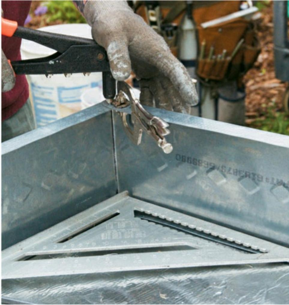
**3** Fasten the corners of the metal box with two 1/8"-dia. sheet-metal pop rivets in the top and bottom. Leave one corner open to create access for the insulation panel insert.
