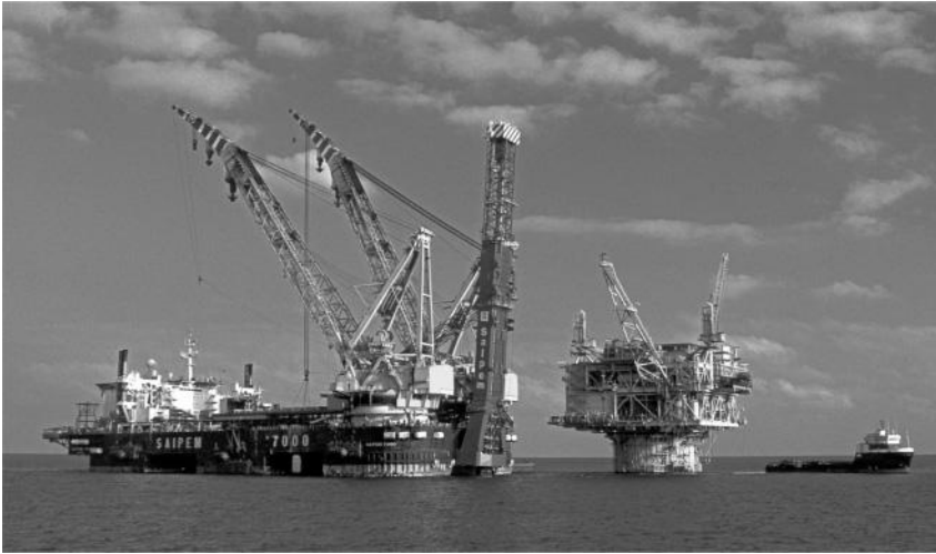
Figure 5.5 Saipem 7000, a 198 m long multipurpose crane vessel for placing off-shore hydrocarbon production platforms and laying pipelines in deep waters. It can lift 14 000 t up to 42 m (world record); its tower is 135 m high, and the overall weight of the
