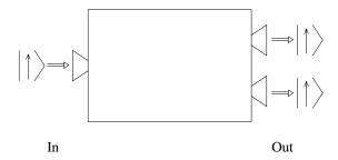
Fig. 8.4 Schematic diagram of quantum Xerox machine
