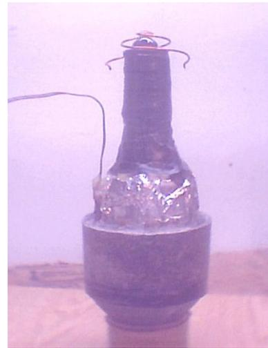
The coil is simply a double spiral coil. Two opposed arms radiate outward in a spiral pattern from an “S” shape in the center of the coil. Use # 15 AWG or thicker solid copper wire. Regular household electrical wiring, such as the type commonly used for 110 Volt Alternating Current in North America works great. In these pics I used # 15 AWG magnet wire with lacquer insulation. It should be a solid copper wire, thick enough to hold its shape once you have formed the coils.
