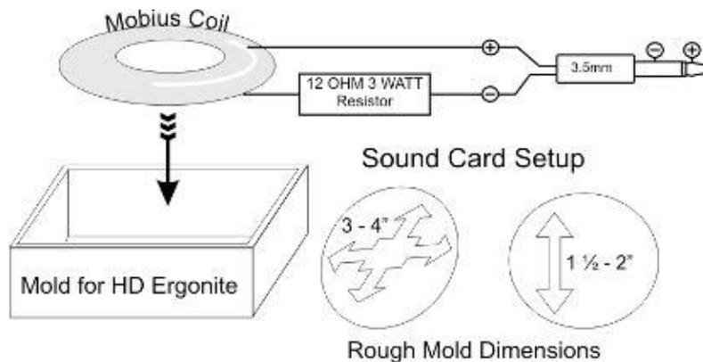
Make the coil and connect the leads to a length of 2 conductor wire long enough to reach from your sound source (PC or other audio device) to the place where you are pouring. Then connect the wires to the resistor and plug as shown. Plug it into the Headphone jack of your PC speakers and test it (turn on the audio signal). Adjust the volume on the PC speakers to about 1/3 power. Lay the coil in the center of the wet Ergonite
