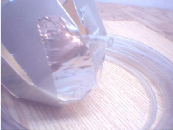
Cut about an inch of plastic tubing. Slide the coil leads through it, so that it forms a sleeve around the coil leads. Feed the ends of the leads through the tubing. Slide the tubing all the way up the leads until it butts against the coil. This is to protect the coil leads where they pass between the sharp edges of the metal reflector. You will have one seam on the reflector that joins the whole thing together. On this seam, at the
