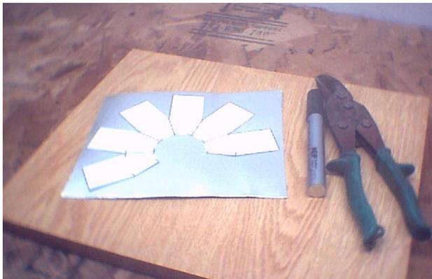
Resize the graphic if necessary, print it out on a sheet of paper, and cut around the outside edges of the black shape. Lay the paper template down on the aluminum flashing, working on a smooth firm surface. Hold the template firmly in place or secure it with a little tape.
