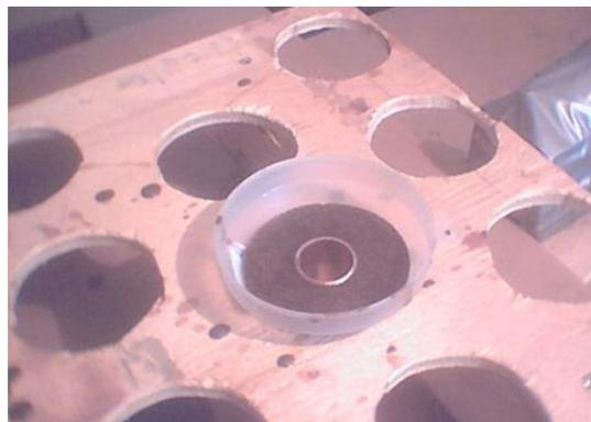
couple wraps of electrician's tape. Stretch the tape so that it forms a gasket around the seam where the pipe meets the funnel.
