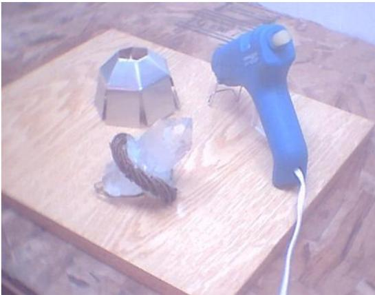
Bend along the white dotted lines to form the metal cutout into the shape shown in the picture. You will wind up with a hexagonal reflector with a small hole at the narrow end. Bend the tabs around the outside of the metal cutout up, so that they form sides for the reflector. Do the best that you can to get it neat, but again what matters here is that you have a metal enclosure for the coil and crystal. It does not have to be pretty. The enclosure should have a
