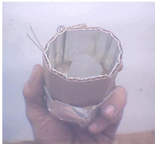
Once the tube is tacked in place, let it cool for a few minutes and then fasten it in place permanently with glue. Fill all the holes at the inside corners of the reflector and glue all the way around the seam where the reflector meets the tube. Fill the seam where the two ends of the strip overlap with glue to form a seal. You need
