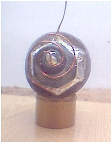
Cut two pieces of wire to a length of about ten inches. The length can be precisely measured if you are up on your resonant mass theory, but it does not need to be. I generally cut mine to 26.5 Centimeters. Any length between six and twelve inches will work fine.
