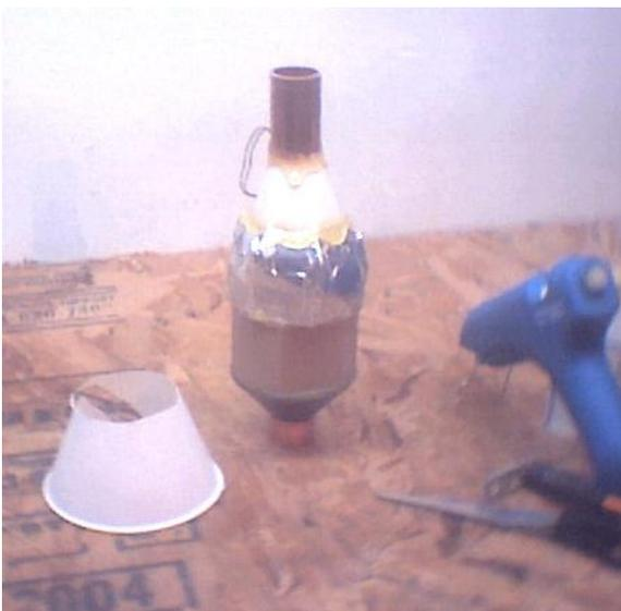
Press down gently on the paper cone and fasten it to the reflector base with hot melt glue. Use enough glue to form a good seal.
