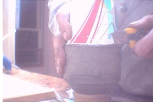
Handle the coil leads carefully and do not scratch the insulation on the coil leads with the sandpaper. Bubbles in this casting do not matter much unless they expose the core assembly. Bubbles in the base casting which expose the core assembly should be filled with Ergonite filler. Otherwise, the matter is purely a cosmetic one. Smooth off any ridges with a grinder or file if desired, and sand the entire project, including the copper pipe at the nose cone.
