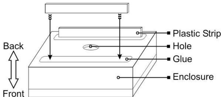
Once you have the ridges attached to the enclosure, remove the masking tape from the side of the pulser base and clean the area left unpainted with a little solvent. Apply construction adhesive or good silicone glue to the back of the box as shown. You should
