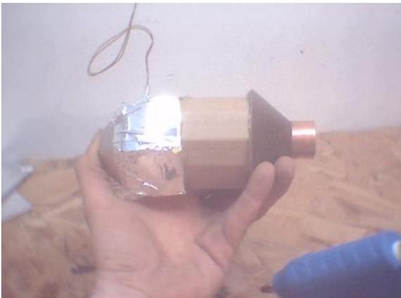
Using a file or grinding wheel, remove the sharp edge around the base of the Ergonite cone you just made. Rough up the flat base of the Ergonite cone with sandpaper, and wipe it clean with a little solvent or alcohol. Test fit it on the end of the cardboard tube. The axis of the copper pipe should be parallel to the axis of the cardboard tube. Line it up as best you can so that the copper pipe is parallel to the sides of the cardboard tube. The Ergonite cone does not have to be perfectly
