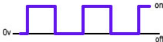
Simply put, the current switches on and off very rapidly. This type of signal in the coil will produce a rapidly expanding and collapsing magnetic field. The magnetic field is the exciter that essentially kicks the ergonite into action.
