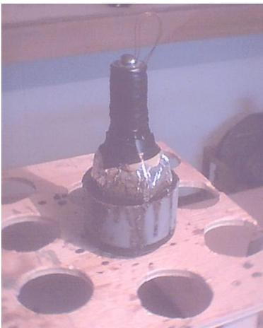
Use a grinder or rough sandpaper to smooth off the sharp lip on the base of the nose cone Ergonite casting. Rough up the surface of the base of the nose cone casting, the side that was the top when you poured the Ergonite. Check the surface of the core assembly for potential leaks again, and wipe the outside of the cardboard tube and aluminum reflector with a little solvent. Wipe the base of the nose cone casting that you just sanded with a little solvent also.
