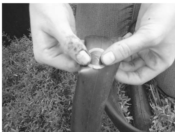
Figure 2-17 Press the patch onto the inner tube and hold for a second. If some glue leaks out the sides, spread it around the edges and make sure they are securely stuck to the tube. The edge of the patch is a common place for leaks to reoccur.
