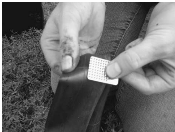
Figure 2-14 Scrape the tube gently, to clean the surface and give the glue a rough area to adhere to. Be careful, as it is possible to create a bigger puncture at this stage.
