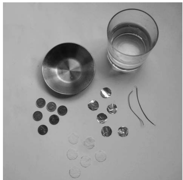
Figure 10-6 Simple materials for this project: a dish, coins, aluminum foil, wire, and salty water.
