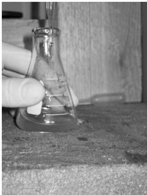
Figure 14-11 The beaker placed under the pipette with a measured volume of distilled water added slowly.
