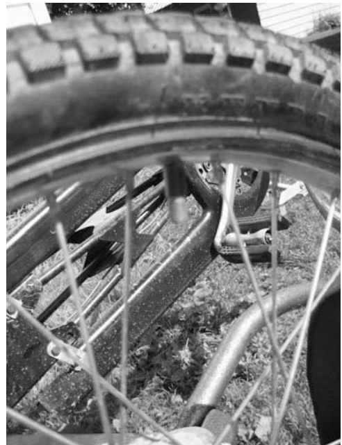
Figure 2-10 Detail of the valve; push it back into the rim before trying to remove the inner tube.
