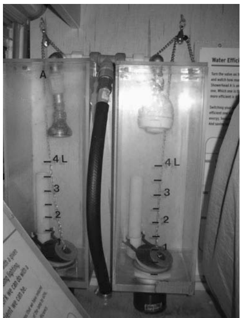
Figure 6-9 A dramatic demonstration of how much less water is used by a low-flow showerhead, on the Climate Change Bus at the Falls Brook Centre, New Brunswick. Both showerheads empty into graduated sealed containers using the same water pressure. The message: for the same shower, a low-flow showerhead uses less water.
