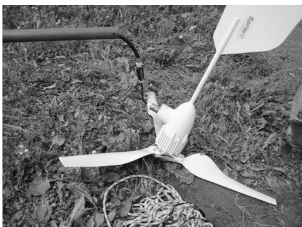
Figure 12-25 The turbine wired up, with the protective cover closed.
