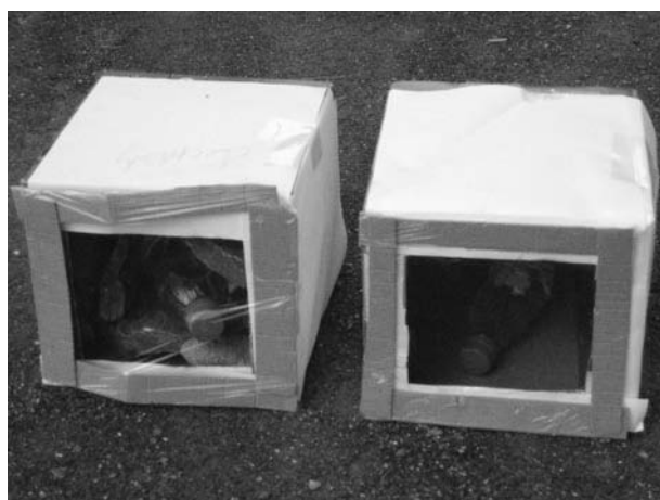
Figure 3-15 “Model rooms” with and without thermal mass inside.
