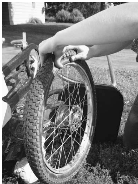
Figure 2-21 With the newly repaired inner tube inside, start pushing the tire back onto the rim.
