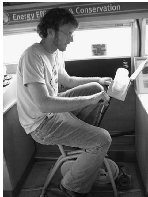
Figure 5-6 A tactile demonstration of the amount of work needed to light a bulb, by pedaling an old exercise bike attached to an electric generator. The generator powers one of two lights in front of the rider. When the switch is flipped from the incandescent to compact fluorescent, the work the rider must do to light the bulb is much less.
