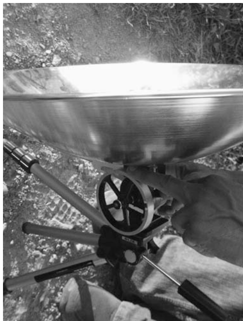
Figure 9-18 Use one finger to start the engine turning. On a larger system, an automatic starter would of course serve this function.
