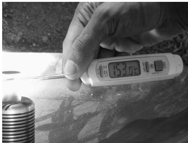
Figure 9-19 Use a simple oven thermometer to measure the approximate temperature at the apex of the concentrator dish.
