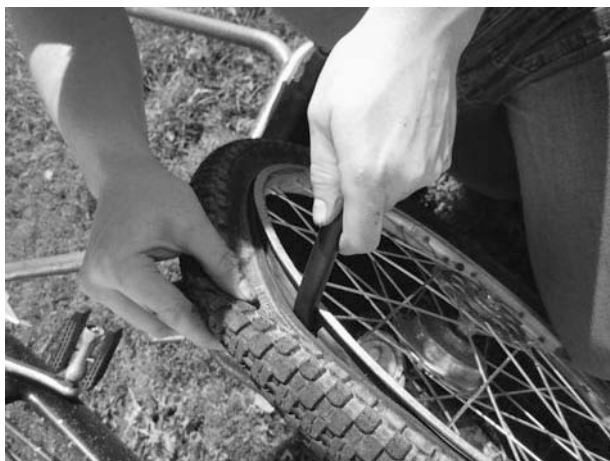
Figure 2-6 Pushing the flat end of the tire iron under the edge of the tire.
