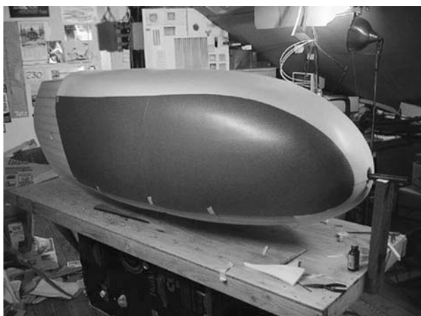
Figure 13-33 The two colors joined after having been heat-formed separately.
