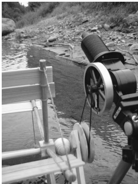
Figure 9-20 The Sun Runner Stirling engine, attached by a thin belt and powered by the model water wheel from Chapter 8.
