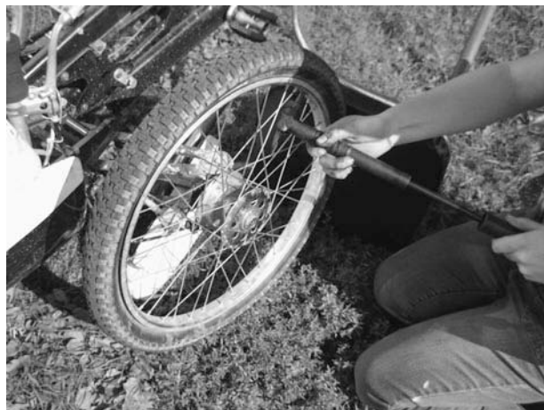
Figure 2-23 Fill the tire with air, and check the pressure (read on to the next project if you are unsure how to do this).
