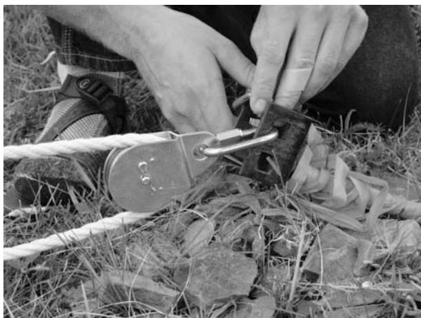
Figure 12-14 The pulley attached to the lift anchor.
