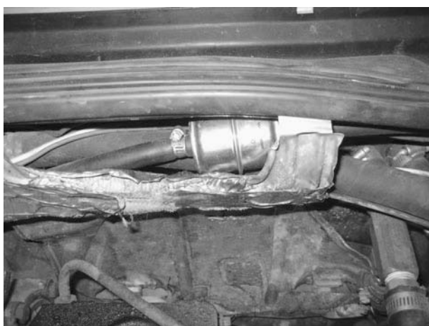
Figure 14-22 Second and even third filters on the vegetable oil side of your fuel system help protect your engine from small pieces of food waste.
