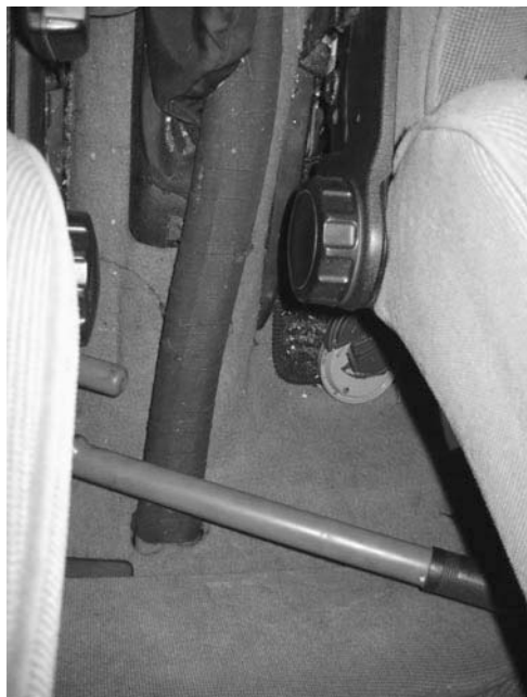
Figure 14-18 The hoses filled with radiator fluid and, through the center in its own tube, heated vegetable oil, running through a hole inside the vehicle.
