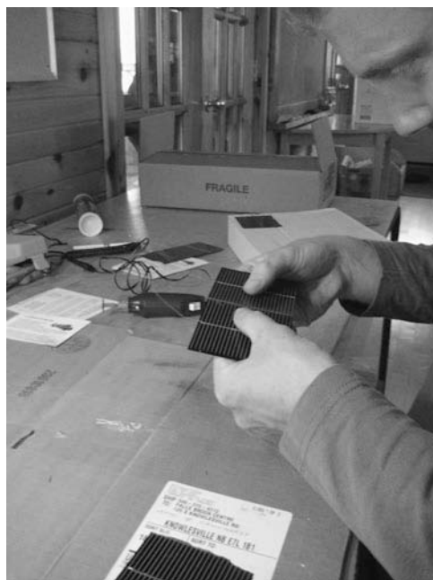
Figure 11-9 Grasp the cell firmly with both hands, and press with all four fingers on the underside and your thumbs on top.
