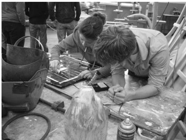
Figure 11-18 Solder the connections between rows of cells.
