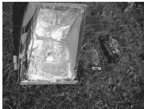
Figure 7-9 The insulated solar cooker with a clear plastic bottle of water being purified inside. To the right are the water purifiers from an earlier project, which were all worse at capturing the sun's heat than this simple pizza box cooker.
