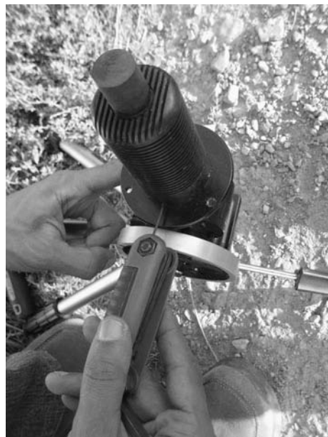
Figure 9-17 Tightening the tiny Allen bolts on the side of the cylinder body that hold it in place and keep a tight seal.
