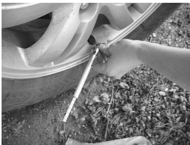
Figure 2-25 Using a tire gauge to check the correct pressure.
