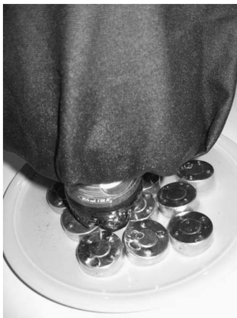
Figure 6-6 Salvaged metal pieces form a base for the bottle of pop on top of a water-filled plate. A metal cage covered in damp fabric is being lowered over the top to induce evaporative cooling of the drinks.
