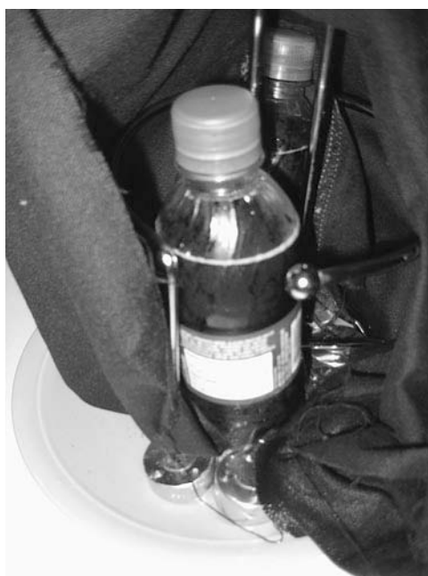
Figure 6-7 The cage of the easy-to-build evaporative cooler is shown.
