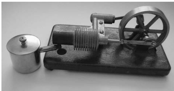
Figure 9-3 The Thinking Man's Engine, available as a kit from PM Research Inc., is a gamma-type engine. It is shown with the optional burner under the hot end of the displacer piston. The separate power piston is seen attached to the far side of the flywheel, which regulates the phase of the piston movements inside the cylinders.
