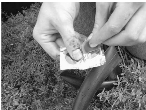
Figure 2-15 Peel both sides of protective packaging off of the patch. Start by rolling the patch away from the aluminum backing at one corner and then peel diagonally to avoid tearing the patch.
