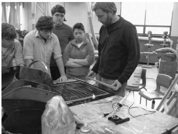
Figure 11-25 Sizing pieces of the (reclaimed) aluminum frame.
