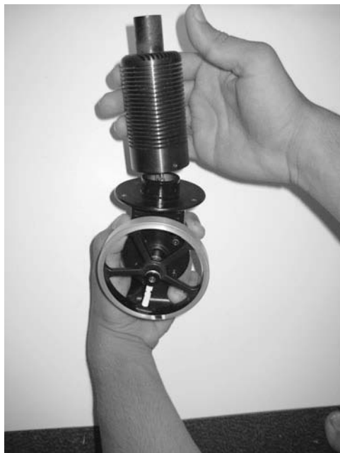
Figure 9-16 Sliding the cylinder and cooling fins onto the body of the Sun Runner model Stirling engine.
