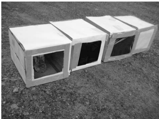
Figure 3-6 Four model rooms with reused hot water bottle “heat sources” inside, cooling down in the waning sun. The model room on the far left has no curtains, to its right is the model room with no window, followed by a thick curtain in the window, and a thin curtain (kitchen towel) in the last window. All windows are made from plastic wrap, on a cardboard frame mounted on identical cardboard boxes.
