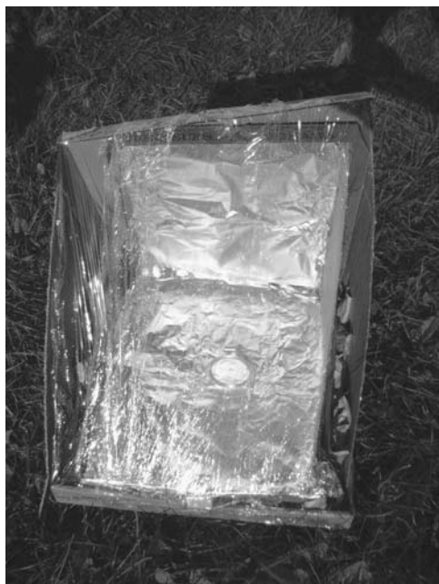
Figure 7-6 The completed pizza box solar cooker in the sun. The temperature inside reached a balmy 70°C (158°F) within 90 minutes on a partly cloudy day—temperature of 25°C (77°F)—in New Brunswick, Canada.
