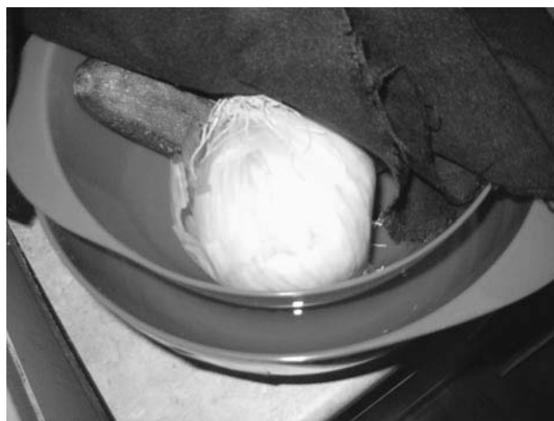
Figure 6-5 An experimental, modified Zeer fridge made from common household mixing bowls. The vegetables inside stayed fresh until used.
