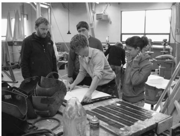
Figure 11-17 Lay down a piece of paper to protect the connections behind the cells.
