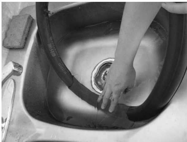
Figure 2-13 Place the inner tube in a bucket or a sink with some clear water in it. Look for bubbles, which indicate where there is a leak. Mark the spot once you find it.
