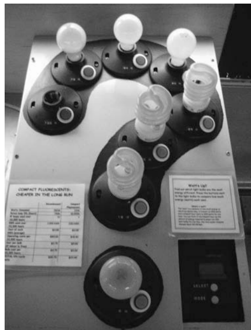
Figure 5-5 A demonstration unit that shows the energy consumption of a variety of bulbs, and allows users to notice that the same amount of light can have large variations in energy use. Shown on Big Blue, the Climate Change Awareness bus run by the Falls Brook Centre.
