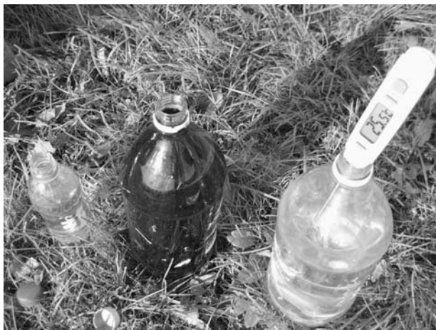
Figure 6-2 Taking the starting temperature, with an inexpensive digital oven thermometer, of the water inside one of two large solar water purifiers. A third smaller version is also visible on the left.
