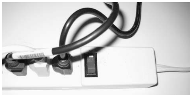
Figure 5-8 A power bar in use. Note the power button to the right of the plugs, which is not normally perceived as an energy conservation tool, but if used correctly could save you money by eliminating “ghost loads.”
