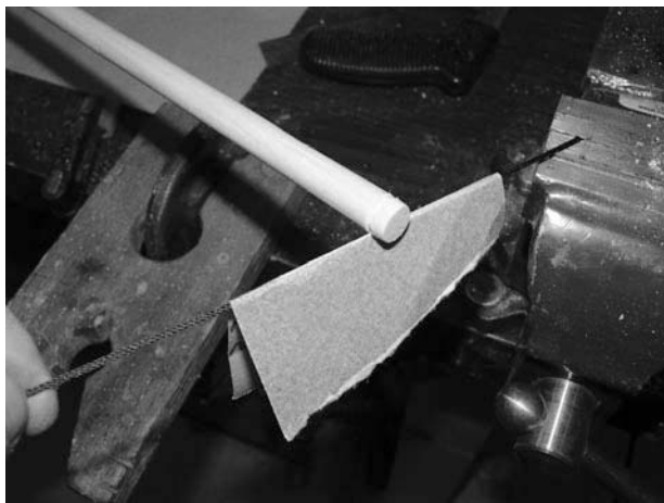
Figure 8-21 Making the groove in the wooden dowel using a piece of string and some sandpaper. Photo courtesy of Rob Bicevskis.
