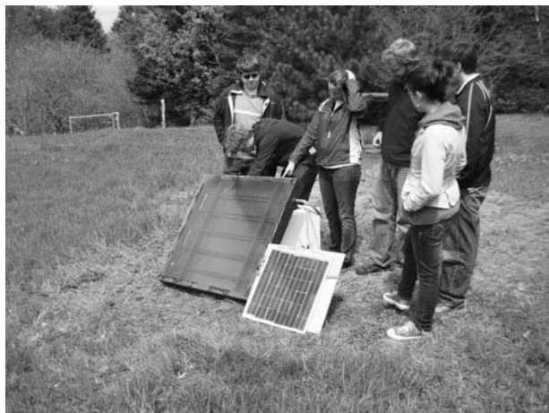
Figure 7-17 Builders of the winning solar thermal collector check on its performance. The solar electric panel to the right powers the pumps, again hidden behind the thermal collector and doubling as a stand.
