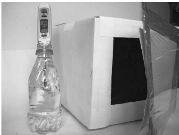
Figure 3-5 Taking the temperature of the warm water with a digital oven thermometer before it is put into the “model room” with a light curtain.
