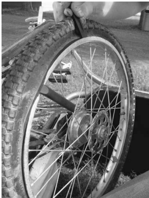
Figure 2-8 Insert a second tire iron; then, slide it along the rim to free one edge of the tire.
