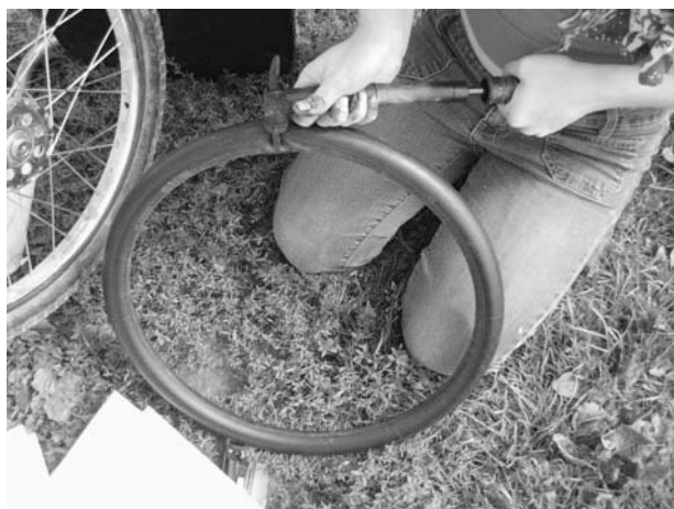
Figure 2-12 Filling air into the inner tube with a hand pump.
