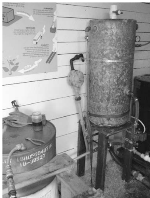
Figure 14-7 The methoxide mixing vessel (on the right), which is vented and feeds directly into the main reactor pictured in Figure 14-5.
