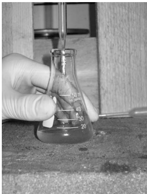
Figure 14-12 Note the volume of reactant added when the reaction starts to take place.
