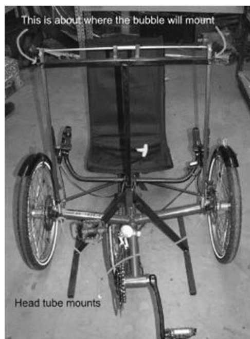
Figure 13-25 Details of where the veloKit will attach to the average tricycle.
