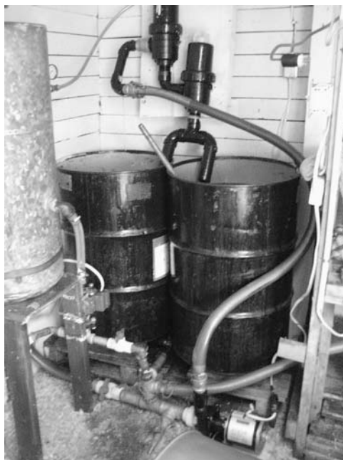
Figure 14-4 The biodiesel processor at the Falls Brook Centre in New Brunswick. Two filters above the heated black barrels are fed by a pump near the floor, which circulates and filters the oil constantly as it is heated.
