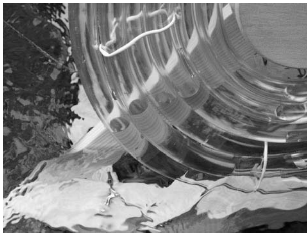
Figure 8-16 Alternating columns of air and water gathered in the spiral pump. As the diameter of the spiral gets smaller, the air is compressed. The alternating columns of water and compressed air can then be turned away from the spiral and sent up an elevation to do work.
