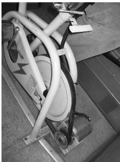
Figure 5-7 Details of how the exercise bike is attached to the generator, for you truly evil geniuses who will undoubtedly try this at home.
