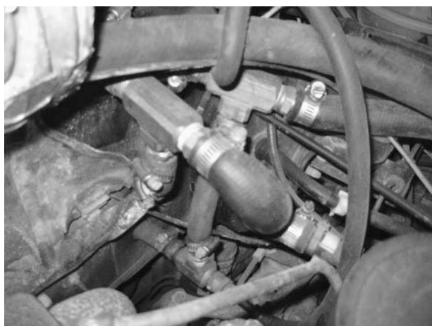
Figure 14-19 The extra addition to the radiator system is about center in the photograph. Two T-junctions tap into the existing system and feed hot fluid down to a second set of T-junctions, through one of which runs a tube filled with heated vegetable oil.
