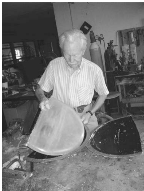
Figure 13-9 Carl Georg Rasmussen, builder of the Leitra velomobile, removing the fiberglass wheel cover from the mold at the factory in Denmark.
