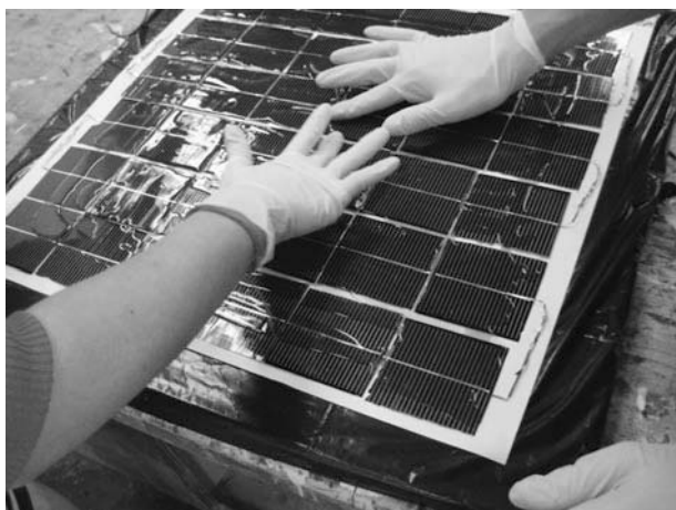
Figure 11-21 Spread the silicon out evenly over all the cells.
