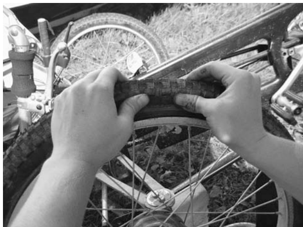
Figure 2-22 Use your thumbs in a rolling action to coax the last parts of the tire onto the rim. No tools are needed at this point!
