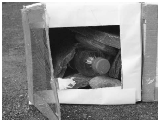
Figure 3-14 Thermal mass (large rocks) surrounding the warm water bottle in a “model room.”
