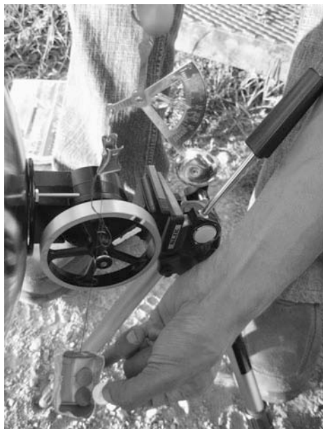
Figure 9-15 Add a coin to the basket and record the apparent weight while the engine is running. Using a high-speed video camera (not shown), or other device to record the speed, will enable you to calculate the power produced by the engine under different loads.
