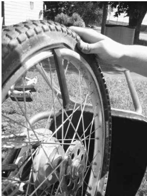
Figure 2-7 Hook the tire iron to the spokes once the flat side is inserted under the tire.
