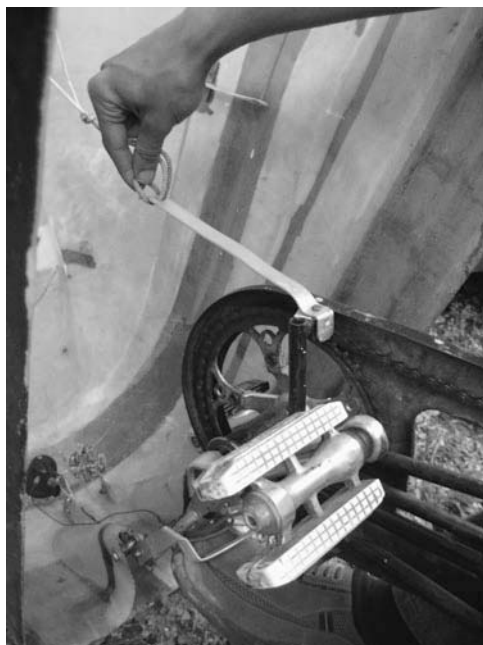
Figure 13-13 Detaching the lightweight device used to keep the front fairing from rotating too far forward.
