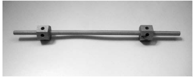
Figure 8-5 The wooden axle and pre-drilled hexagonal hubs from the Walter Kraul kit.
