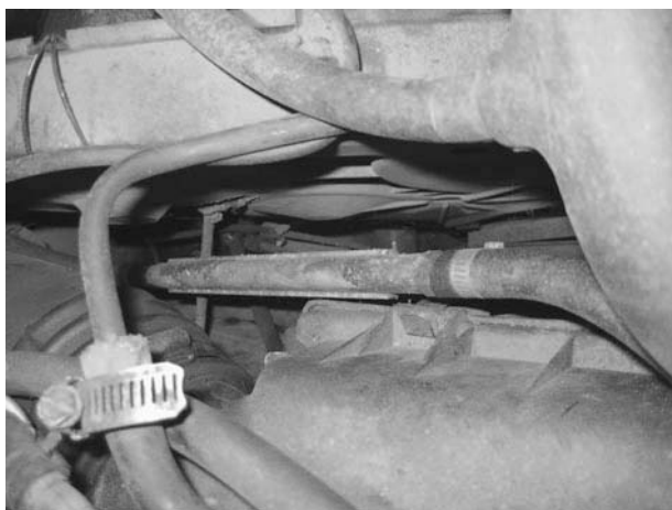
Figure 14-21 The Vegtherm electric fuel line heater (above center—also visible in Figure 14-20) provides a secondary heat source on this cold-weather system, but could be sufficient on its own in a warmer climate.
