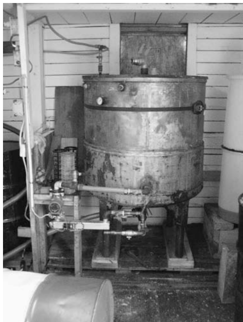
Figure 14-5 The main biodiesel reactor has a water jacket that maintains the required temperature during the reaction of methoxide and vegetable oil. The glycerin and then biodiesel is drained from a valve at the bottom, and the tank is fed via a pump through an inlet at the top.
