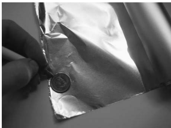
Figure 10-7 Cutting penny-sized circles from tin foil.
