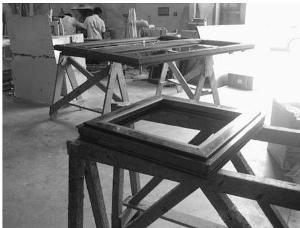
Figure 3-12 Sealed double-pane glass windows awaiting assembly in a factory. A layer of gas is trapped in between panes of glass at the factory, resulting in significant energy savings compared with a single-pane window.
