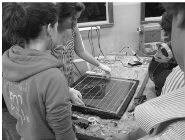
Figure 11-22 Gently position the glass over the silicon and cells.
