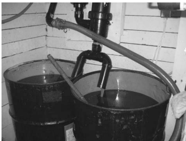
Figure 14-9 Warming the used oil in this large-scale system includes filtering it and continuous pumping to ensure a good mix of the oil.
