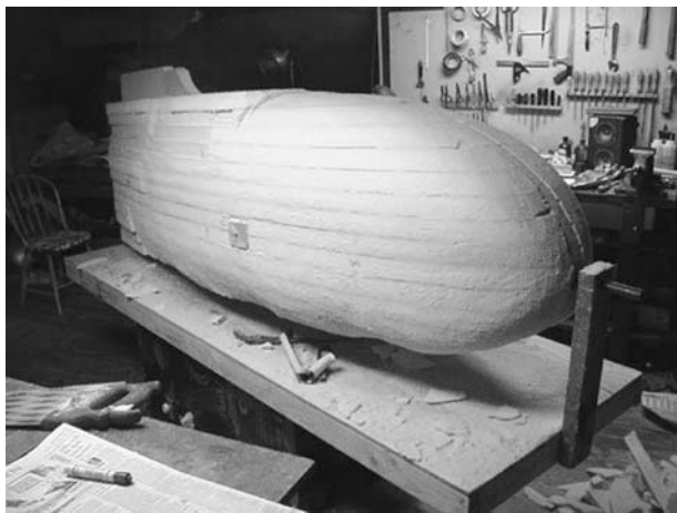
Figure 13-29 The male mold ready for sanding.
