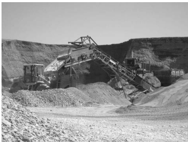
Figure 15-2 Gravel is a component of lots of things, including the concrete in most foundations, and is usually mined in large open pits like this. The concept of the embodied energy of the materials you use assesses a portion of the energy consumed by such an operation to the materials you use.
