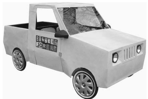
Figure 13-5 A four-wheeled two-passenger Rhoades Car with a lightweight fairing designed to mimic a pickup truck. Image courtesy of bicycleforest.com.
