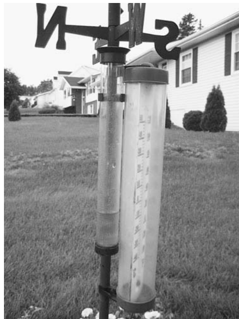
Figure 6-13 This inexpensive commercially sold weather system can assist in understanding the rainwater resource available in the local area and is helpful when planning for a larger system.
