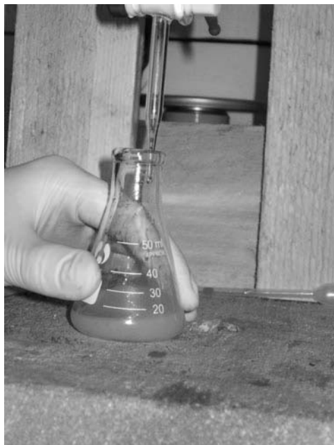
Figure 14-13 Stop adding reactant when you can see the color of the liquid inside the beaker change.
