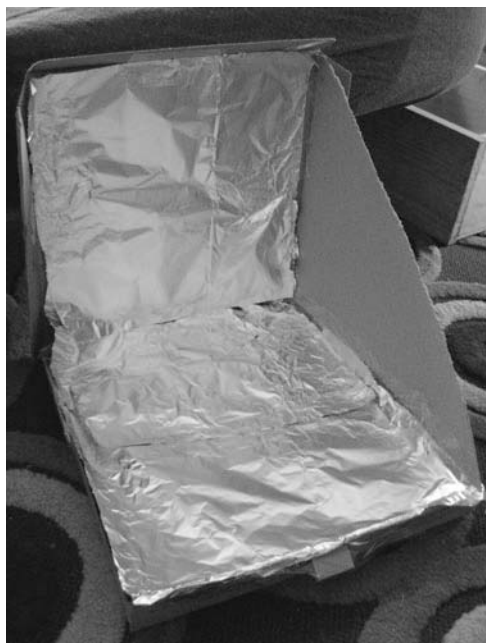
Figure 7-4 Tin foil lining the inside of the smaller pizza box, which will sit on top of the layer of paper insulation.
