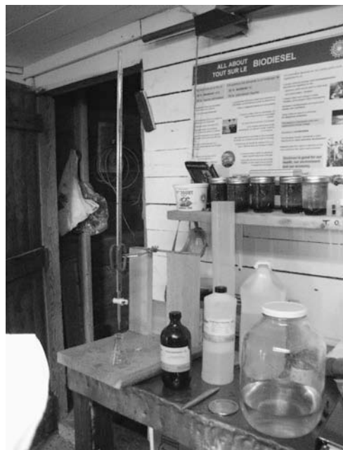
Figure 14-8 A pipette, distilled water, and other materials required for a titration.
