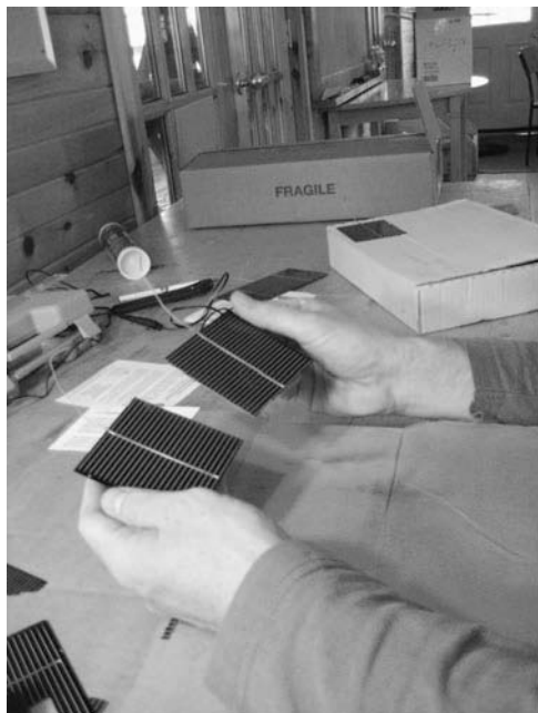
Figure 11-10 Gently “crack” the cells apart along the score line.
