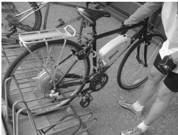
Figure 13-40 The BionX electric assist system is a popular choice for cyclists. It replaces the rear wheel in a very simple operation that can be performed on most bikes.
