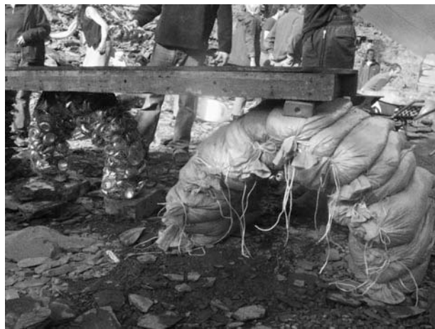
Figure 15-6 Two arches made of composite materials—on the right is an earthbag arch and on the left an arch made from reused aluminum cans and some chicken wire—shows the potential strength in individually weak materials.
