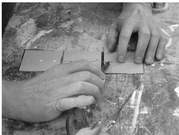
Figure 11-13 Solder the connection together and be careful not to put any pressure on the cells.
