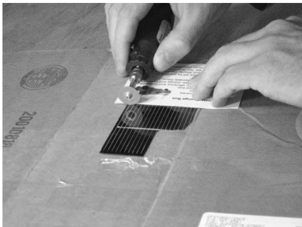
Figure 11-6 Using a straight edge to score a slightly damaged cell—practice first on one that is quite damaged, to get your skills up.
