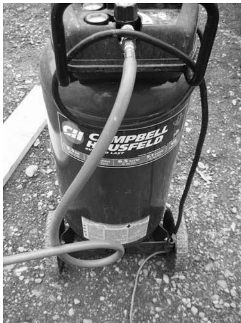
Figure 8-12 A commercial electric air compressor and high-pressure tank, used on construction sites as a portable power source, like a chemical–electrical battery.
