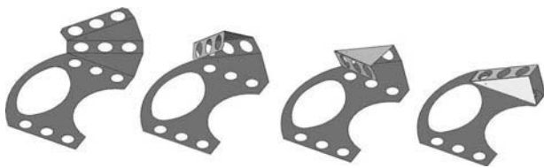
Figure 9-10 One of the diagrams from the Eco-Power Stirling Engine kit shows how to fold the superstructure. Image courtesy of www.stirlingengine.com .
