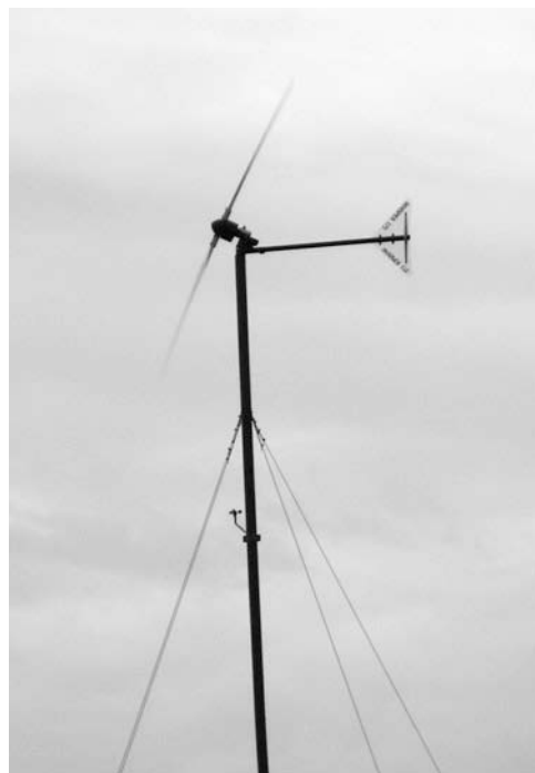
Figure 10-11 The Aurora turbine tilting out of the wind to protect it from spinning too fast and damaging the turbine or electronics.
