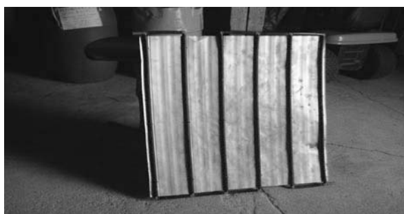
Figure 7-15 The completed basic collector. The inlet is visible at the bottom right, the outlet at top left.
