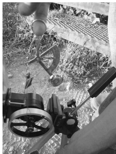
Figure 9-14 Scale and cotton cord wrapped around the axle of the solar Stirling engine, acting as a breaking dynamometer. Note that for accuracy, the scale should be held securely in place and a more accurate scale could be used.
