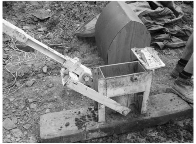
Figure 15-9 An earth brick maker works by compressing a small amount of earth into a small brick, which can be used to create all manner of structures.
