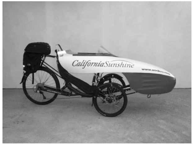
Figure 13-3 The Leitra front fairing fit to an inexpensive recumbent tricycle, named “California Sunshine.” Image courtesy of Leitra.dk.
