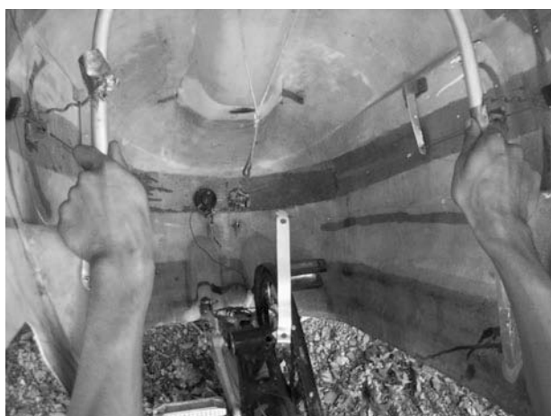
Figure 13-15 Lift the front fairing off with two hands on the aluminum support bar; and carefully place it on the protective wrap.
