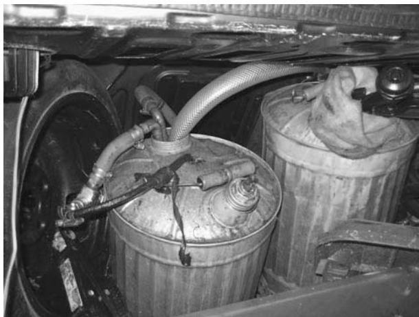
Figure 14-17 Two metal jerry cans repurposed as vegetable oil tanks in the trunk of a VW Jetta. The tank on the right provides extra storage capacity and holds a prefilter, which enables raw grease to be collected from restaurants. The tank on the left is heated by copper pipes filled with radiator fluid, and has a fuel line running through the radiator fluid up to the engine.
