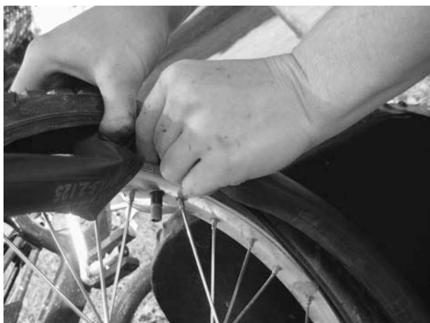
Figure 2-19 Feed the valve stem on the inner tube through the hole on the rim.
