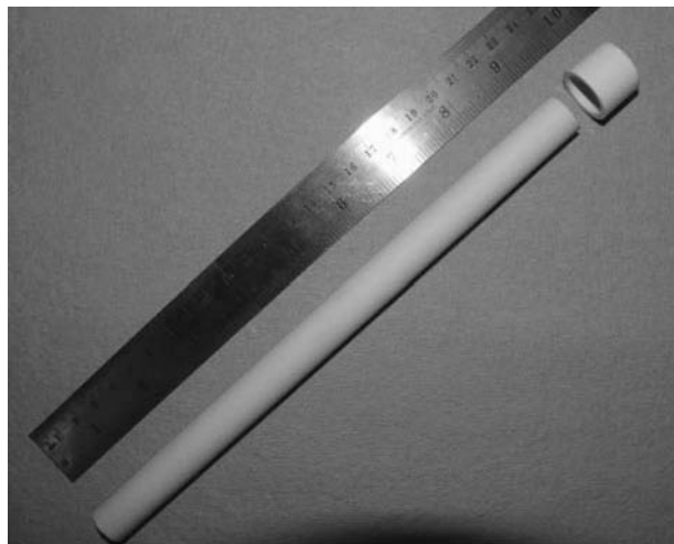
Figure 8-19 Length of PVC pipe and cap used for the model T fire piston. Photo courtesy of Rob Bicevskis.
