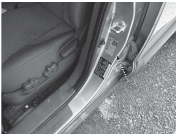
Figure 2-24 Location of the label on the inside of the car door, showing the correct tire pressure for the vehicle.
