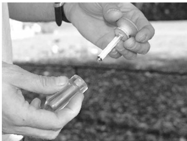
Figure 8-25 A smaller fire piston with its ember burning. Photo courtesy of Rob Bicevskis.
