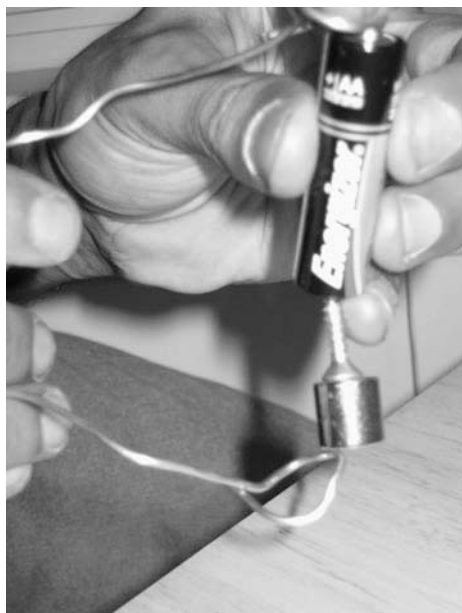
Figure 10-5 The assembled spinning screw-type homopolar engine.
