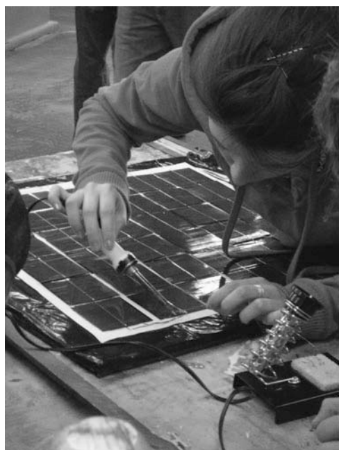
Figure 11-19 Take care not to put any pressure on the cells and check the electrical connection before going on to the next step.
