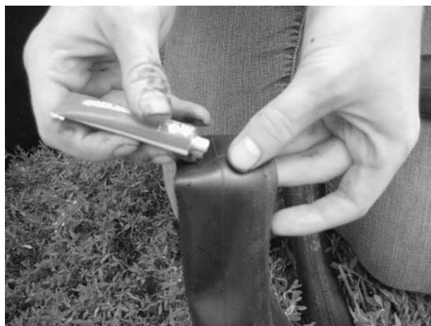
Figure 2-16 Apply some glue to the tube over the patch you previously scraped.
