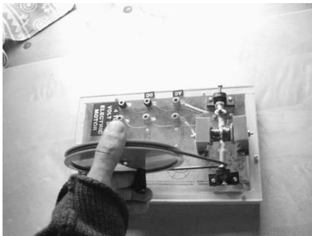
Figure 10-3 The layout of a demonstration electric generator kit: a large wheel is hand-turned to drive an electric generator, creating current at the terminals.
