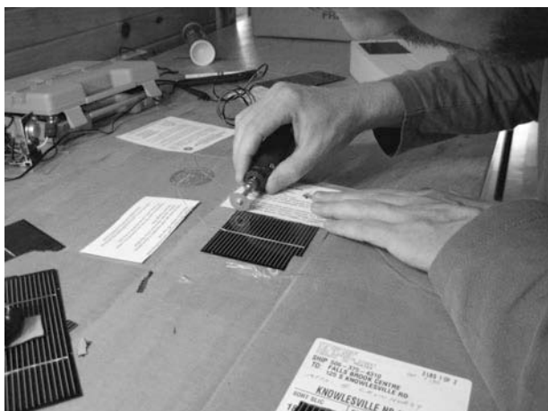
Figure 11-7 Scoring a less imperfect photovoltaic (PV) cell in half. Be gentle, they are very fragile!
