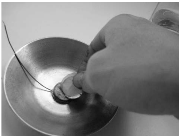
Figure 10-8 Layering coins, aluminum, and wet paper towel to form a battery.
