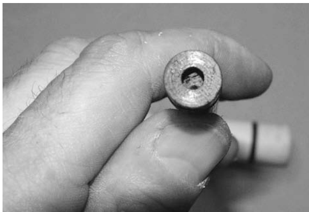
Figure 8-23 Detail of the bottom of the piston, showing where the small amount of fire-starter will sit. Photo courtesy of Rob Bicevskis.
