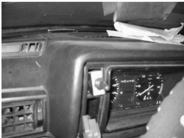
Figure 14-23 The electric switch that will connect to your solenoid and change the fuel source from diesel to straight vegetable oil. You will need to remember to turn it back to diesel a few minutes before arriving and turning the car off, or else starting again will be a problem.
