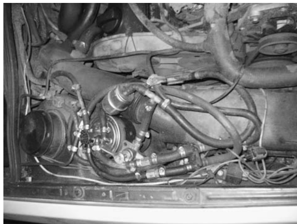
Figure 14-20 The location where the fuel line has been cut into, and the six-port solenoid (a little left of center) in the photograph. An emergency return valve has also been fitted to this system to enable air bubbles to be cleared after a filter is changed.
