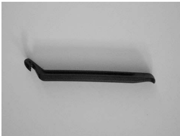
Figure 2-5 Detail of a common tire iron (now made out of plastic), showing the end (pointing down) that interacts with the tire.
