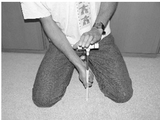
Figure 8-24 The completed model T fire piston. Push down on the T while it is in the cylinder; the O ring forms an airtight seal that results in air compressing at the bottom of the piston, setting the fire-starting material alight.
