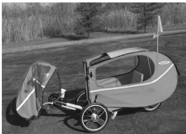
Figure 13-24 How the veloKit opens to enable the driver to enter and exit.
