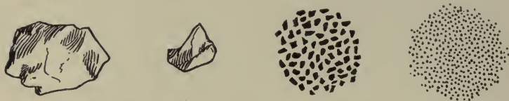
COMPARATIVE SIZES OF SAND AND CLAY PARTICLES (ENLARGED)
