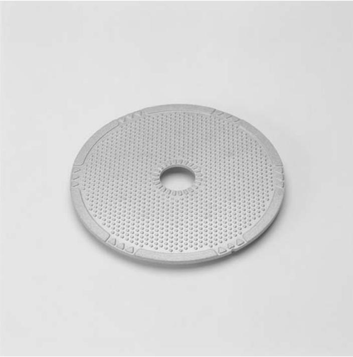
**Figure 4.13** Electrolyte of the Hexis SOFC
