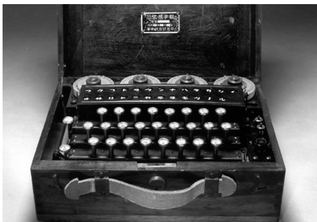
Fig. 78. Japanese ENIGMA imitation, GREEN machine
