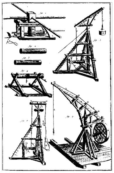
FIGURE 8.1. Early rotating cranes and other devices for raising or moving loads. (From Diderot and d'Alembert, *Encyclopedic* [1751-1772], reproduced in Fitchen 1986.)
