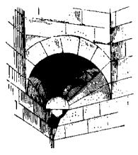
Squinch. A corbelling, usually a small arch or half-comical niche, which is placed across the corners of a square bay in order to form an octagon suitable for carrying an octagonal cloister-vault or a dome. [Krautheimer 1981.]
