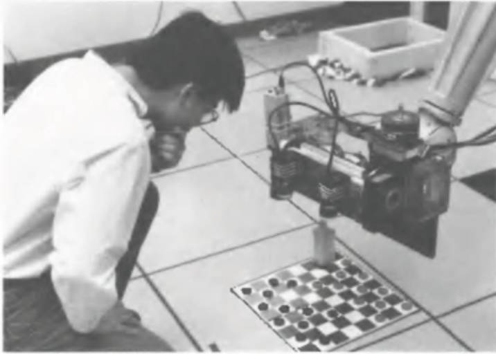
Figure 51.1. Rochester checkers playing robot. (Photo courtesy of James Montanus and the University of Rochester. Photo by Chris Brown.)
