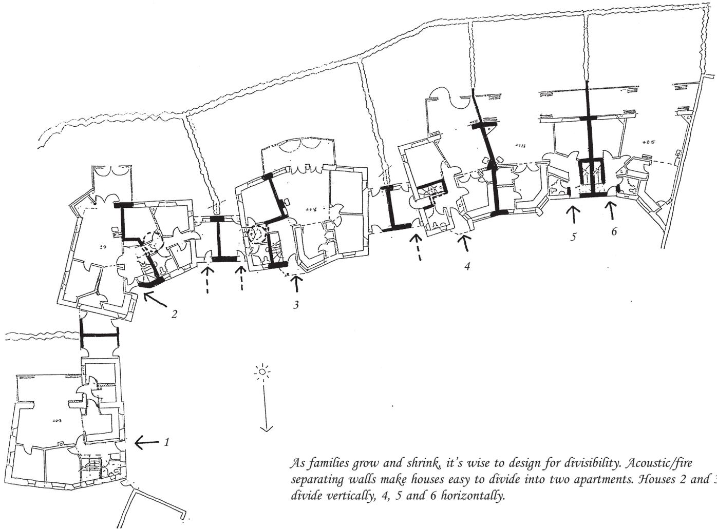
*As families grow and shrink, it's wise to design for divisibility. Acoustic/fire separating walls make houses easy to divide into two apartments. Houses 2 and 3 divide vertically, 4, 5 and 6 horizontally.*
