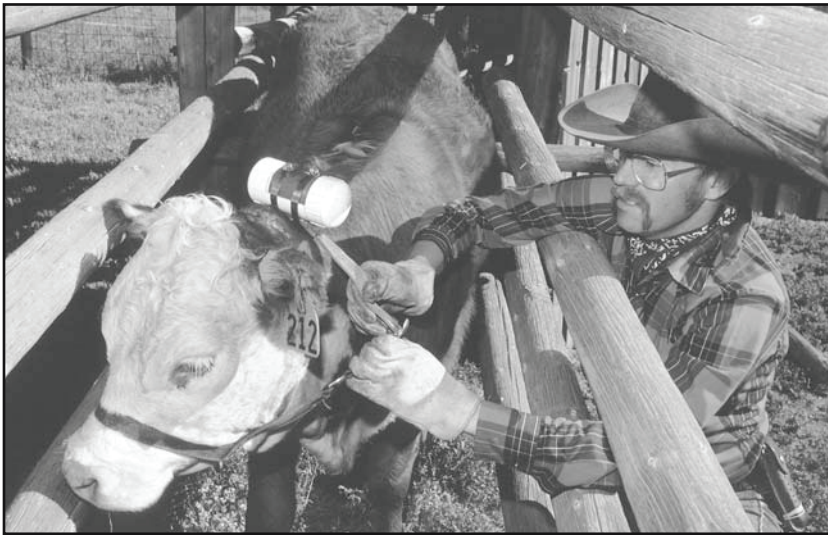
The sensing unit that a technician is attaching to this steer records motion and other physiological data that enable scientists to determine how much time the animal spends grazing each day. (Photo courtesy of the Agricultural Research Service, U.S. Department of Agriculture)
