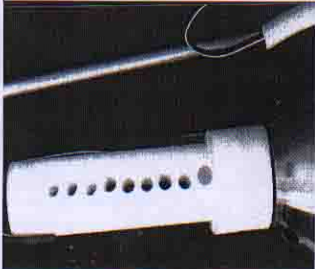
FIG 8. A side view of the central nylon rod showing the adjustment holes that allows a variable gap between the cone stack and the bottom of the vat.
