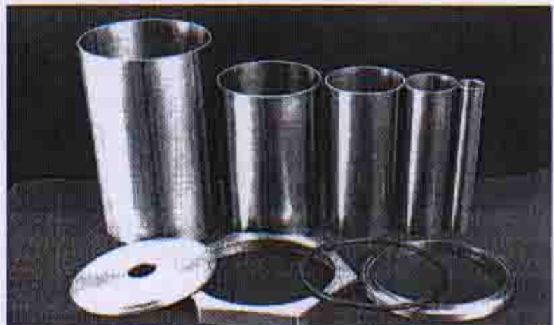
FIG 17. Cell - 5 cylinder. All major components of the cell. Note separate base plate and nut. The thread ring is still to be push fitted to the lower part of the outer cylinder.
