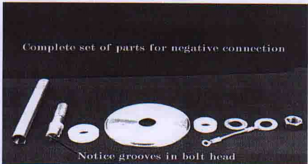
FIG 20. Cell - 5 cylinder. All the components required for the construction of the negative connection to the central 1 inch cylinder.
