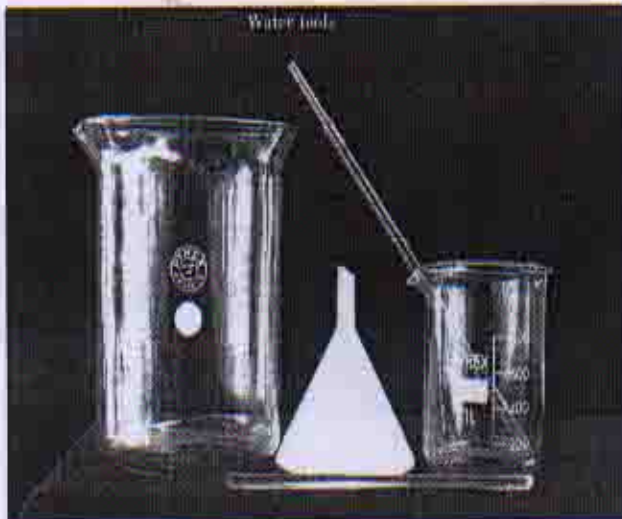
FIG 2. Water Tools - Large Beaker to hold charged water during cell service. Funnel and small beaker for topping up the cell. Burette for adding or removing a small quantity of water from the cell and a glass stirring rod
