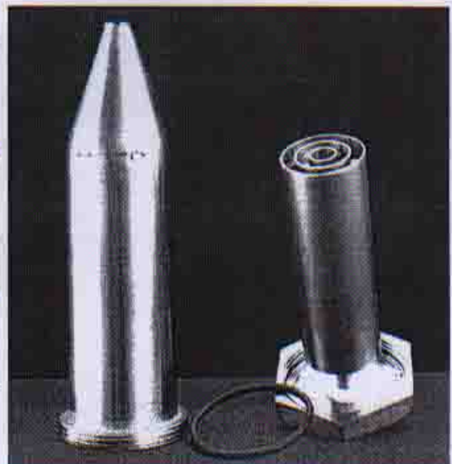
FIG 16. Cell - 4 cylinder. View of the completed cell sub-assemblies. Note that the compression fitting is missing from the top of the cone. The O-ring fits between the outer thread and the base cap.
