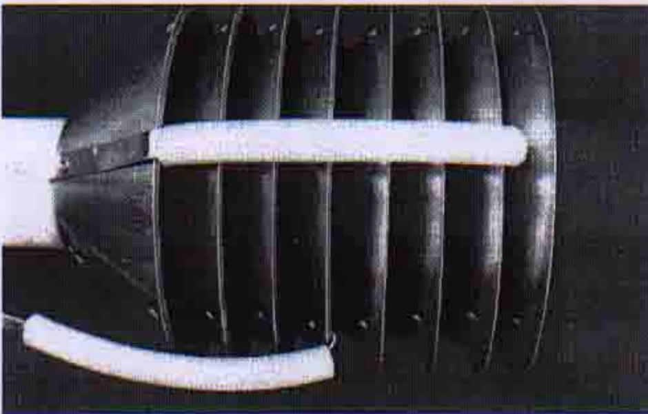
FIG 9. Charging Vat. A side view of the cone stack. Notice the connections, insulation of the straps and connection to the cone.
