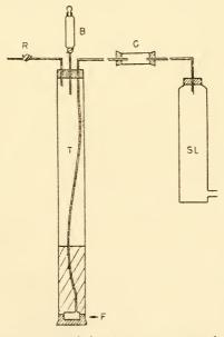
FIG. 27. Apparatus used for the measurement of  $CO_2$  production in mice. For explanation see text.
