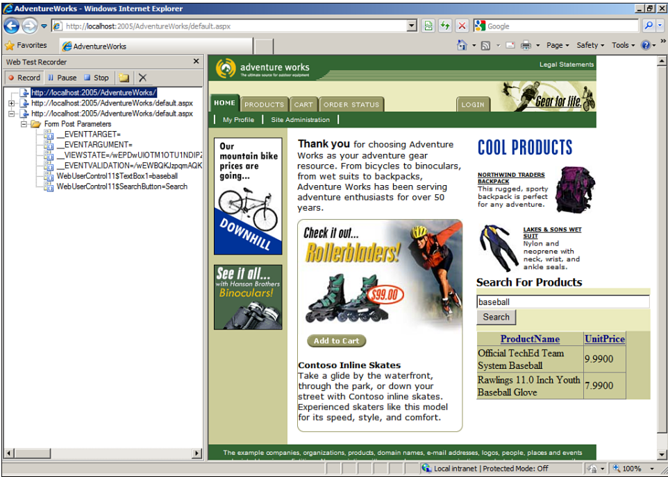
FIGURE 8-14: When you add a Web performance test in VS, you drive the scenario as a user would—but the instrumented Web browser captures the interaction at the HTTP level and produces a parameterized test against the server.
